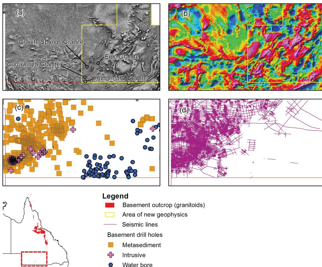
Figure 2: Datasets used in interpretation and compilation of the basement geology map. a) Magnetics (including new data) and distribution of outcropping rocks, b) gravity (including new data), drill holes, d) seismic lines
