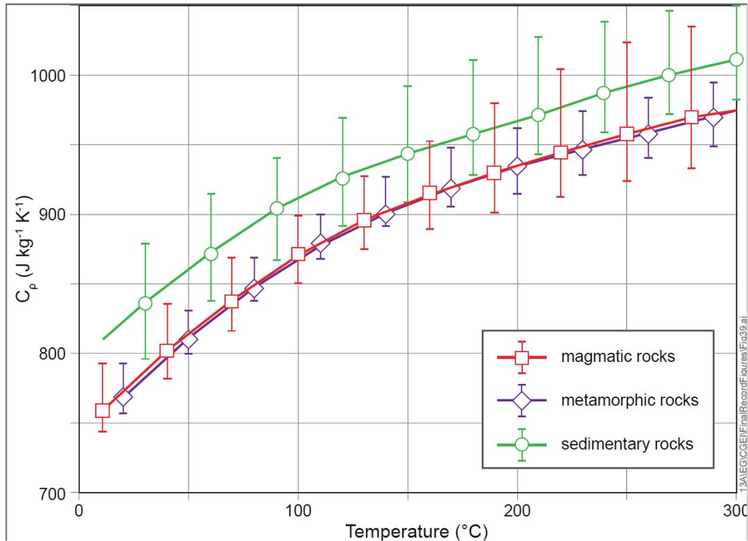
Figure 3: Mean values and ranges of variation of specific heat capacity ( $C_p$ ) at constant pressure as a function of temperature for magmatic, metamorphic and sedimentary rocks (Vosteen & Schellschmidt, 2003).
