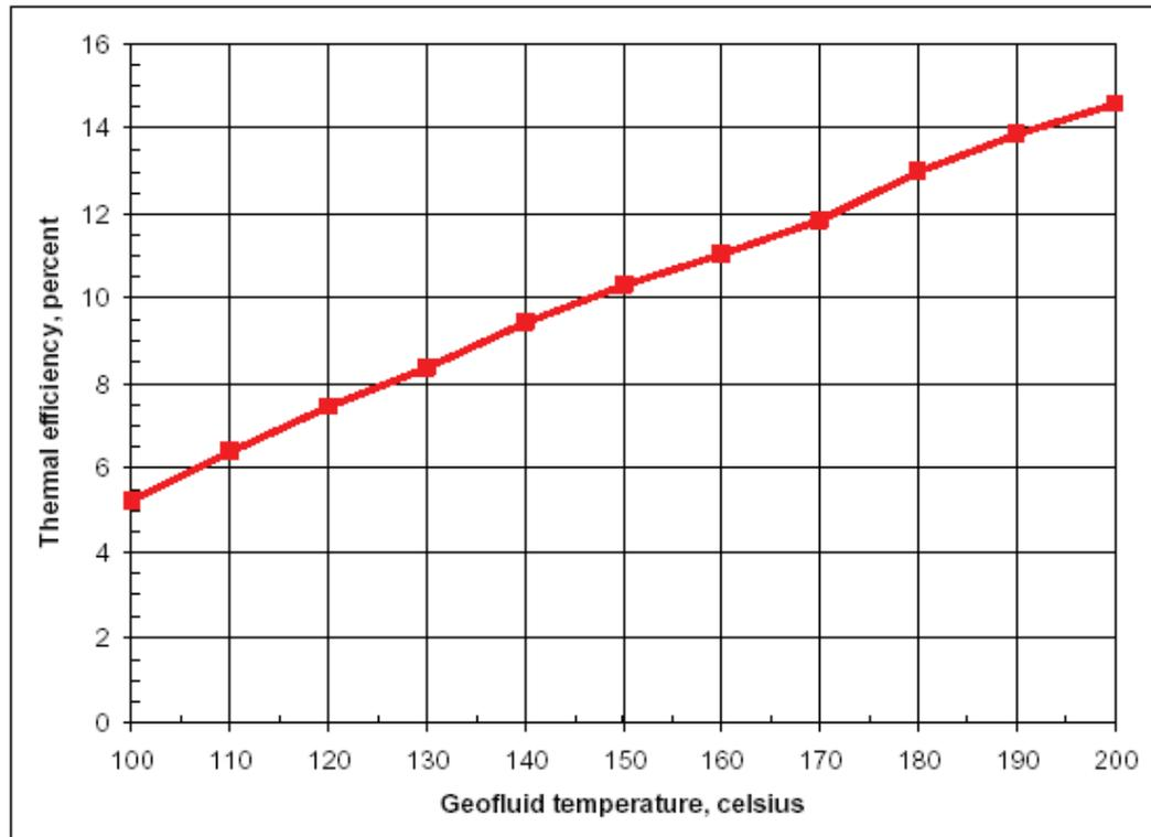
Figure 5: Level of typical thermal efficiencies for electricity generation of ORC binary plants (Bertani, 2010).
