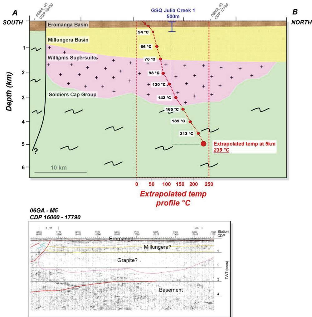
Figure 2: Temperature extrapolation at 5km depth beneath Julia Creek 1, Millungera Basin, based on heat flow of  $113\text{mW/m}^2$ , in conjunction with geological and seismic cross sections.
