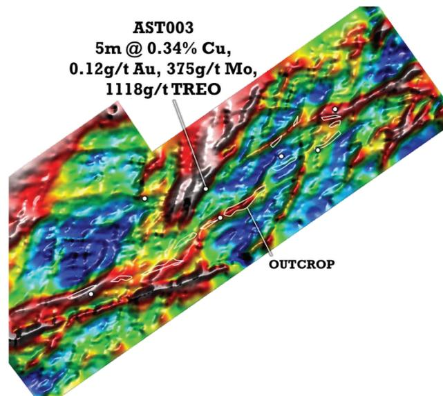
Figure 1. SAM conductivity response over the Mount Agate EPM
