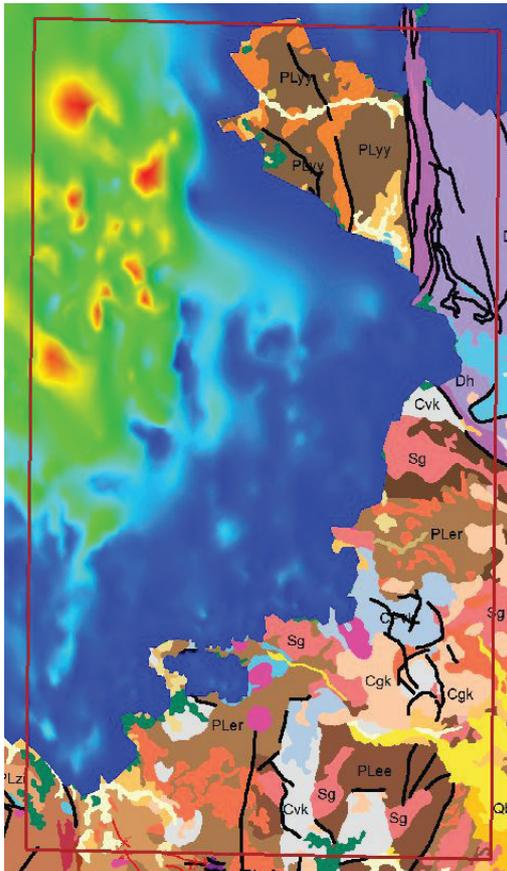
Figure 6: Depth to basement map of Red River Project area overlain on outcropping geology. Blue areas indicate shallow cover and red areas indicate thick cover (1200 metres).
