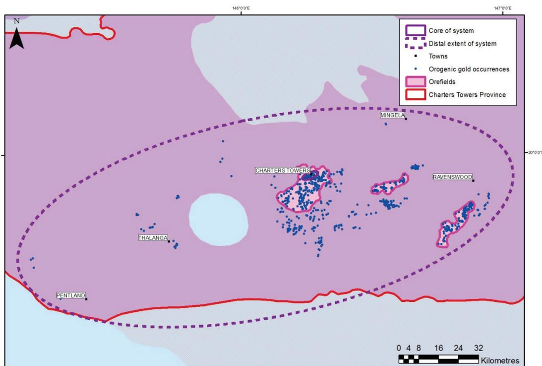
Figure 2: Orogenic gold mineral occurrences within the Charters Towers Province, showing the main three orefields and generalised geology. The purple circles show the core and distal extent of the mineral system.
