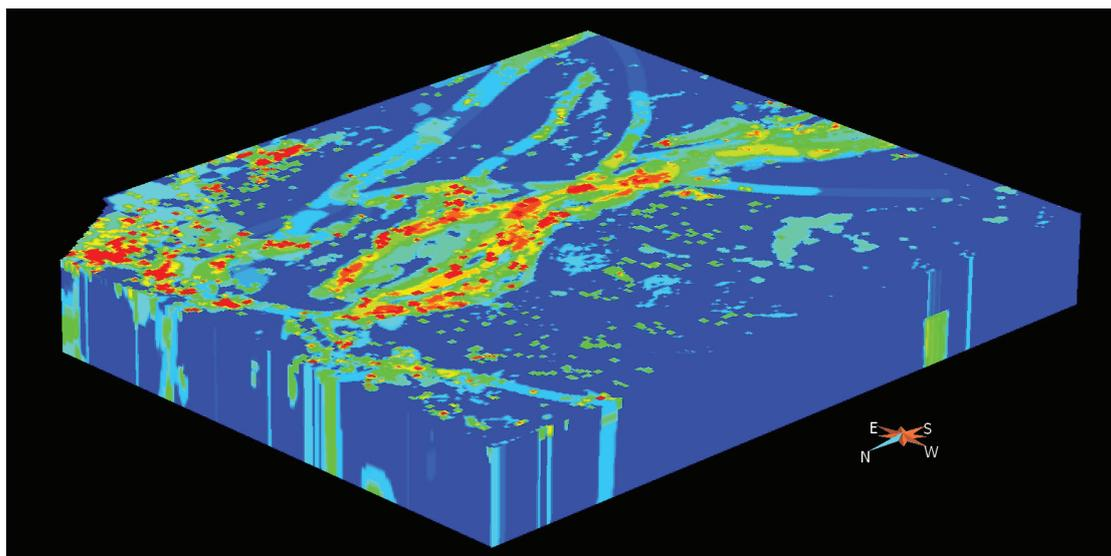
Figure 3: Mineral potential index for the northern section of the Mount Dore region where hot colours represent high mineral potential derived from the Weights of Evidence modelling.
