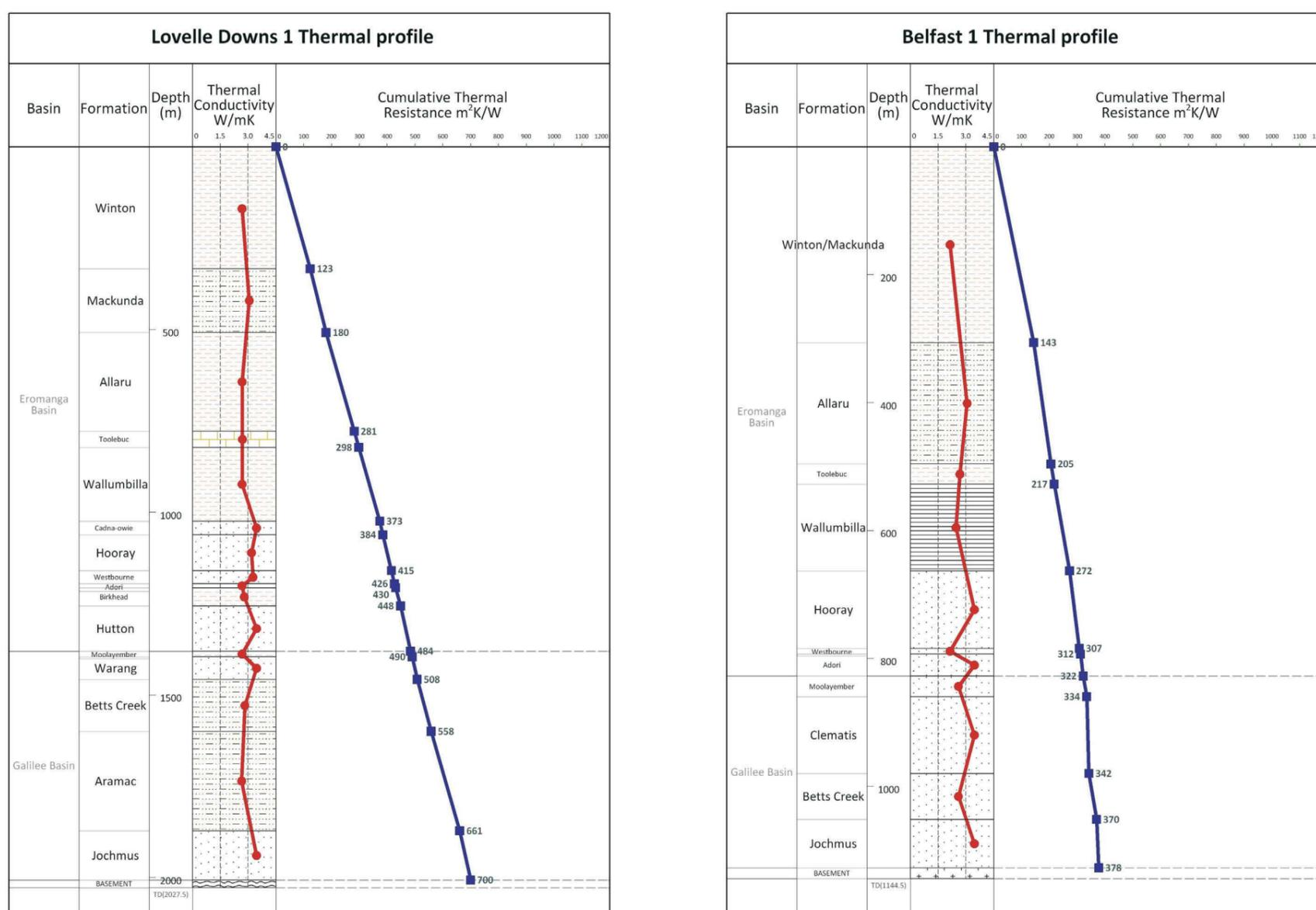
Figure 12.3: Thermal profile of the Galilee Basin estimated from HPP Lovelle Downs 1 and JHR Belfast 1 bulk rock types. Weighted thermal conductivity values calculated from Huston (2010). Refer to Appendix 8 for the raw data.
