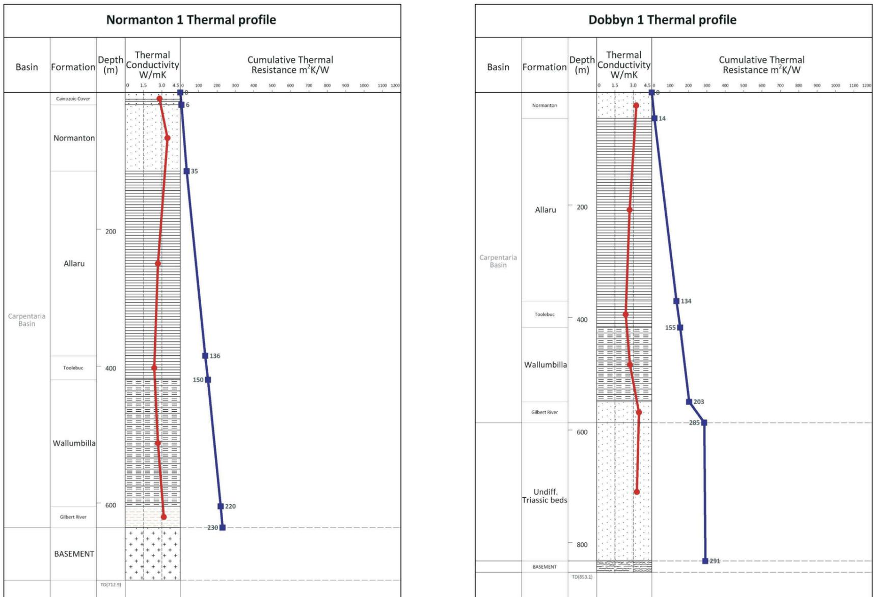
Figure 12.4: Thermal profile of the Carpentaria Basin estimated from GSQ Normanton 1 and GSQ Dobbyn 1 bulk rock types. Weighted thermal conductivity values calculated from Huston (2010). Refer to Appendix 8 for the raw data.
