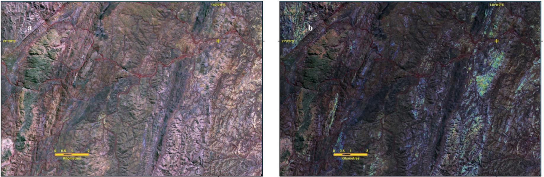
Figure 10.2: a) False colour composite image from Hyperspectral survey shows the Fountain Range Fault crossing the north-west corner of the image, and the Pilgrim Fault (NNE grey zone in the east). b) White mica distribution image for the same area, derived from Hyperspectral data, shows high abundance in red and low in blue; black = not detected. The Wonga Batholith in the west is characterised by high mica abundance.
