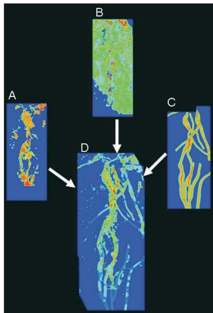
Figure 9.8: Three exploration criteria: Distance to conductive bodies (A), Coincident Magnetic and gravity anomalies (B) and Distance to crustal scale faults (C), and the Mineral Potential Index (D)
