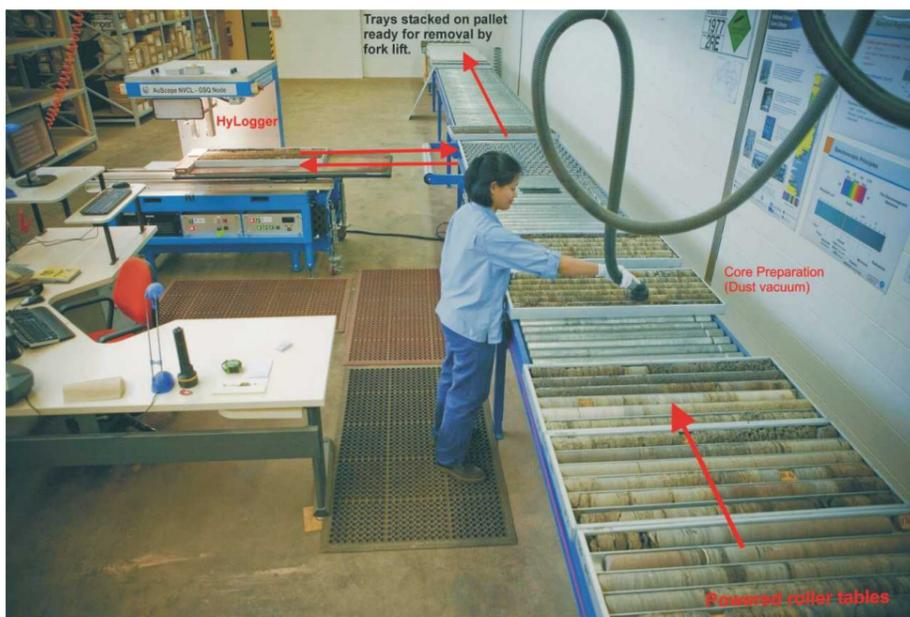
Figure 10.3: Core is cleaned and annotated with depth information before being scanned by HyLogger™ to determine Visible to Short Wavelength Infra-Red spectra. The HyLogger™ is operated by the Geological Survey of Queensland at the Exploration Data Centre, Zillmere, Brisbane.
