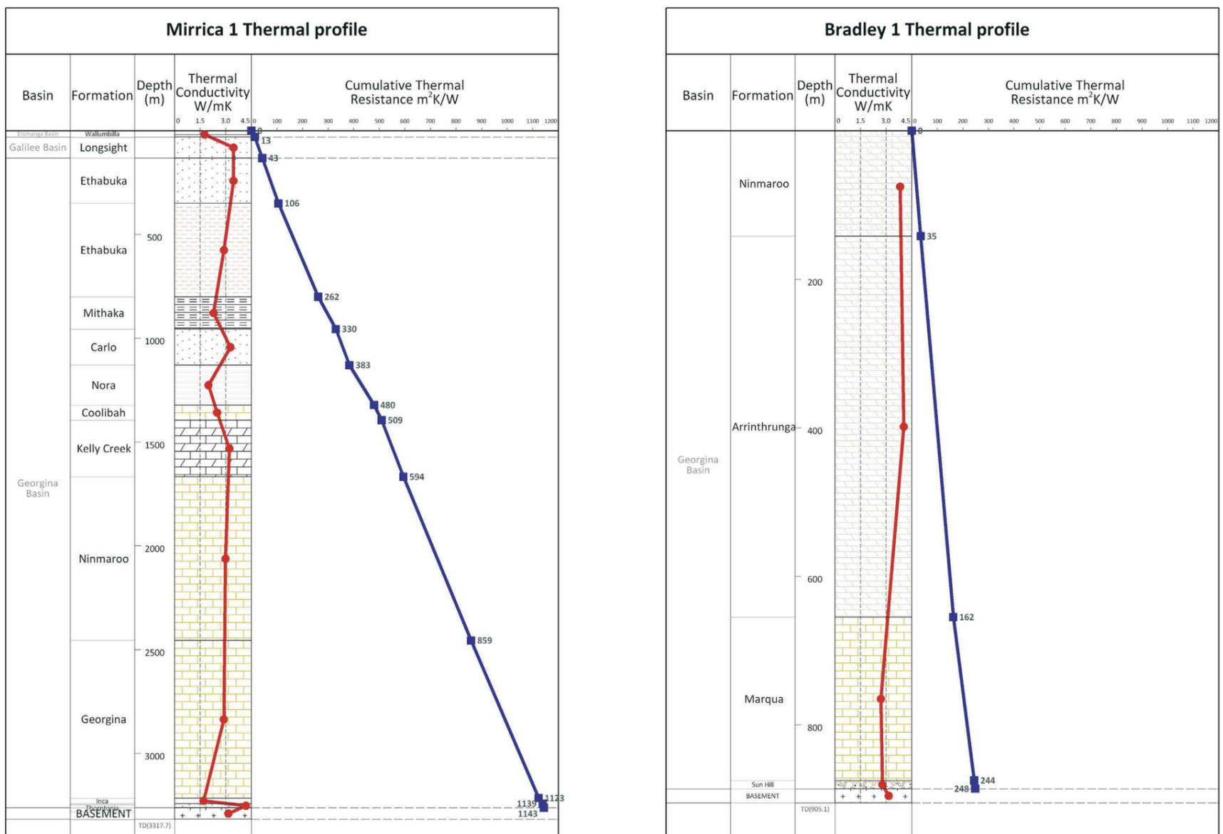
Figure 12.2: Thermal profile of the Georgina Basin estimated from AOD Mirrica 1 and PGA Bradley 1 rock types. Weighted thermal conductivity values were calculated from Huston (2010). Refer to Appendix 8 for the raw data.
