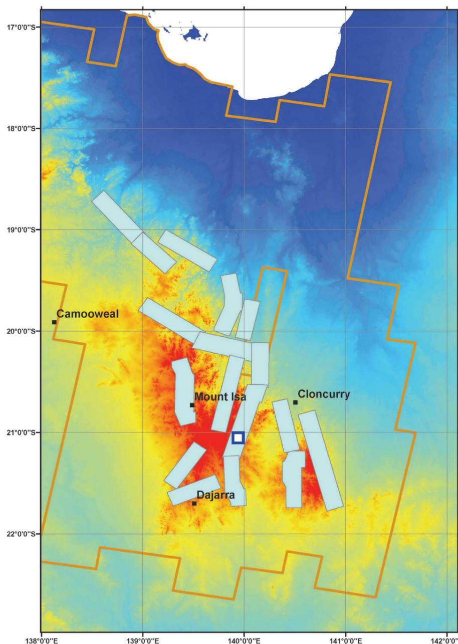
Figure 10.1: The airborne Hyperspectral coverage in the Mount Isa region comprises seventeen 15km-wide swaths within the footprint of an extensive regional ASTER mosaic (large polygon). Blue square shows location of Figure 10.2. Underlying image shows topography (Blue = low; red = high).
