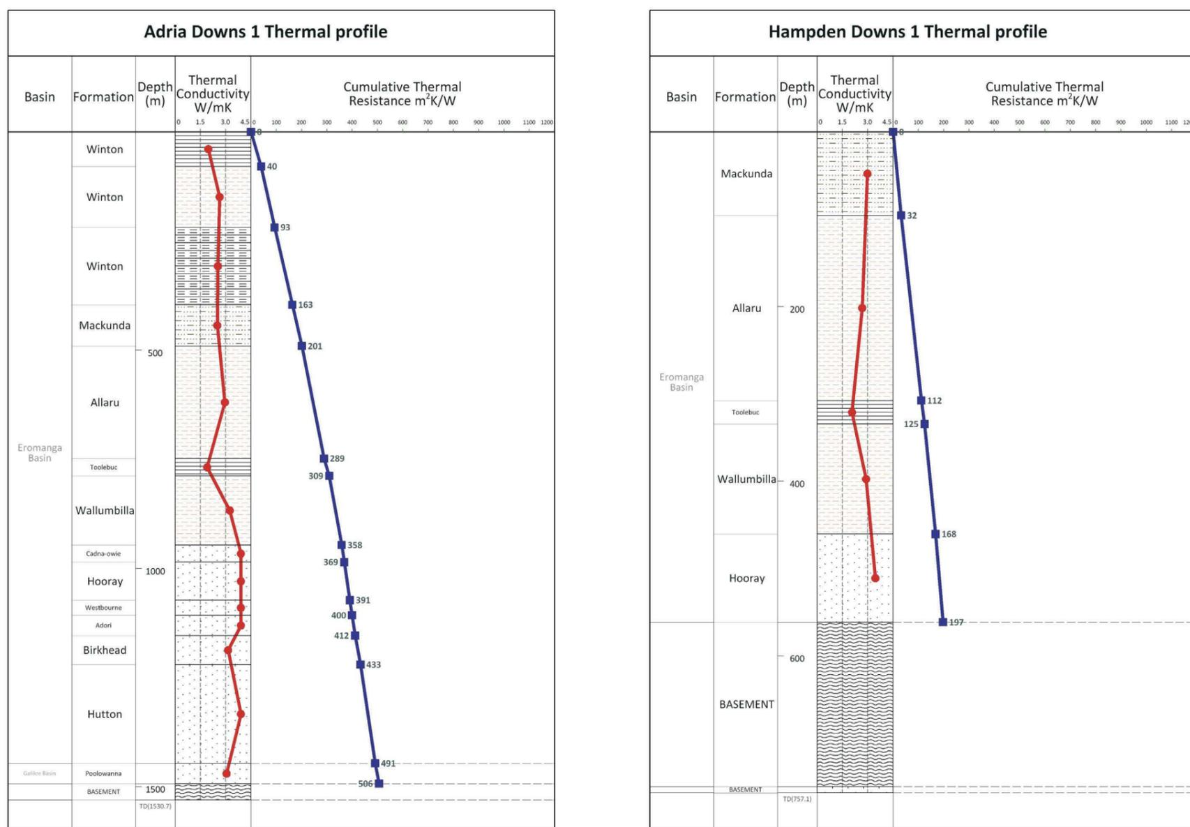
Figure 12.5: Thermal profile of the Eromanga Basin estimated from DIO Adria Downs 1 and JHR Hampden Downs 1 bulk rock types. Weighted thermal conductivity values calculated from Huston (2010). Refer to Appendix 8 for the raw data.
