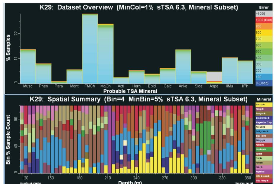
Figure 10.4: Overview display in TSG software shows mineral abundance and downhole distribution (Depth on horizontal axis).
