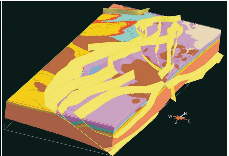
Figure 9.2: Voxel model of the Mount Dore region (900m x 200m) viewed from the south with SKUA faults
