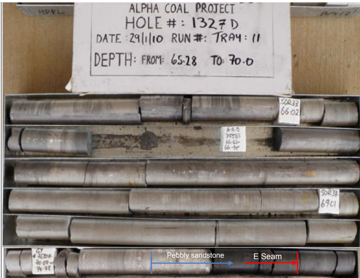
Plate 4-12 E to D interburden showing pebbly sandstone overlying the E seam
