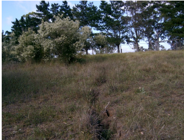
Fig. 5.8 Photographs of Surface Cracking on sides of steep sloping areas in the NSW Southern Coalfield with greater than 400 metres cover
