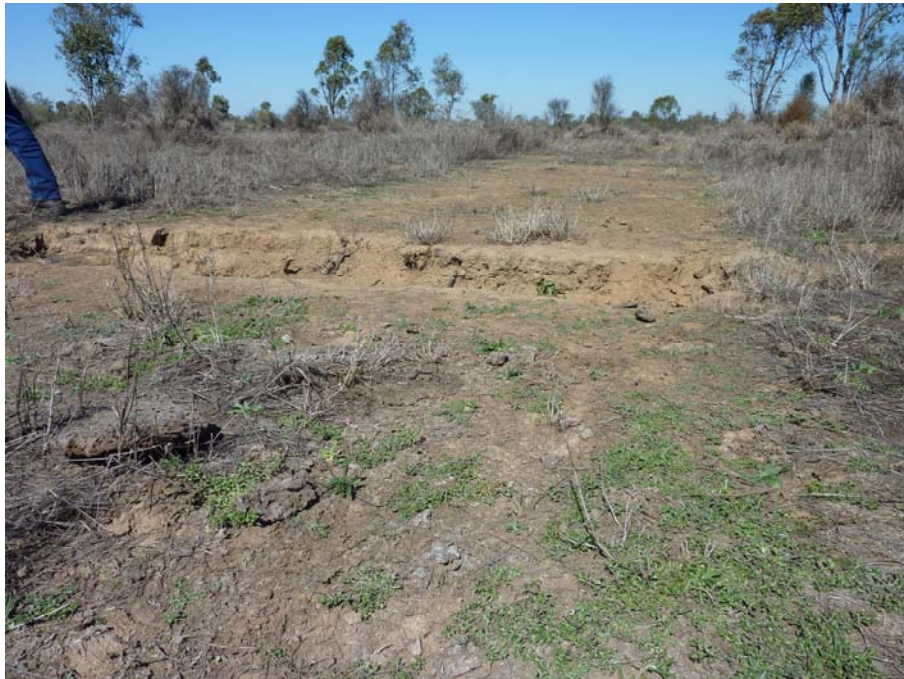
Fig. 5.3 Step in ground across longwall centreline at approx. 180 m cover
