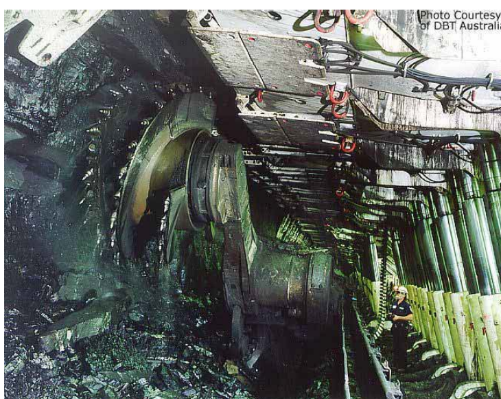
Fig. 3.1 Cross-section along the Length of a Typical Longwall at the Coal Face and a photograph of a typical Shearer, Conveyor and Hydraulic Support Chocks
