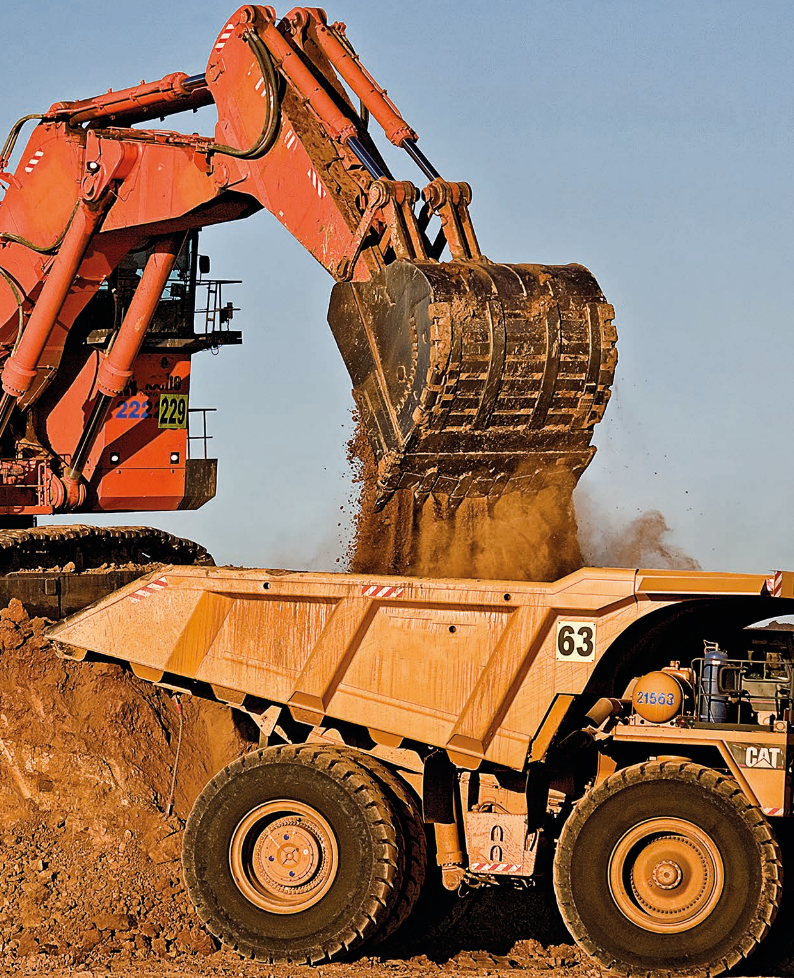
Overburden removal by truck and excavator
