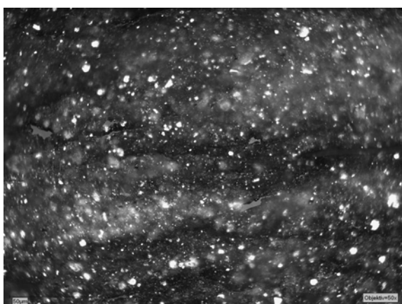
E2616E Fluorescing lamalginite in silty claystone, reflected white light, X50
