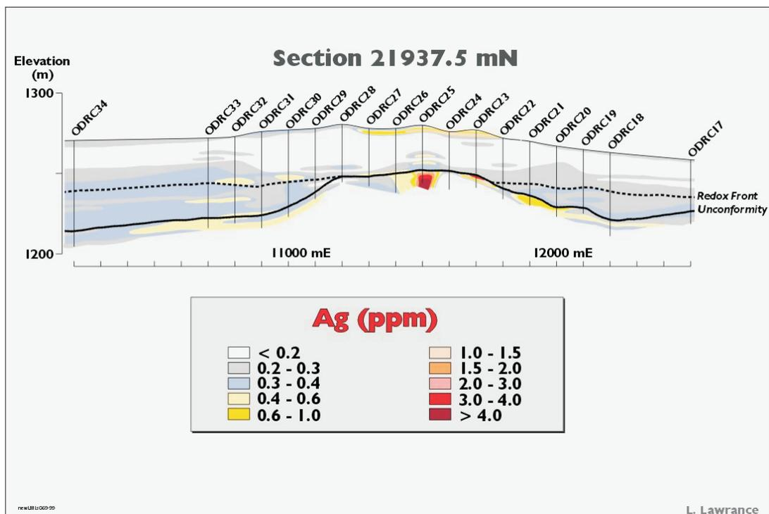
Figure 4.18 Distribution of Ag within Mesozoic cover on Section 21 937.5 mN over the buried Osborne Cu-Au deposit, Northern Queensland, Australia (after Lawrance, 1999)
