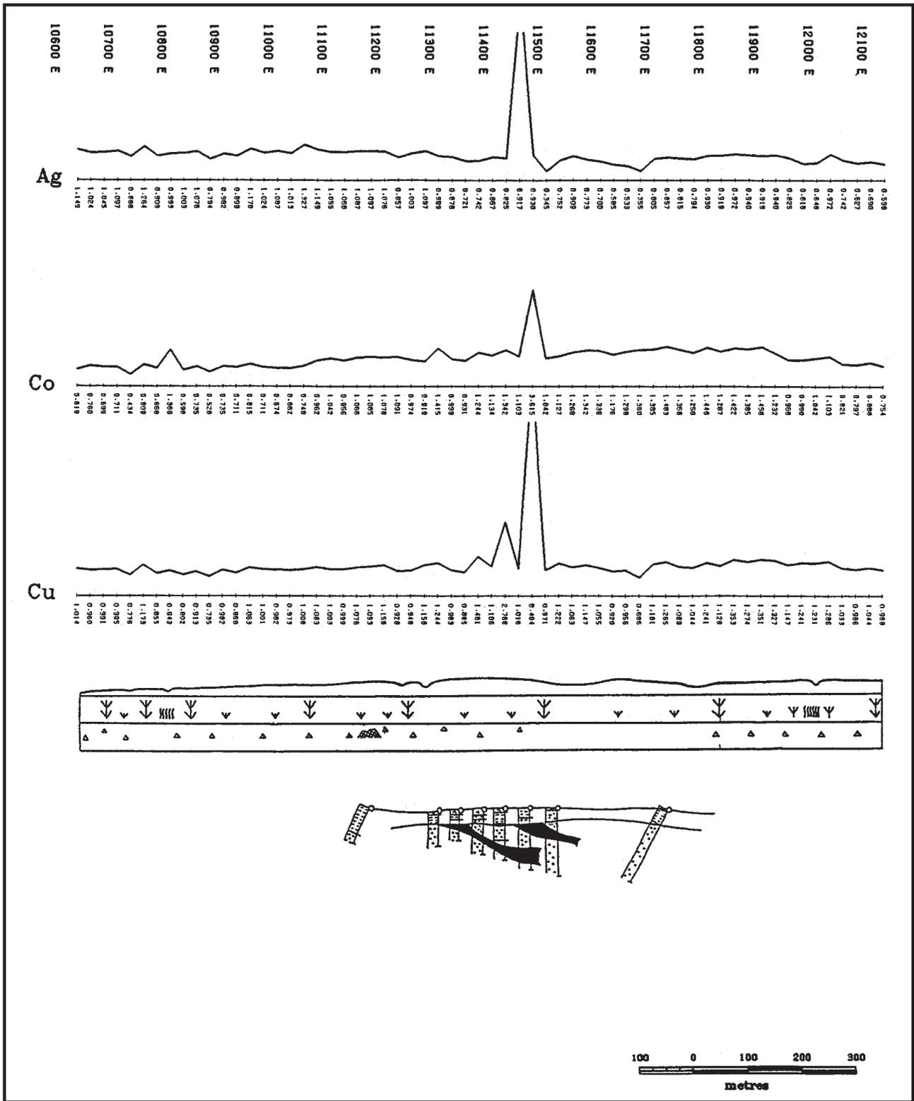
Figure 4.11 TMGM Cu, Co and Ag results on Line 21 937 mN at Osborne (after Ryss et al, 1992)
