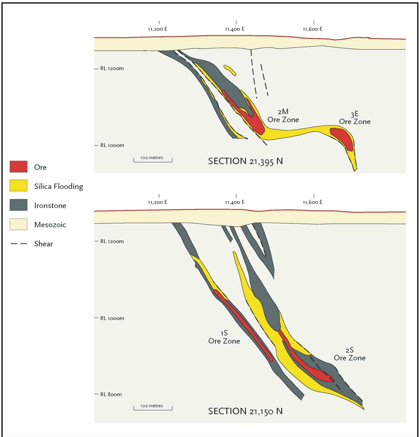
**Figure 4.32 Osborne cross sections at 21 395 mN and 21 150 mN showing zones of silica-flooded rock** (after fb\_osborne.pdf, at the Placer Dome internet site, 2001)
