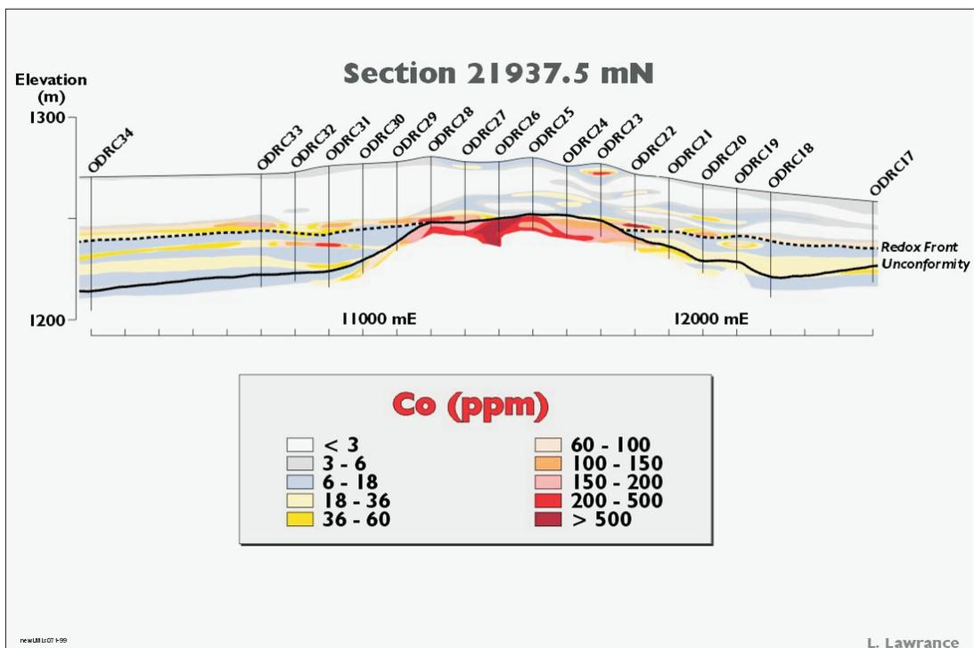
Figure 4.20 Distribution of Co within Mesozoic cover on Section 21 937.5 mN over the buried Osborne Cu-Au deposit, Northern Queensland, Australia (after Lawrance, 1999)
