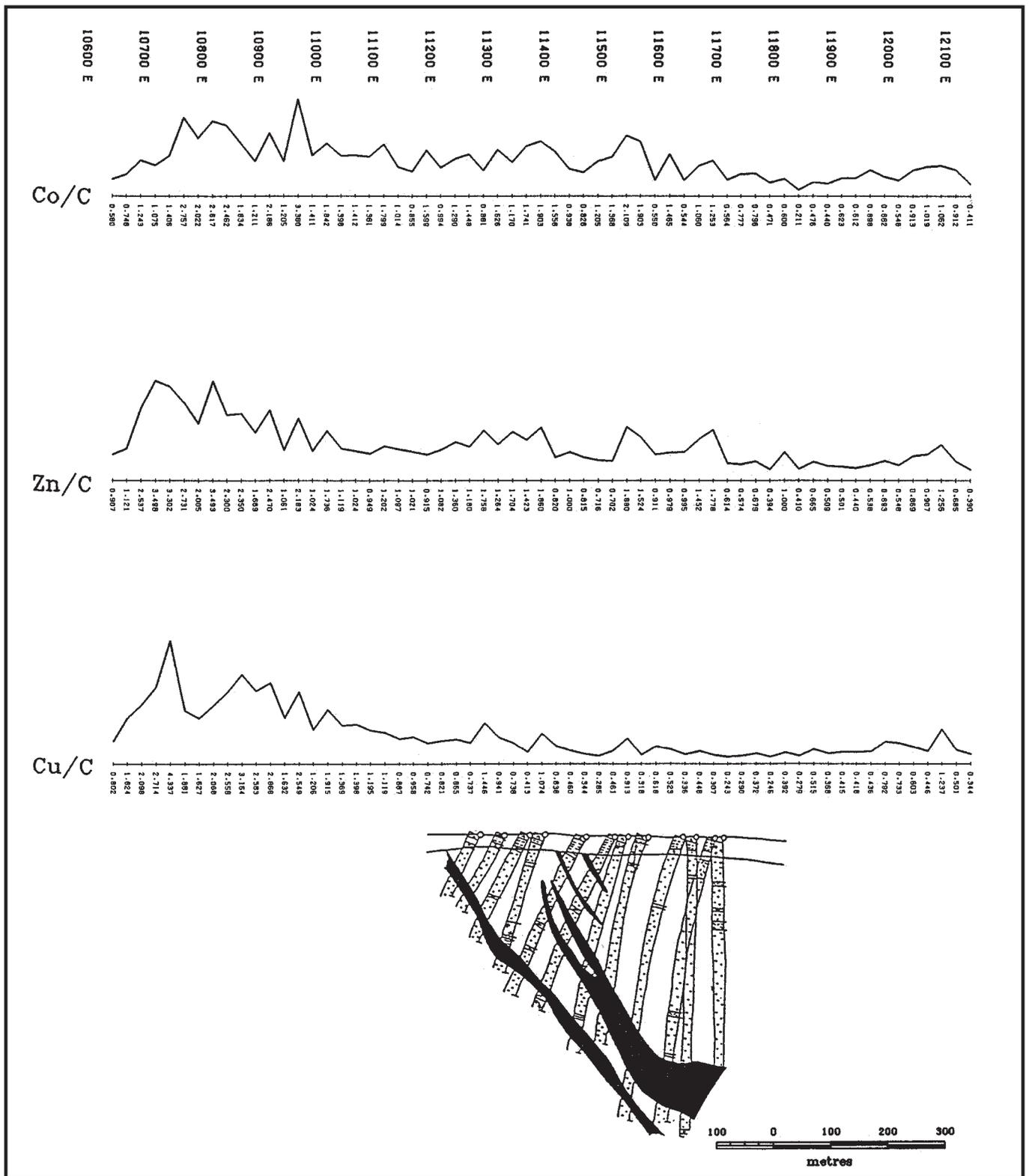
Figure 4.9 MPF geochemical profiles on Line 21 140 mN (after Ryss et al, 1992)
