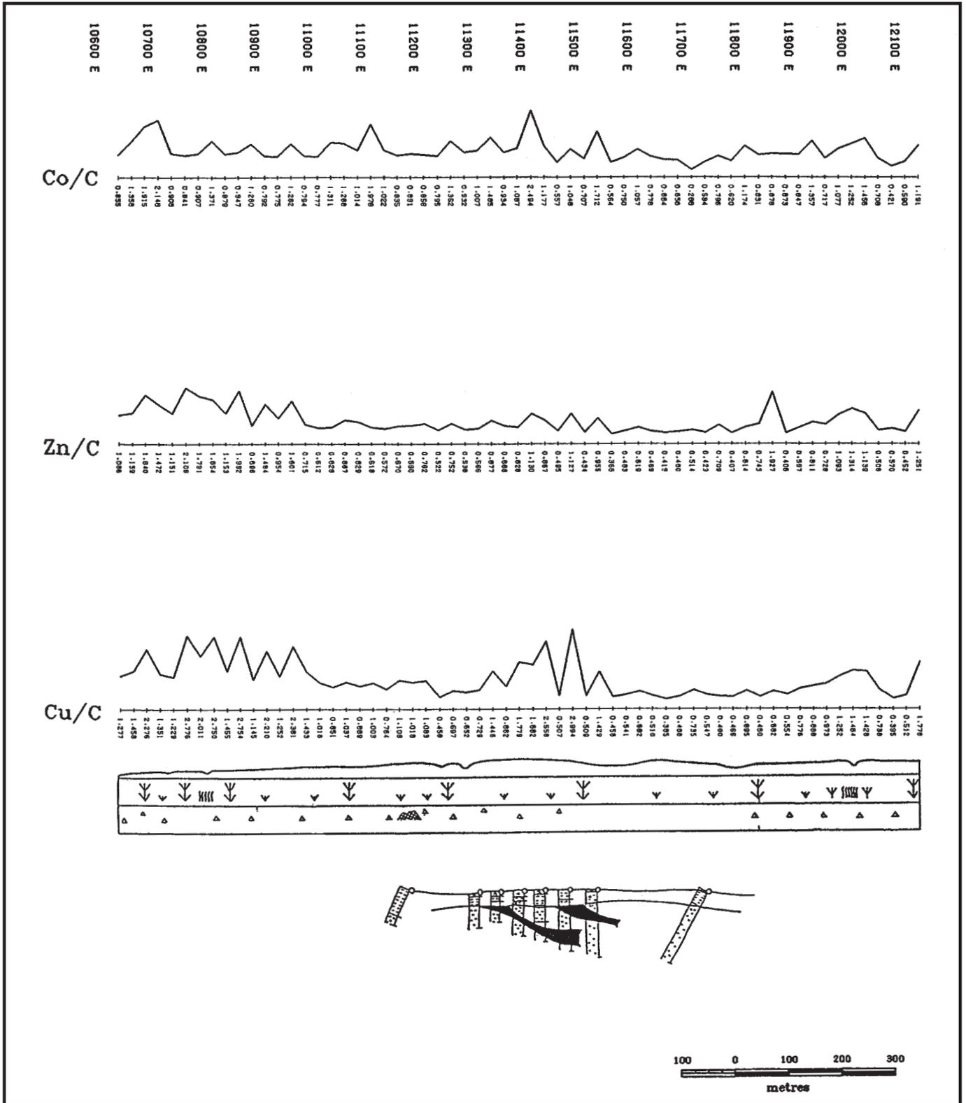
Figure 4.8 MPF geochemical profiles on Line 21 937 mN (after Ryss et al, 1992)
