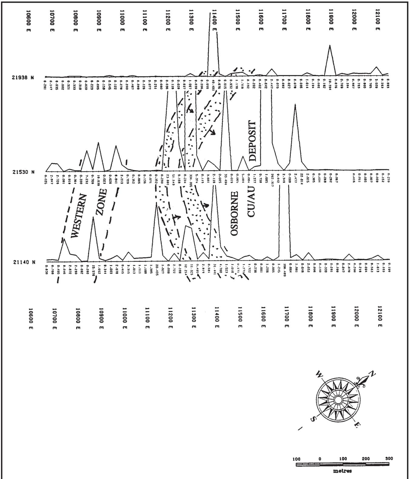
Figure 4.14 CHIM Cu x Zn x Co in plan at Osborne (after Ryss et al, 1992)
