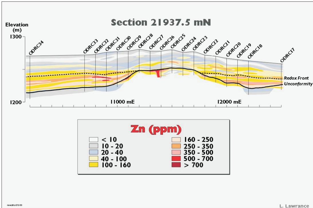
Figure 4.19 Distribution of Zn within Mesozoic cover on Section 21 937.5 mN over the buried Osborne Cu-Au deposit, Northern Queensland, Australia (after Lawrance, 1999)
