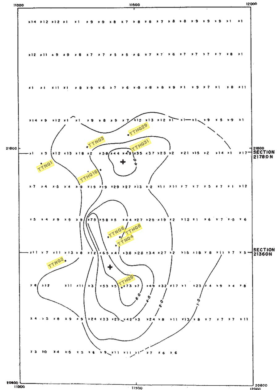
Figure 4.29 Contours for "late-time" moving loop TEM response - Sirotem channel 14 (delay time 11.6 ms) at Osborne (after Anderson and Logan, 1992)
