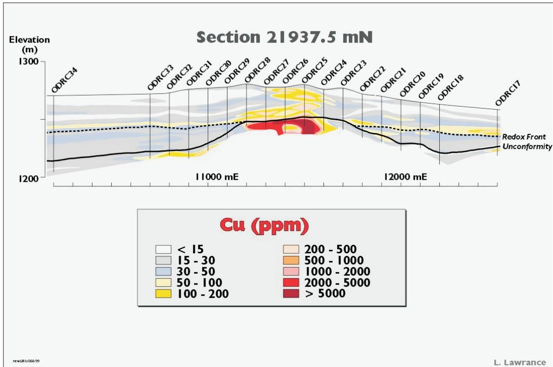
**Figure 4.15** Distribution of Cu within Mesozoic cover on Section 21 937.5 mN over the buried Osborne Cu-Au deposit, Northern Queensland, Australia (after Lawrance, 1999)
