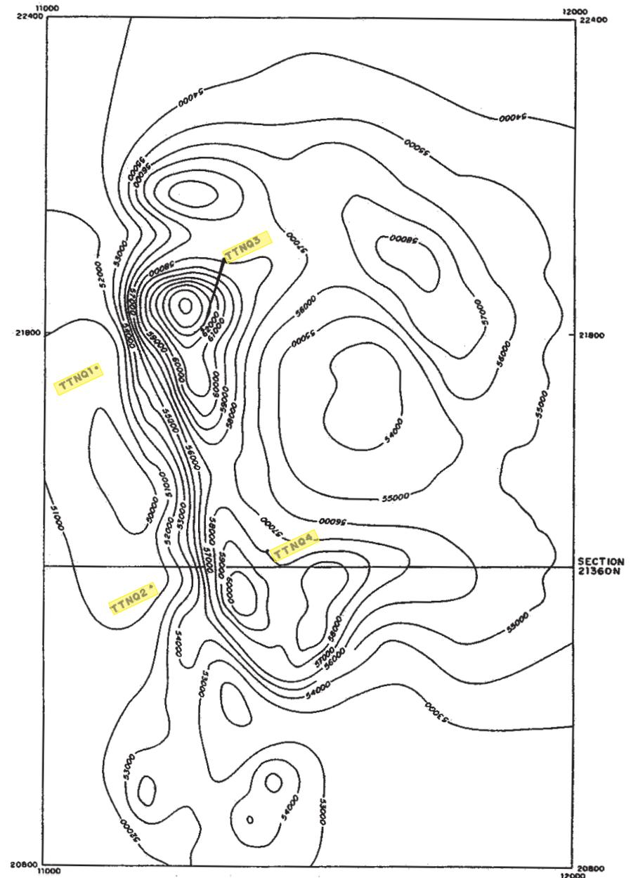
Figure 4.27 Total magnetic intensity for ground magnetic data at Osborne, with early drill holes indicated (after Anderson and Logan, 1992)
