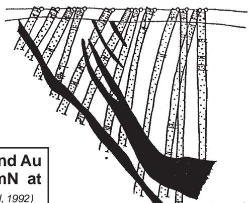
**Figure 4.13** CHIM Cu, Zn, Co and Au on Line 21 140 mN at Osborne (after Ryss et al, 1992)
