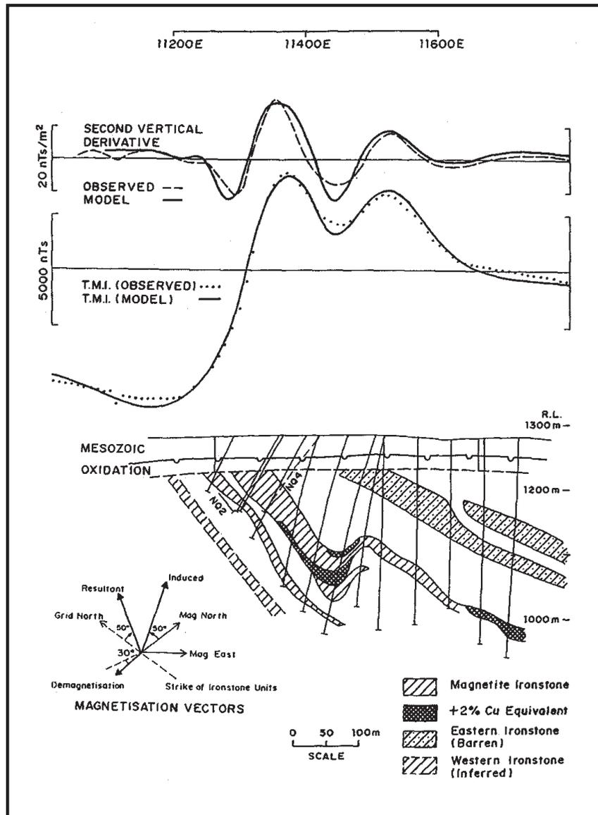
Figure 4.28 Ground magnetic data on section 21 315 mN showing model results, and TMI relative to the geology (after Anderson and Logan, 1992)
