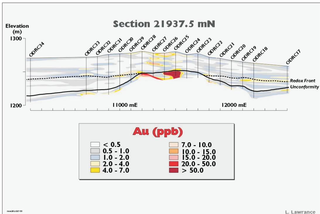
**Figure 4.16** Distribution of Au within Mesozoic cover on Section 21 937.5 mN over the buried Osborne Cu-Au deposit, Northern Queensland, Australia (after Lawrance, 1999)
