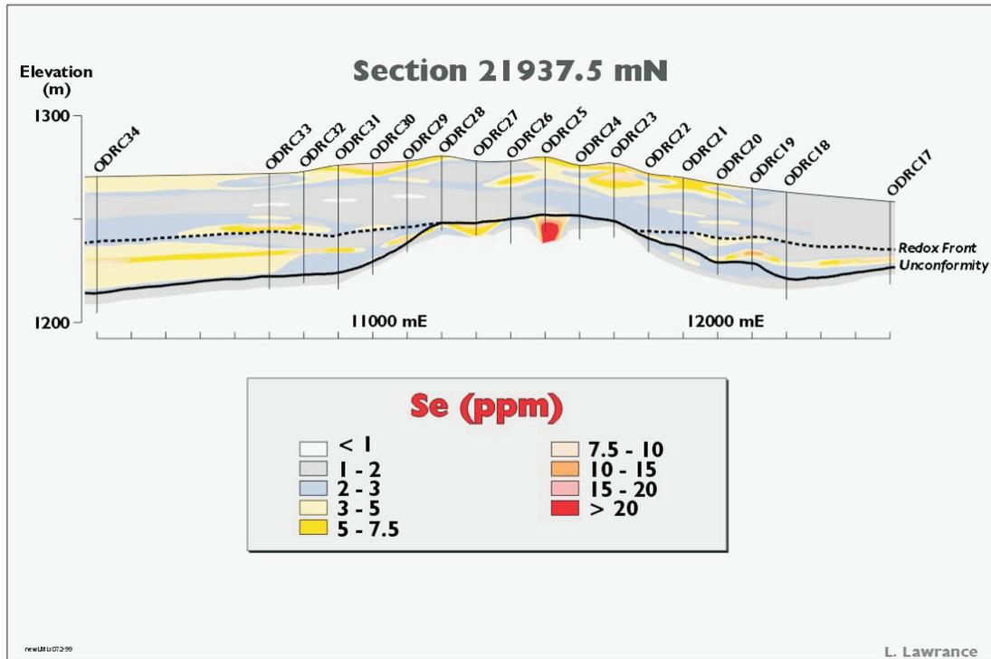
**Figure 4.21** Distribution of Se within Mesozoic cover on Section 21 937.5 mN over the buried Osbornite Cu-Au deposit, Northern Queensland, Australia (after Lawrance, 1999)
