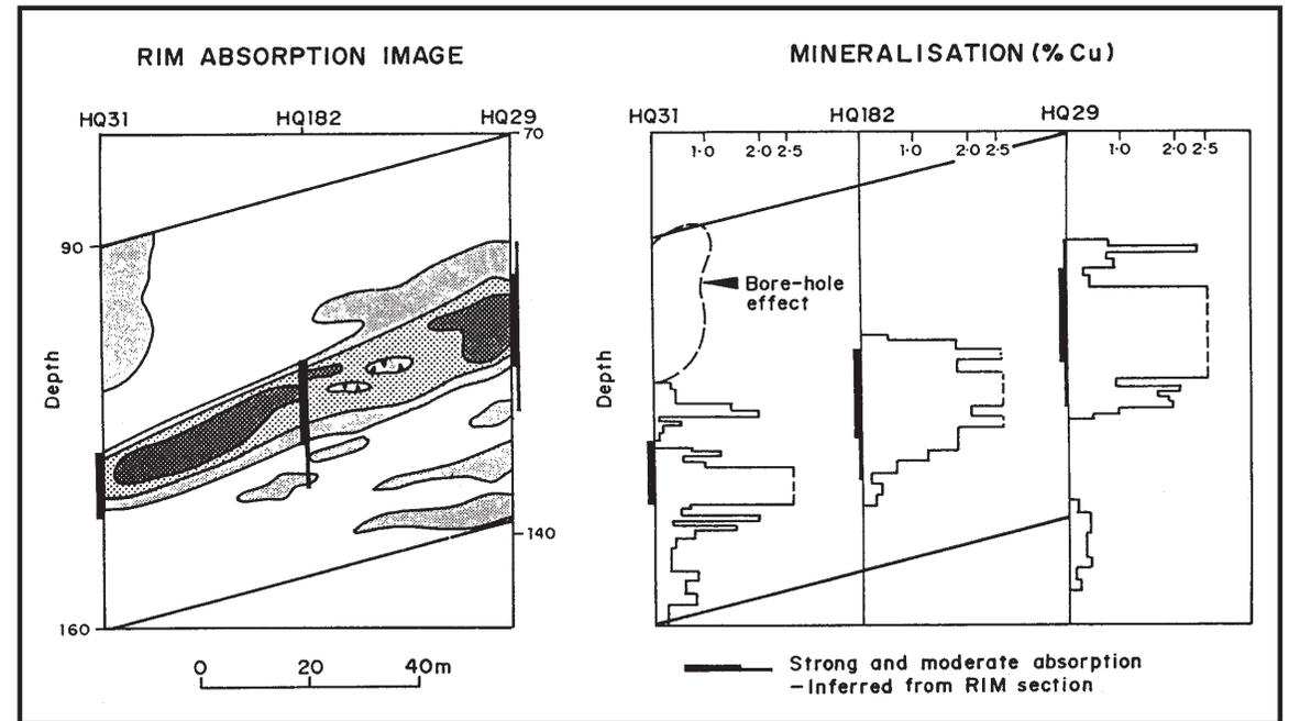
**Figure 4.31** RIM absorption image compared to drill assays in three holes at Osborne (after Anderson and Logan, 1992)
