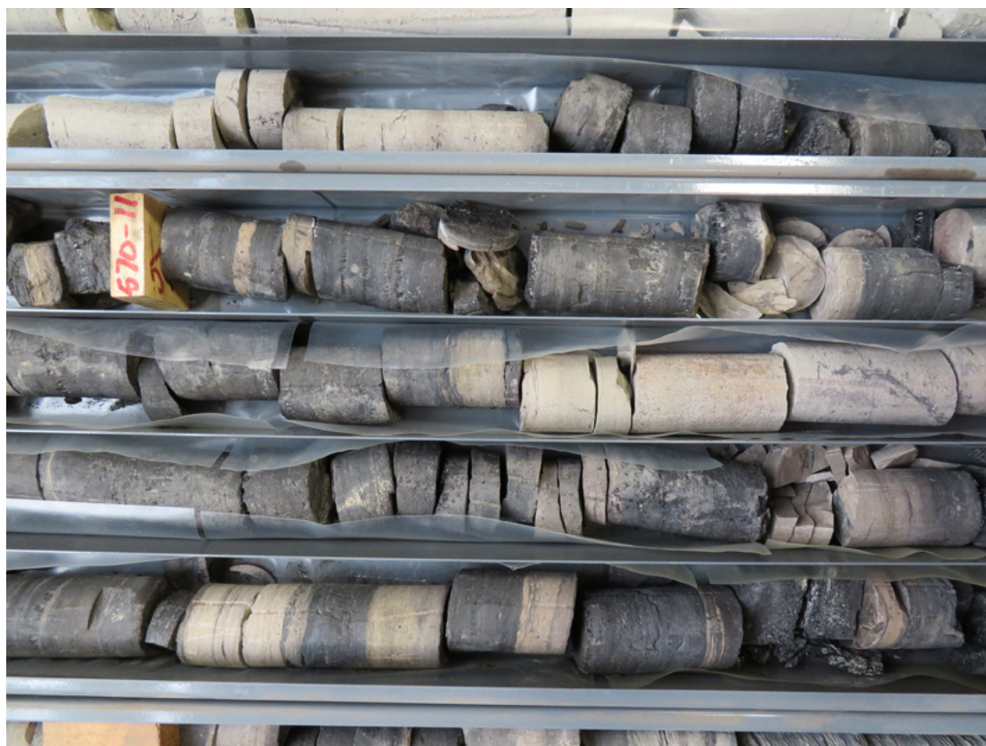
Plate 5. Banded coal with thick intervals of tuffaceous siltstones and carbonaceous mudstones, Grosvenor 3 (depth ~174 m).
