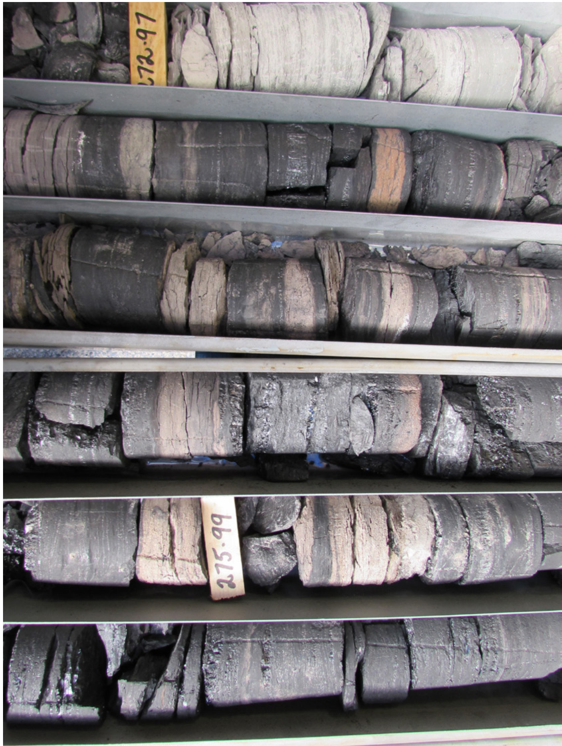
Plate 13. Typically dull coal, thinly interbedded with Fe-rich or tuffaceous mudstones, Cairns County 583.
