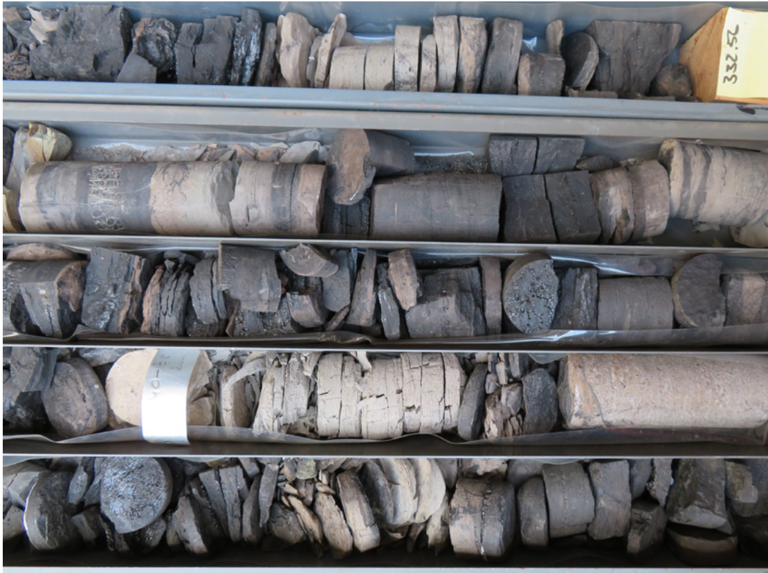
Plate 9. Banded coal and tuffaceous siltstones/mudstones in Grosvenor 12.
