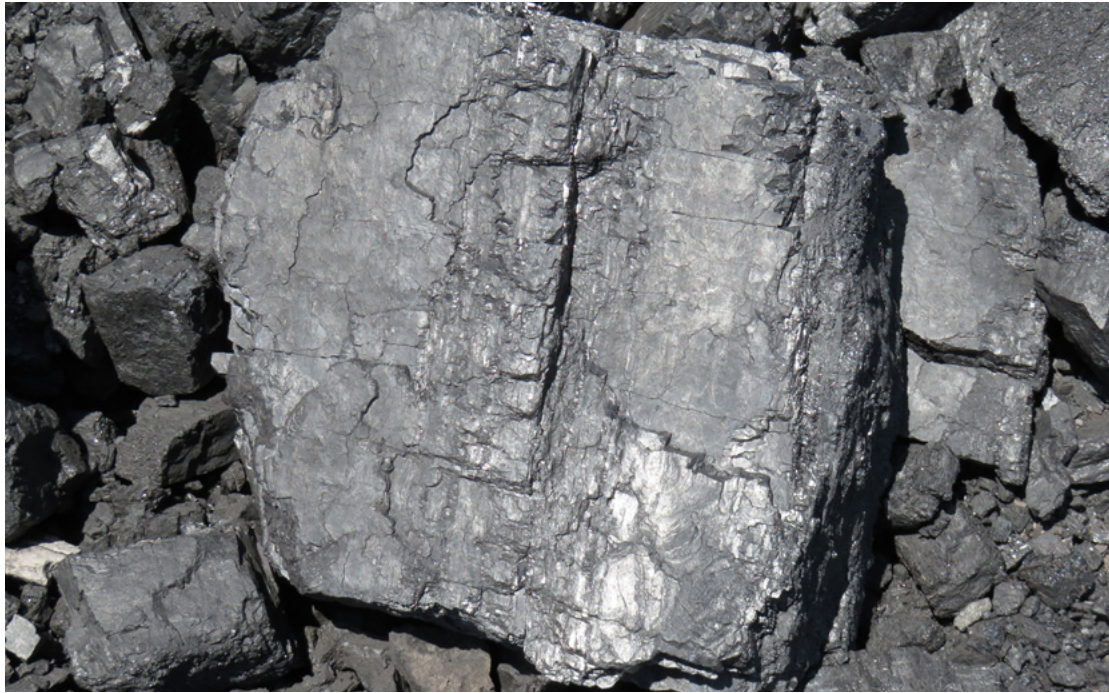
Plate 16. Mineable ply, Fort Cooper Coal Measures (sample size 10 x 10 cm), Hail Creek Syncline.
