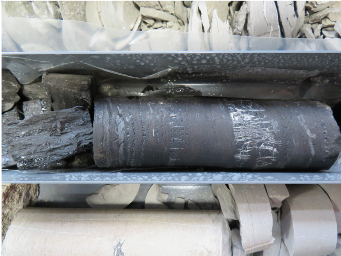
Plate 6. Calcite precipitation in cleats of bright coal bands, Grosvenor 3.
