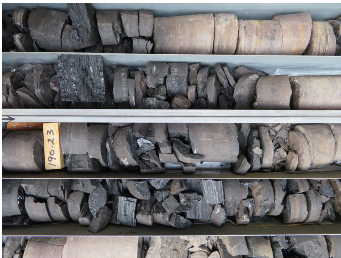
Plate 22. Relatively bright-banded high vitrinite reflectance coal in Talbot 854 (see Figure 62 for vitrinite reflectance profile and Figure 60 for borehole location proximal to a fault).
