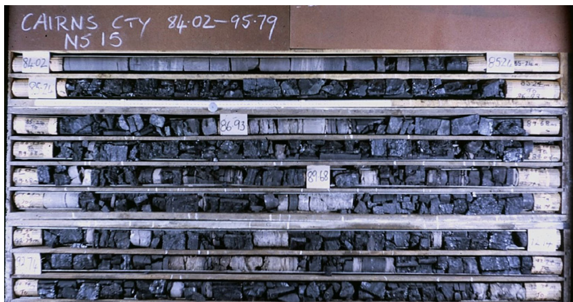
Plate 20. Coal thickness (11.20m) in Cairns County 15 at Winchester.
