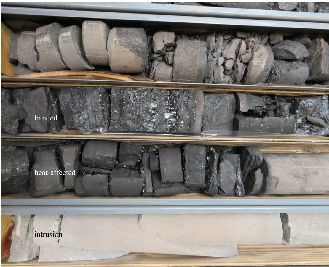
Plate 2. Heat-affected and banded coal proximal to intrusion in Wodehouse 1 (depth ~ 60–65 m).
