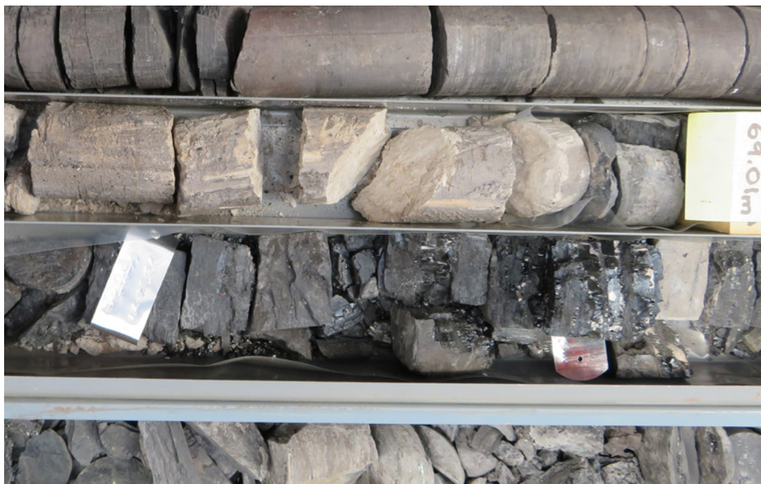
Plate 7. Yarrabee Tuff overlying the Vermont-Girrah Seam, Grosvenor 12.
