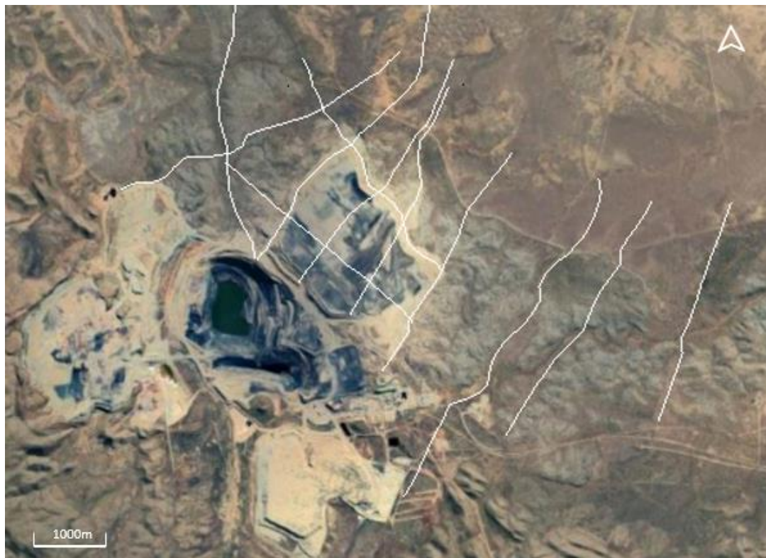
Figure 11. Induced Polarisation (IP) line locations - 2018 Geophysical Survey.
