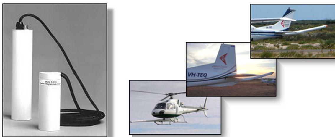
**Figure 6** G822A Magnetometer and Typical Stinger Mounts
