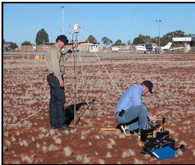
**Figure 12** Setting up base station magnetometer
