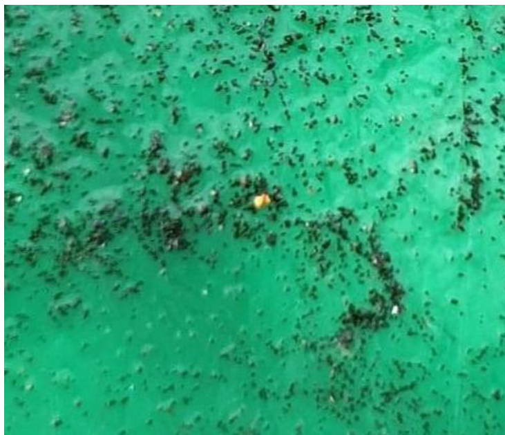
Figure 52: Approximate 0.5mm gold grain panned from soils at the 19.26g/t Au soil site.
