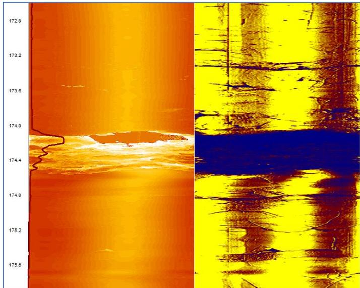
Figure 26: Travel time (left) and amplitude (right) images of a major structure, with caliper trace.
