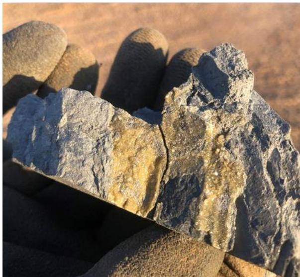
Figure 21: Spalerite vein in laminated micaceous phyllite
