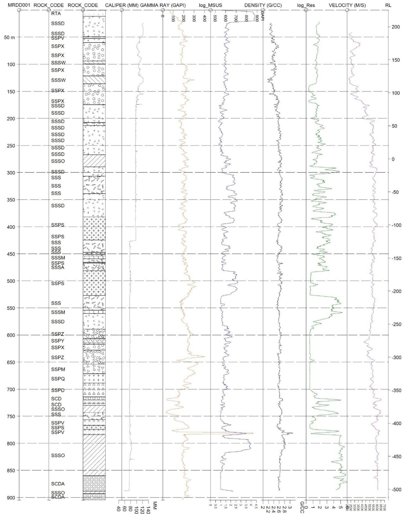
Figure 24: Composite strip log of MRDD001 wireline geophysics results.
