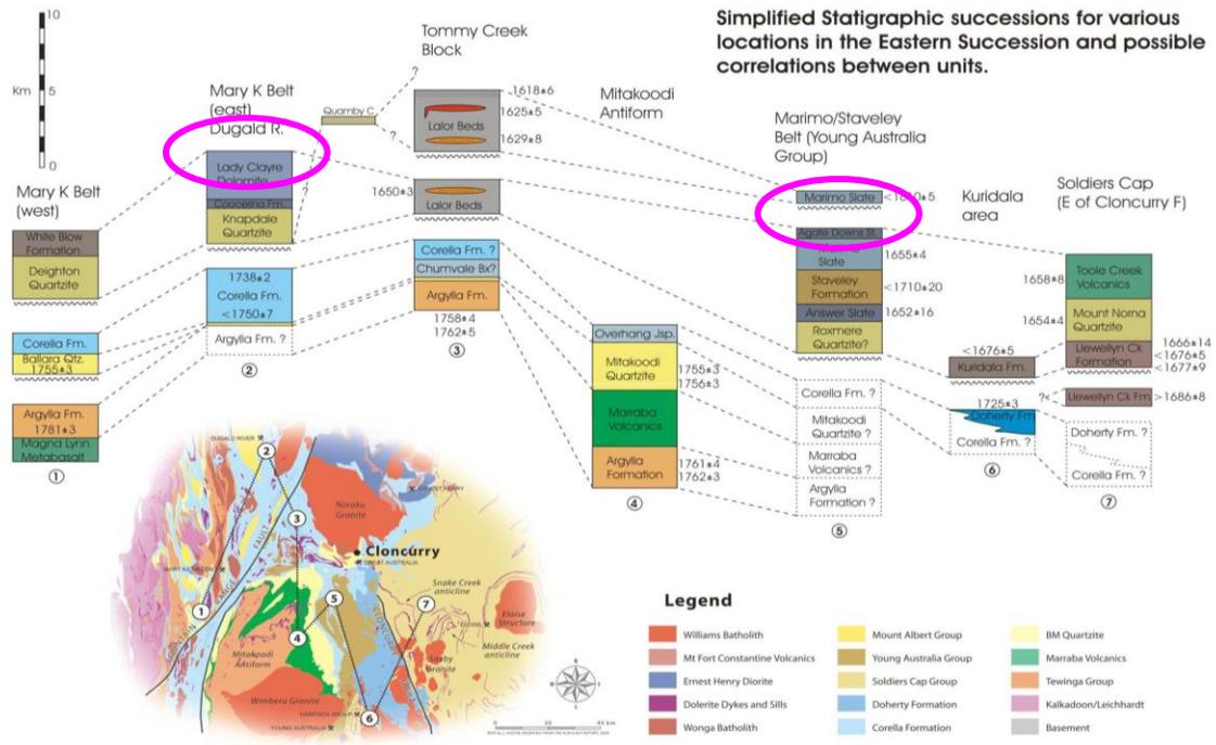
Figure 5: Suggested correlations between simplified stratigraphic columns in the Eastern Succession: from Blenkinsop (2005).
