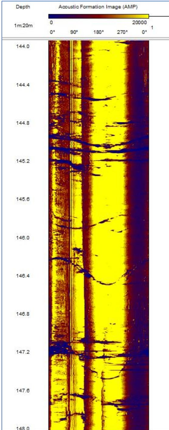
Figure 25: Example of acoustic imager interval from MRDD001, showing several different sinusoidal (planar) features oriented at various angles to the borehole.
