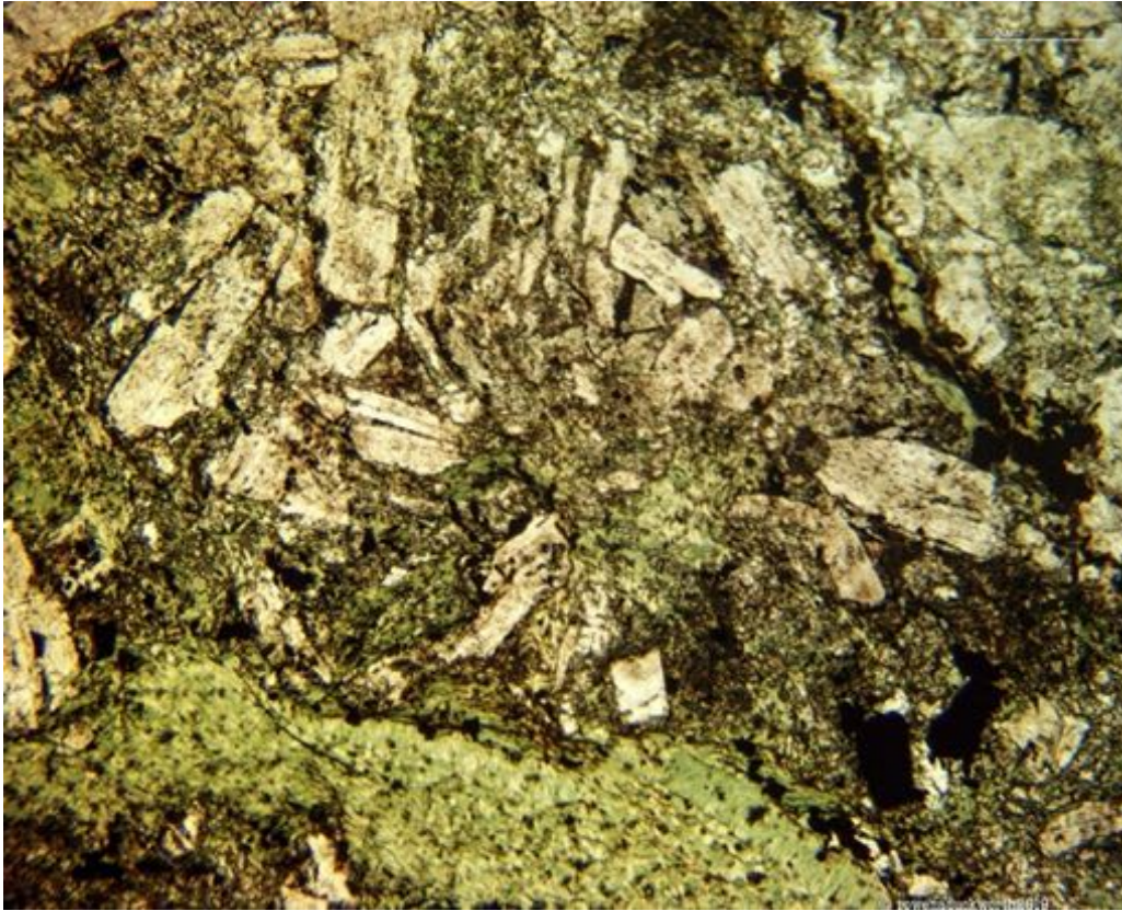
Plane polarised light photomicrograph of sample 162972 (x4) illustrating the texture with feldspar laths and green chlorite and brown carbonate alteration.
