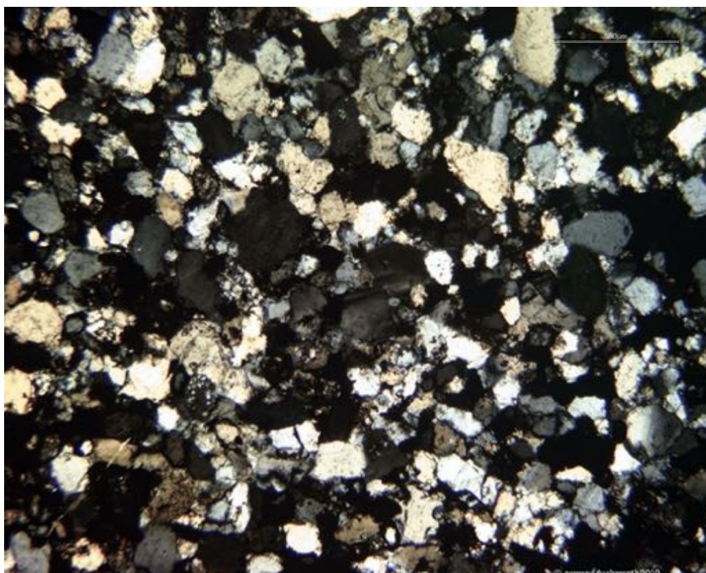
Cross polarised light photomicrograph of sample 163101 (x4) illustrating the texture with anhedronal quartz grains and opaques.
