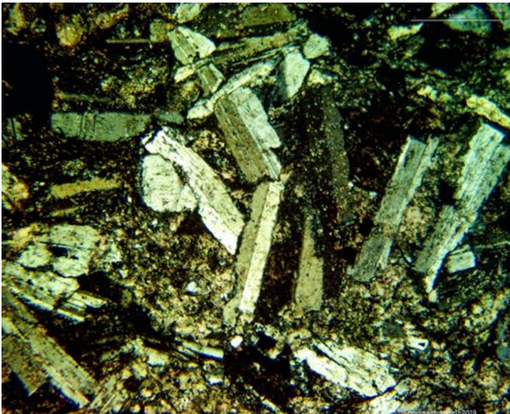
Cross polarised light photomicrograph of sample 162972 (x4) showing the plagioclase-phyric texture of the sample in chlorite-carbonate altered groundmass. Note incipient carbonate alteration of feldspar.
