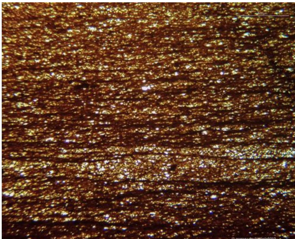
Plane polarised light photomicrograph of sample 163462 (x4) illustrating fine grained foliated texture with two foliations.
