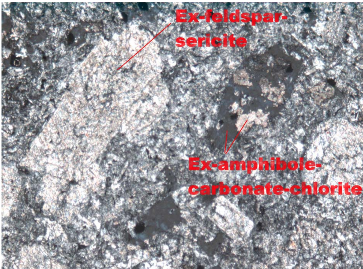
Figure 2. Specimen MM07 DD05 - 68.53-68.66. Altered porphyritic dolerite. WOF c5.6mm.
