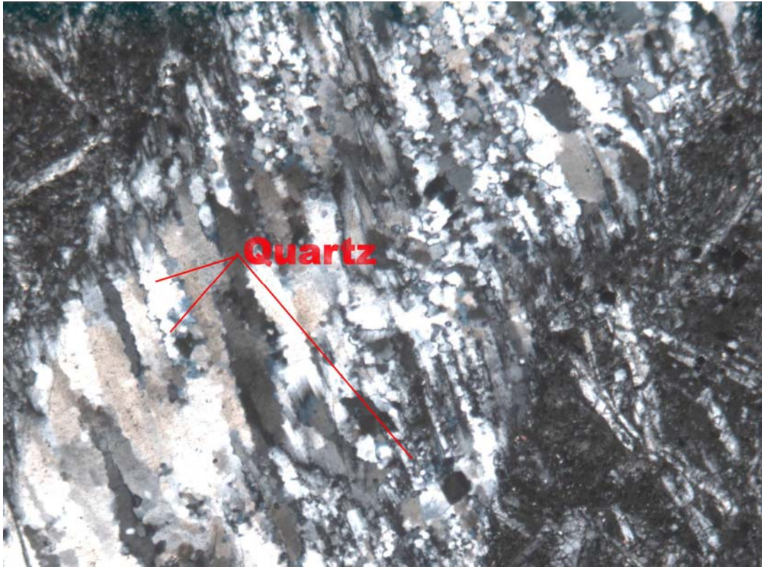
Figure 35. Specimen MM07 DD05 - 176.73-177.03. Deformed quartz vein in basalt/dolerite. WOF c2.8mm.
