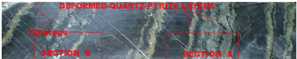
Figure 10. Specimen MM07 DD05 - 80.35-80.65. Meta-pelite – meta-arenite, foliated + deformed sulphide-quartz layers (cleavage overprint). WOF c30cm.
