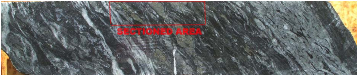
Figure 21. Specimen MM07 DD05 - 168.06-168.30. Meta-pelite – meta-arenite with paler carbonate rich layers. Late carbonate (white) and sulphide (yellow). WOF c24cm.
