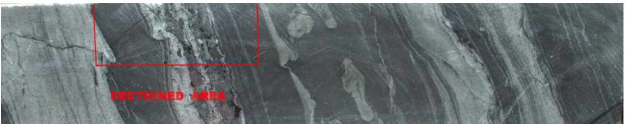
Figure 16. Specimen MM07 DD05 101.75-107.0. Metapelite – meta-arenite (+ fragmental layer) – foliated. WOF c25cm.
