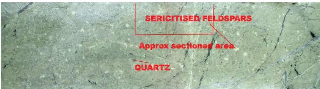
Figure 28. Specimen MM07 DD05 - 171.18-171.43. Altered porphyritic dolerite. WOF c24cm.
