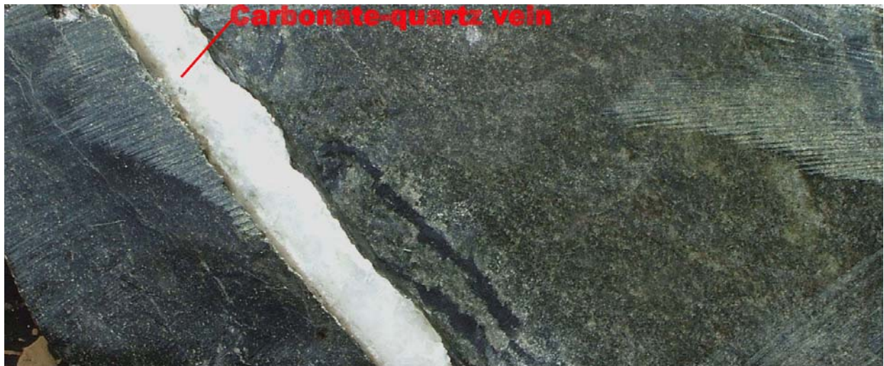
Figure 19. Specimen MM07 DD05 138.70-138.80. Altered dolerite + quartz carbonate vein. WOF c12.0cm.
