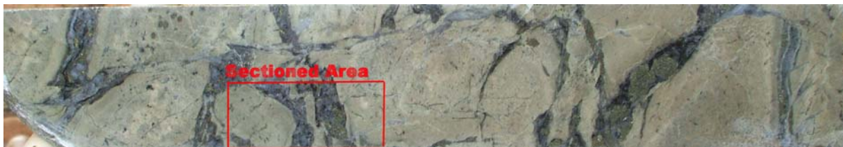
Figure 34. Specimen MM07 DD05 - 176.73-177.03. Altered dolerite/basalt with deformed quartz-sulphide-veins. WOF c30cm.
