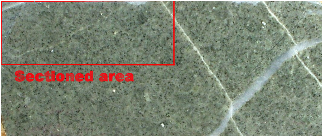
Figure 1. Specimen MM07 DD05 - 68.53-68.66, altered porphyritic dolerite. White carbonate vein, cutting grey quartz. Width of frame (WOF) c10.1cm.
