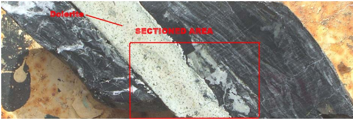
Figure 3. Specimen MM07 DD05 - 71.30-71.42. Altered porphyritic dolerite. WOF c10cm.
