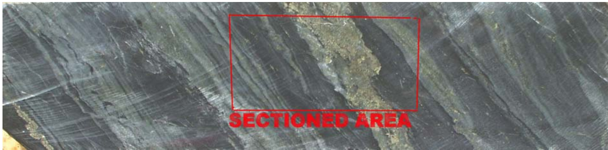
Figure 6. Specimen MM07 DD05 - 77.30-77.50. Foliated meta-pelite - meta-arenite + deformed quartz sulphide vein. WOF c18cm.
