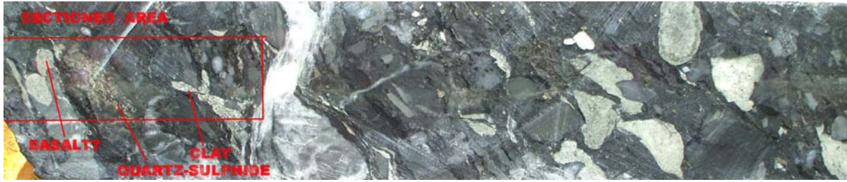
Figure 24. Specimen MM07 DD05 - 168.70-168.95. Deformed fragmental meta-sediment + quartz-sulphide vein. WOF c24cm.
