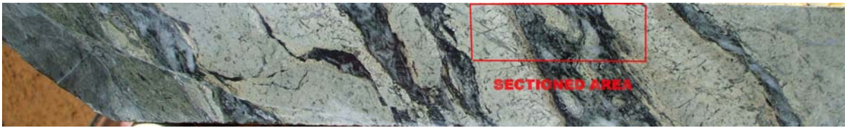
Figure 30. Specimen MM07 DD05 - 173.25-173.60. Altered porphyritic dolerite, quartz veins, and dark clay veins. WOF c30cm.
