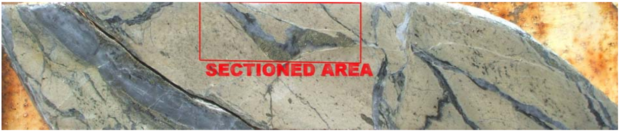
Figure 32. Specimen MM07 DD05 - 175.0-175.25. Altered porphyritic dolerite/basalt, + deformed quartz-sulphide veins. WOF c20cm.
