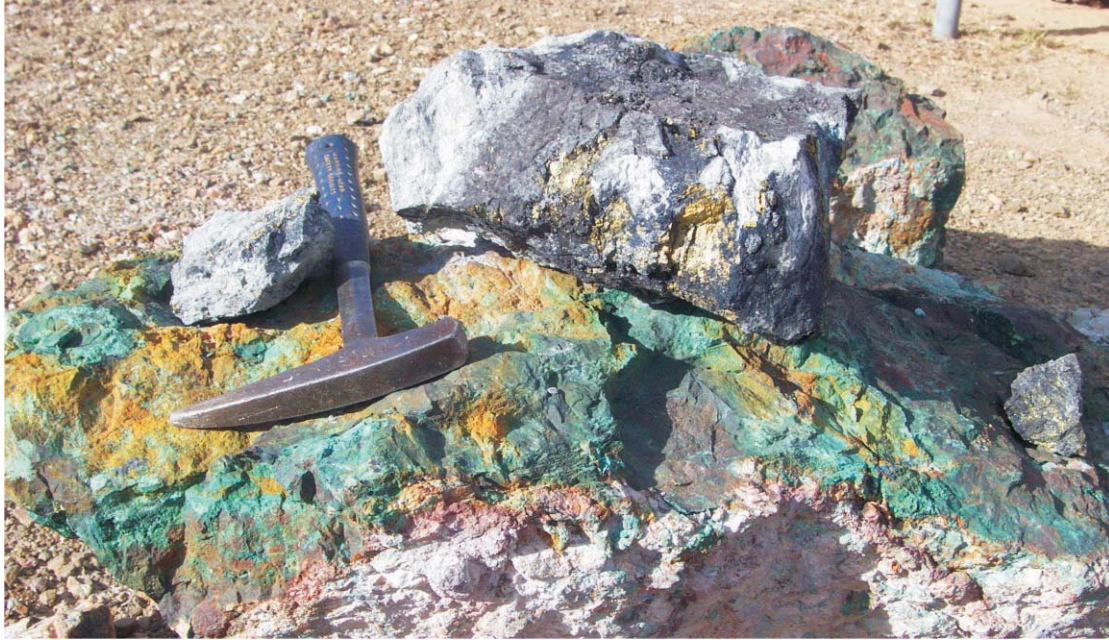
Plate 21: Tartana West oxide ore, copper carbonate, black oxide and chalcopyrite
