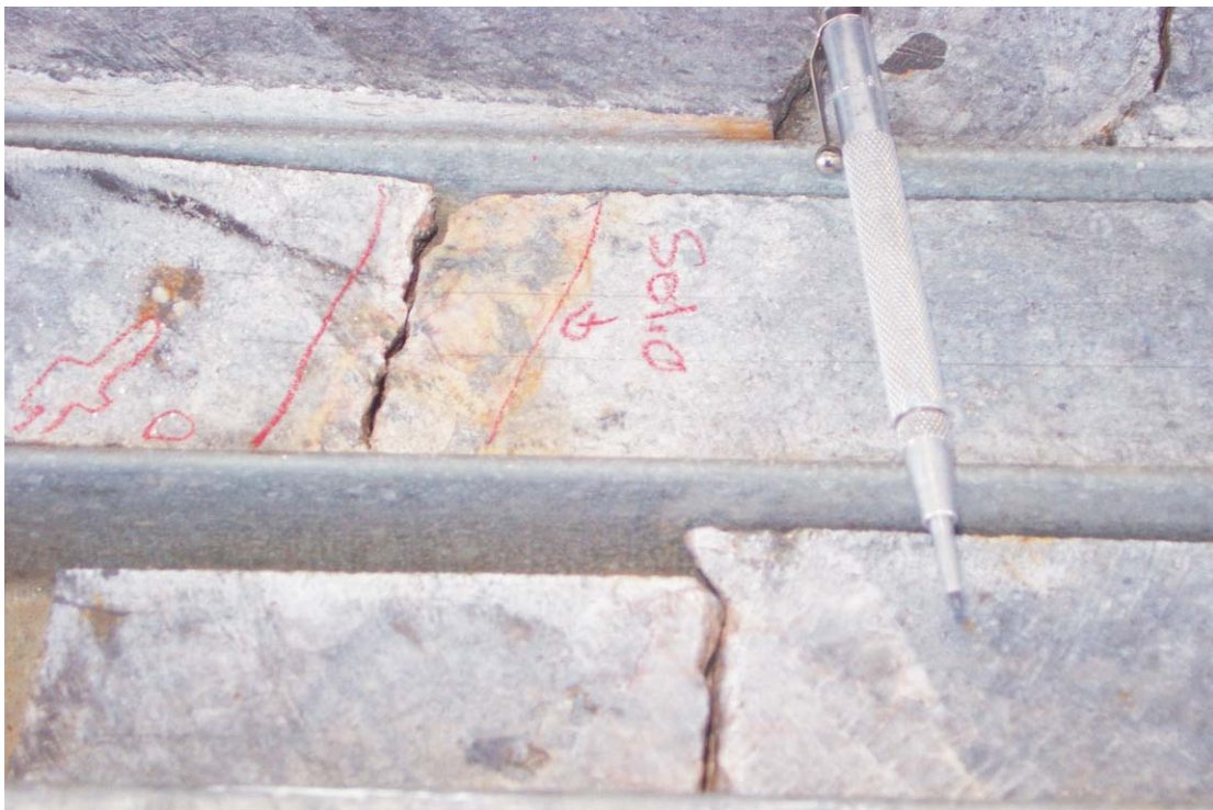
Plate 5: Watershed Grid core (scheelite is outlined in red)
