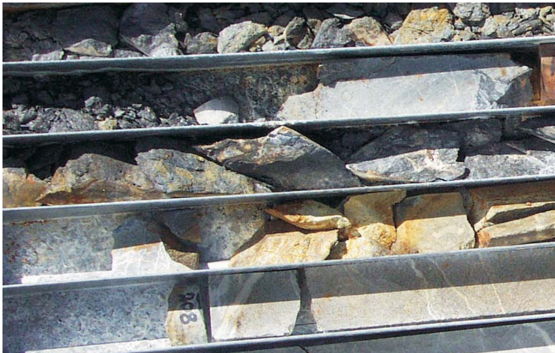
Plate 6: Tregoora core, anomalous gold assay values mainly associated with the competent sandstone and not with the carbonaceous shale
