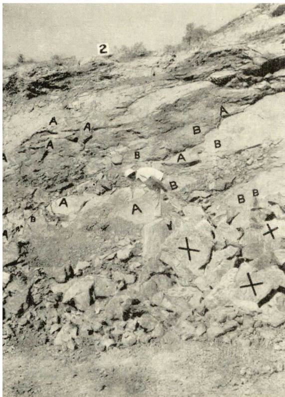
Mary Kathleen open-cut bench shows the classification of the rock face into A and B class ore, and waste (indicated by crosses) to enable selective mining.
