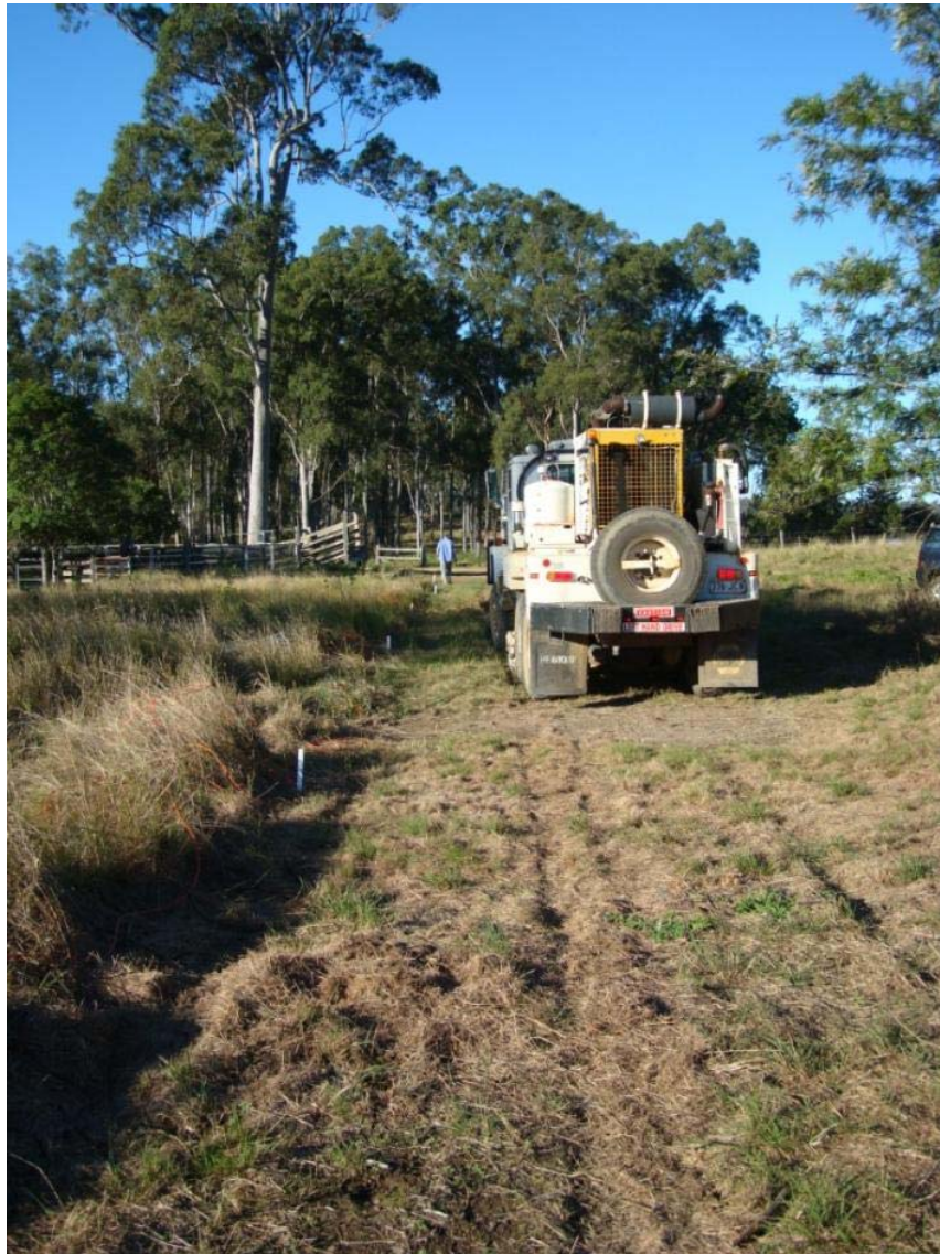
Hemi 44 seismic vibrator truck
