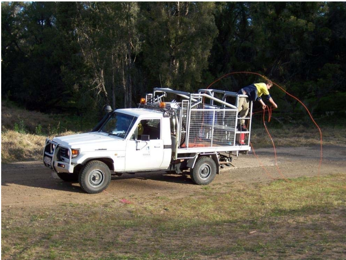
Line vehicle deploying cable.
