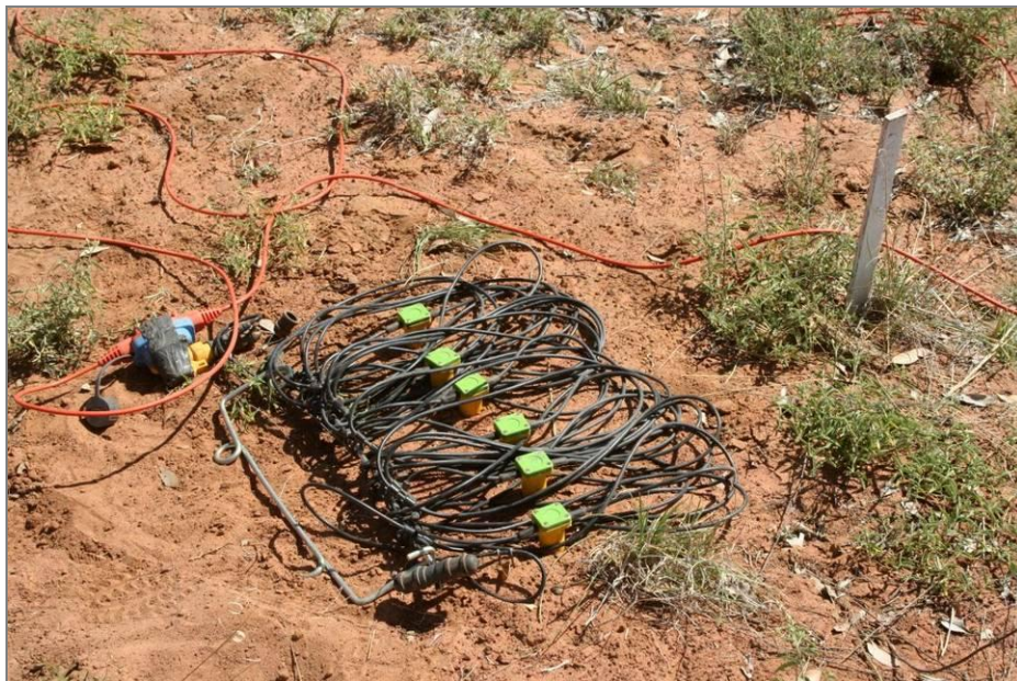
Figure 4: An example of the geophone array on the Aramac 2D
