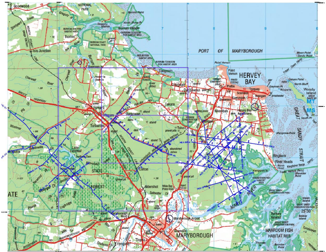
Figure 5 Shotpoint basemap showing BE08 Maryborough and existing seismic surveys within and adjacent to ATP 613P
