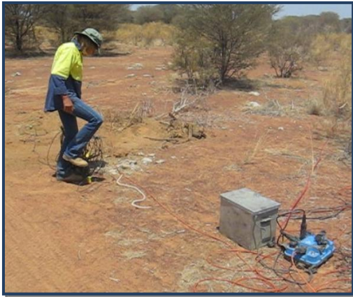
Photo 7: Planting geophones (left) and picking up cables (right)
