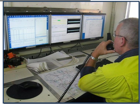
Photo 8: Sercel 428XL recording truck and instruments
