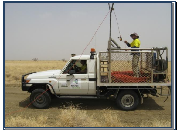
Photo 7: Planting geophones (left) and picking up cables (right)
