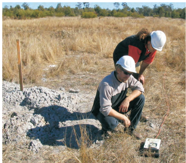
Figure 4: Typical TSIM operation. The TSIM instrument with trailing antenna is traversed taking passive apparent resistivity measurements at a set spacing.
