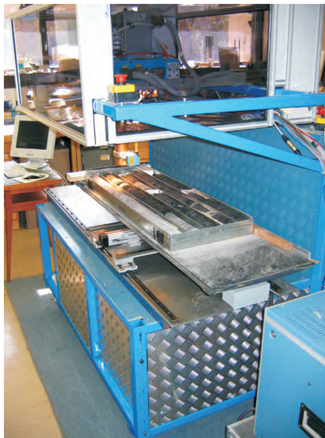
Figure 1: Coal core tray under the HyLogger™. The tray sits on a robotic X-Y table and the tray sections are moved under the spectrometer that sits in the overlying enclosed cabinet.
