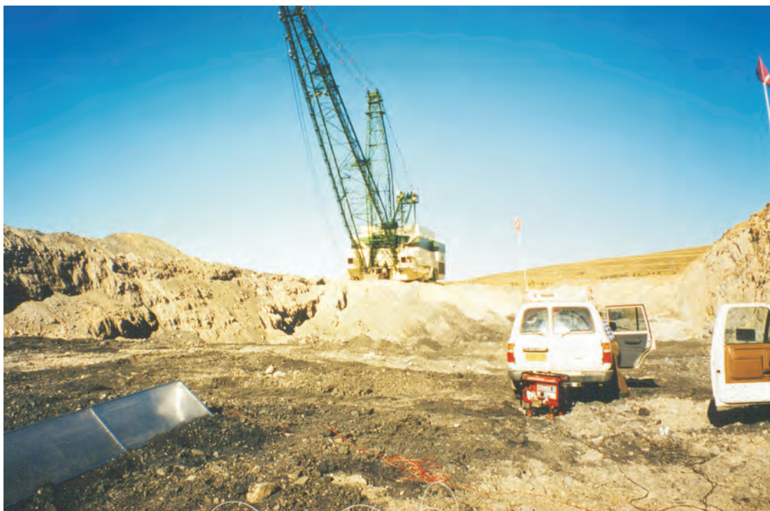
Figure 1: Chamber method used for surface emissions; chamber on the left is connected to gas analysers and loggers which are installed in the 4WD on the right.
