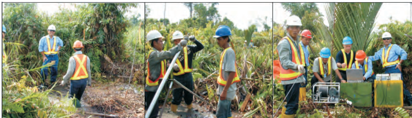
Figure 5: (i) Drill pad, the stick with flagging tape on the right marks the collar location. (ii) Preparing to Geophysically log the hole. The tool is about to be lowered down the hole over the tripod in the foreground. The personnel in the background control the computer and logging unit. (iii) Logging the hole. The cable is lifted up manually away from water and weeds.
