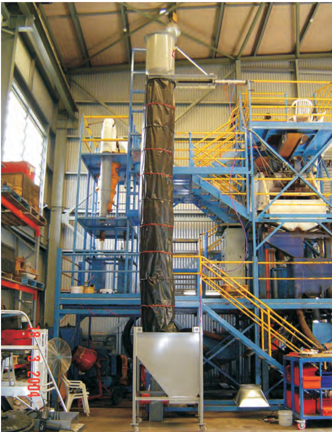
Figure 1: Pilot/ laboratory scaled loadout with the hopper slide gate located 7m above rail
