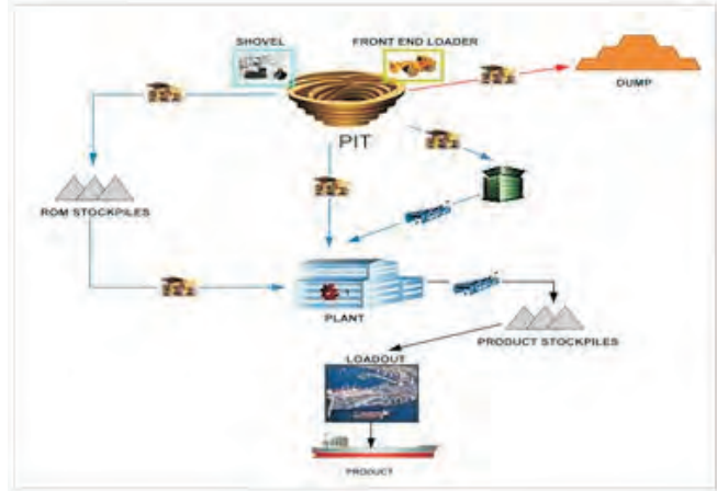
Figure 4: Schematic of typical coal mining operation.
