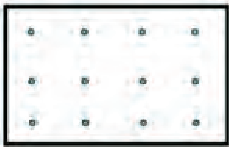
Figure 6: Diagram illustrating a systematic fixed sampling grid.
