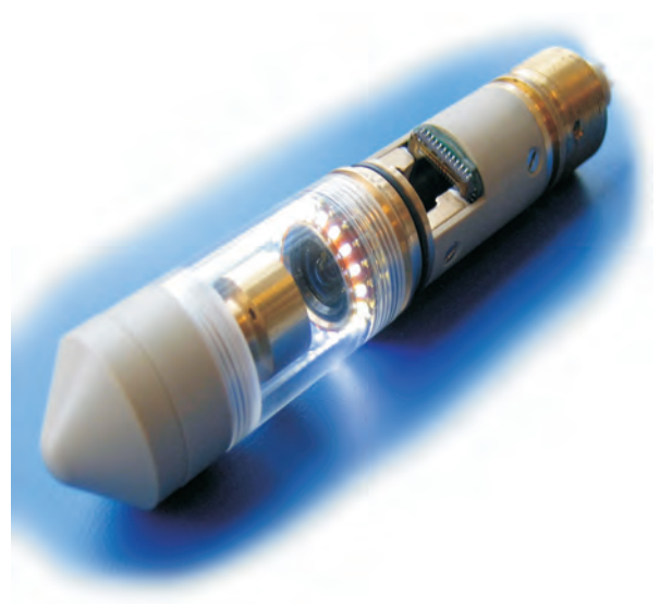
Figure 1: The digital video module of the SBS system.
