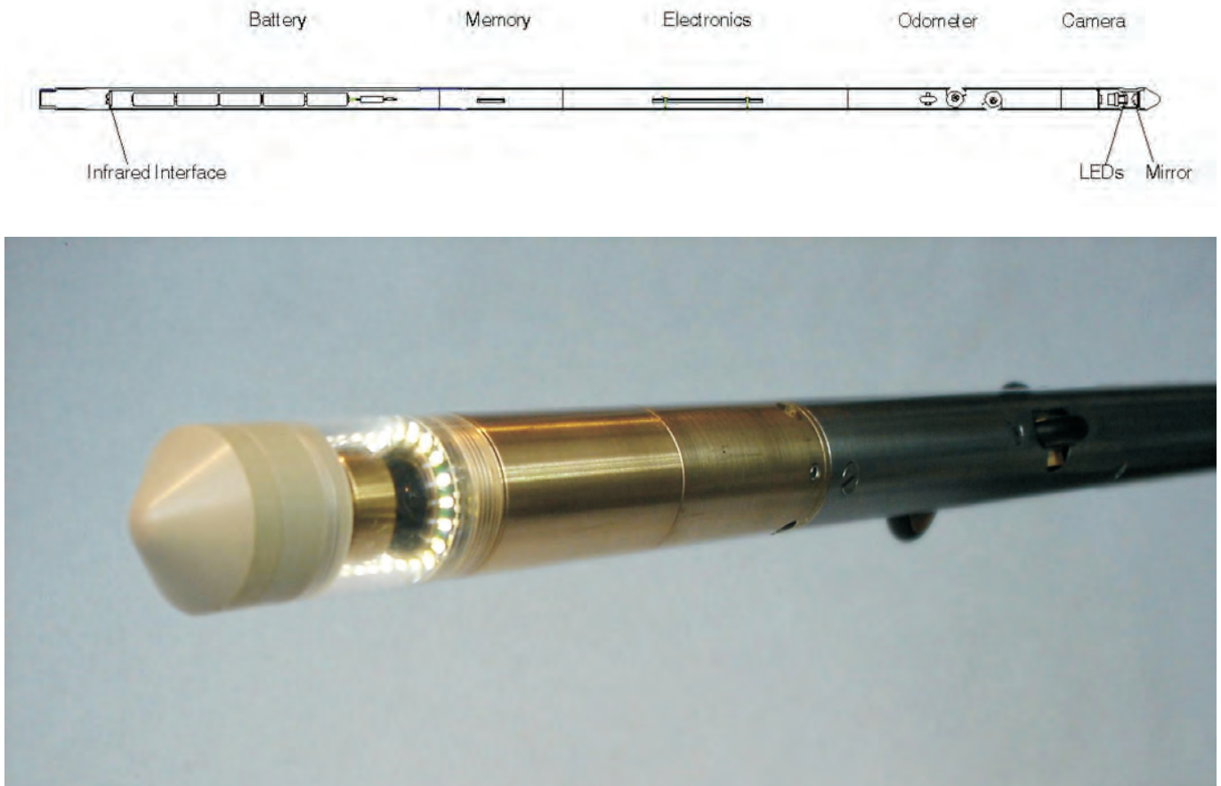
Figure 4: The digital video module of the SBS. A schematic of the tool appears above the main image.
