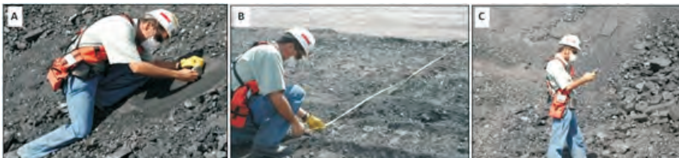
Figure 9: Series of photographs, illustrating the functions of the in-pit geologist (Ramón Daza). A: Structural points of observation, (dip and strike), B: Certified thickness measurements, and C: Seam traces with GPS.
