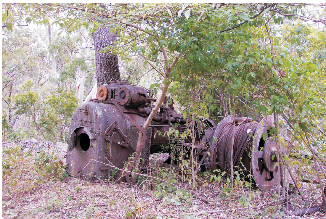
Photo 4: Remains of winding gear, Welcome mine, Normanby Goldfield
