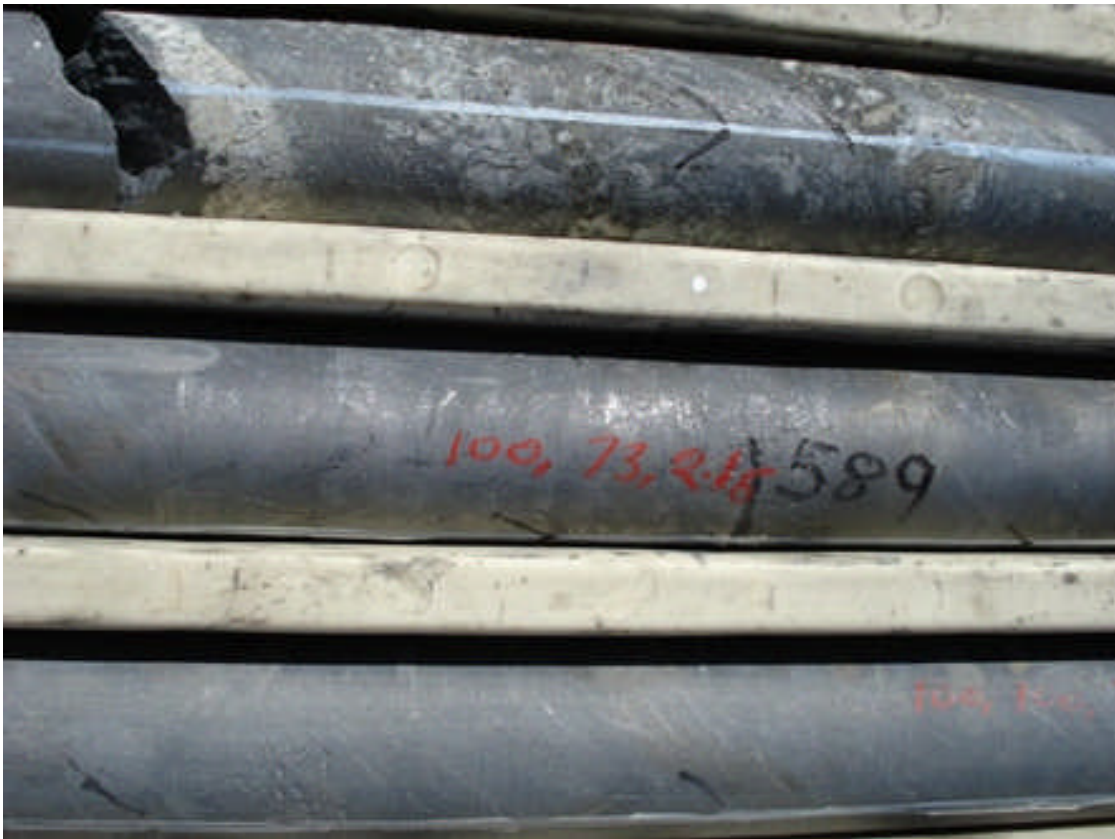
Figure 5: Drill core photograph - SXDD003, 589m - Graphitic schist with up to 80% crystalline graphite, and minor feldspar/quartz
