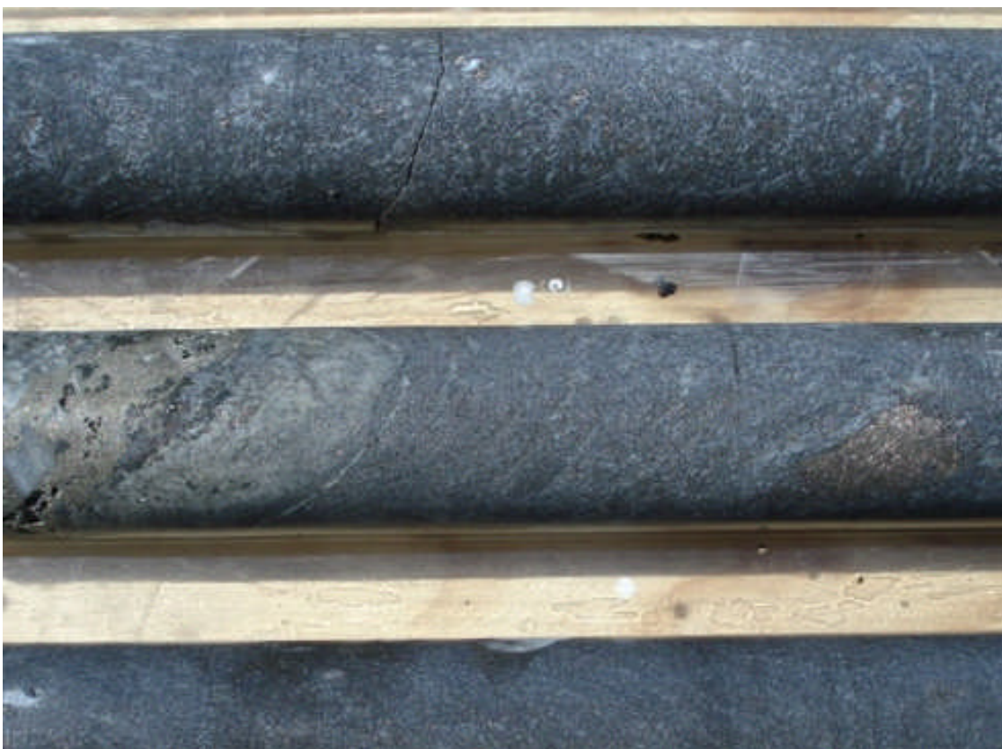
Figure 6: Drill core photograph - SXDD003, ~ 678m - Graphite-sillimanite schist with up to 20% pyrrhotite and minor chalcopyrite.
