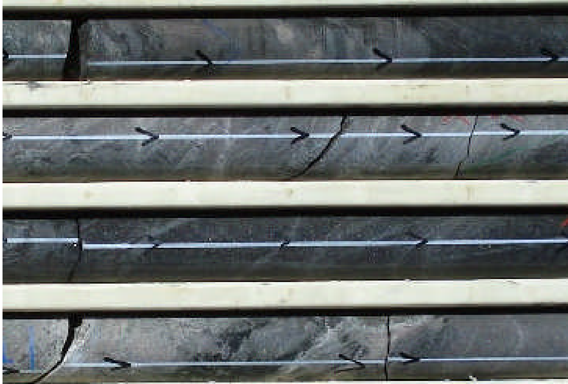
Figure 7: Drill core photograph - SXDD003 ~ 811m - Calc-silicate gneiss, at times intercalated with graphitic schist.
