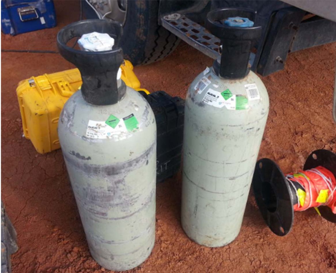
Figure 5- CO2 Liquefied Gas use by HNGS detector.
