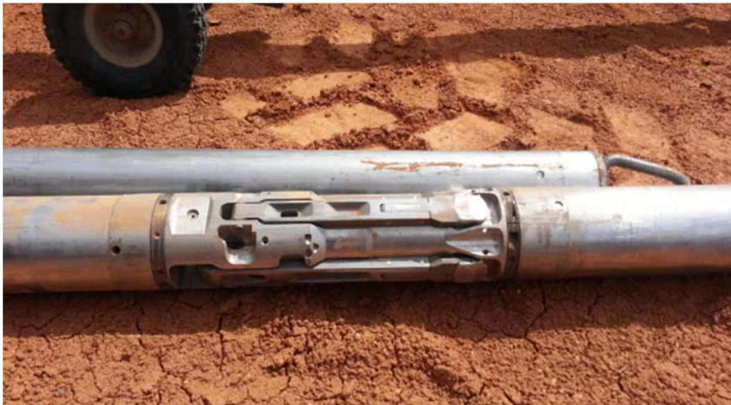
Figure-2 PPC-Powered Caliper used for short-axis kit.
