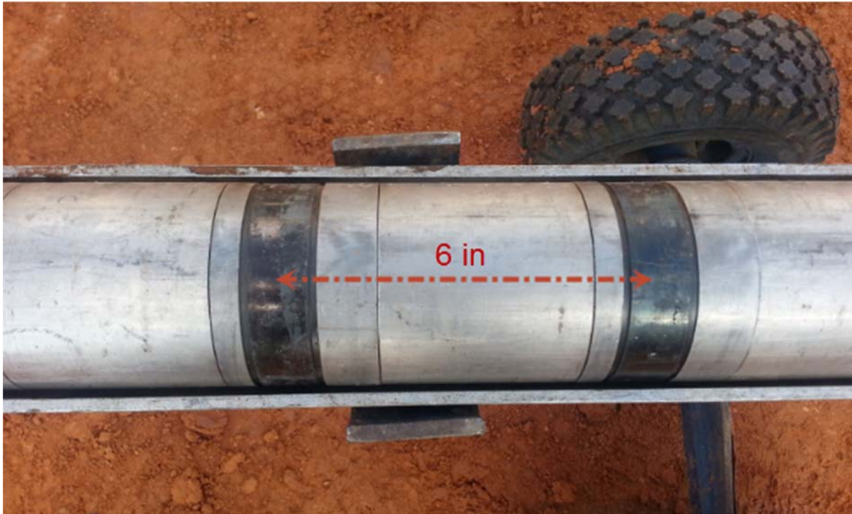
Figure 3- MAST- Sonic Scanner receiver for monopole and dipole
