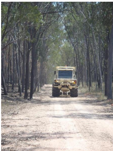
Picture 2: Vibrator working along minor road in Pinelands area
