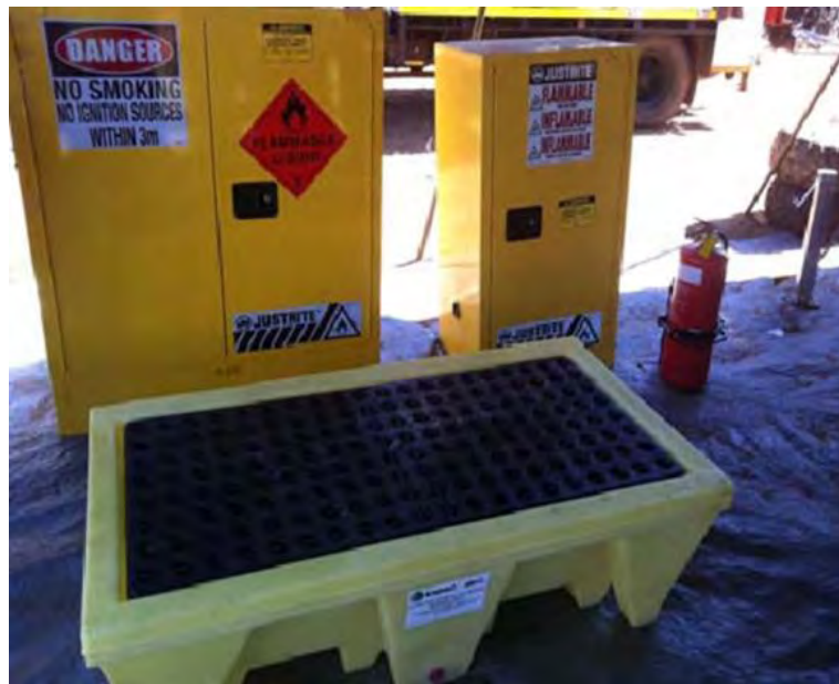
Figure 80. Spill Containment and Segregation
