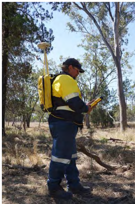
Figure 11. RTK survey by backpack
