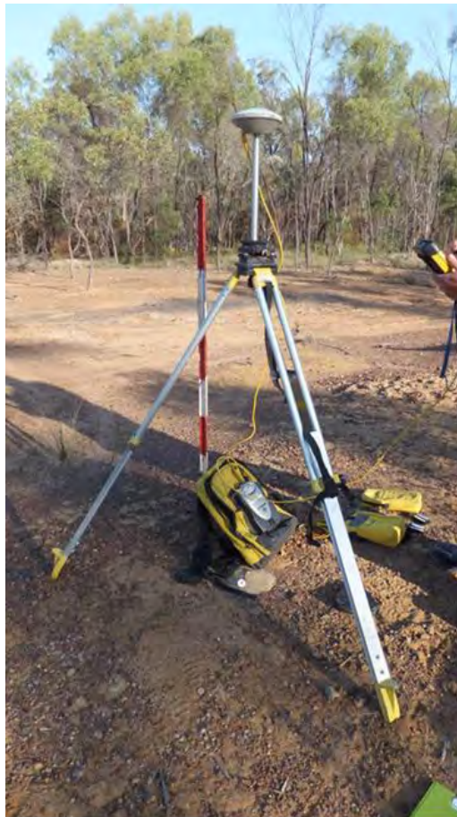
Figure 8. Static observation on 185028 national control network
