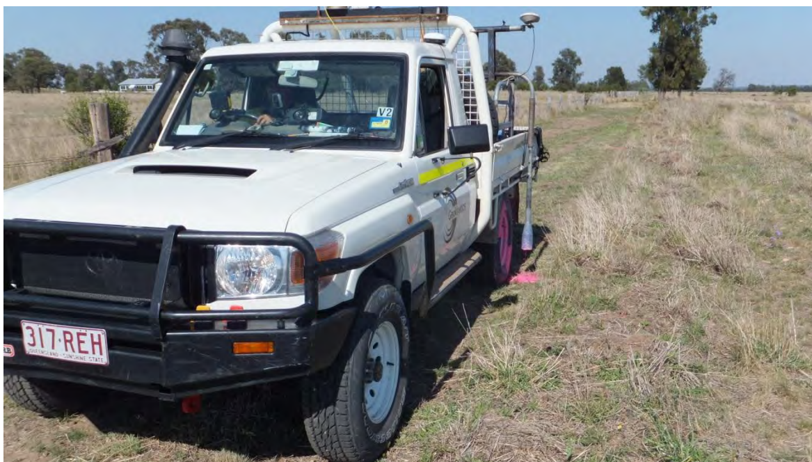
Figure 6. Degradable paint spraying machine mounted below GPS antenna
