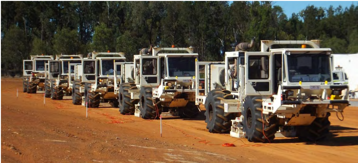
Figure 22. Crew 488 Vibroseis Units at star-up test
