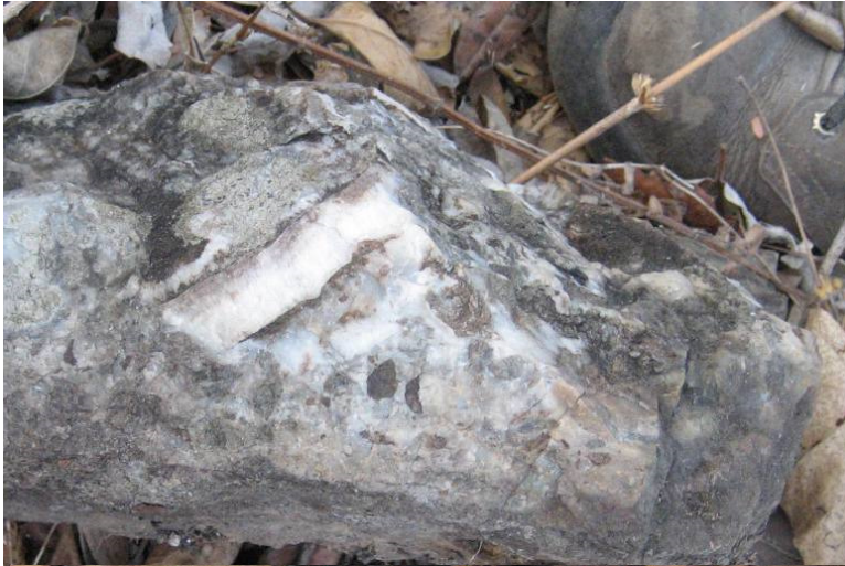
Photo 1: Great Northern Breccia: Quartz veins, brecciated and re-cemented by silica in at least two differing phases. Country rock granites – sericitic altered.
