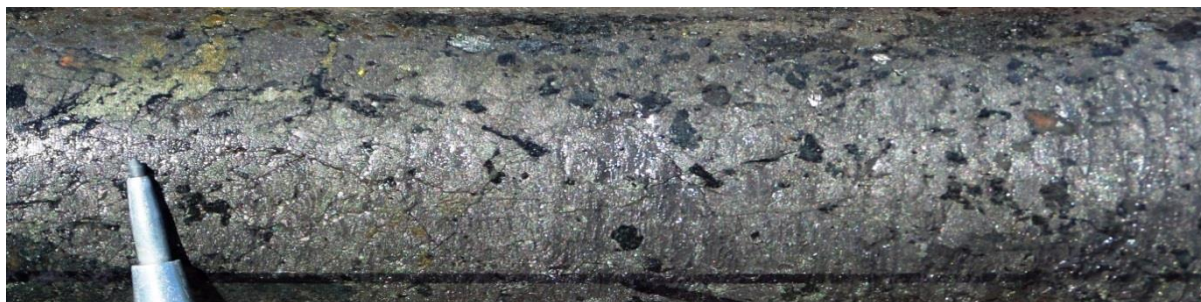
Figure 24: MN13D30 at 168.30m. Massive pyrrhotite-rich breccia with minor chalcopyrite, pyroxene and angular quartz clasts
