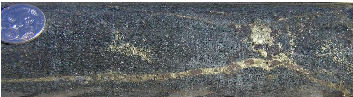
Figure 34: Chalcopyrite +pyrrhotite vein within metasomatite at 168.9 m in drill hole MN12D28
