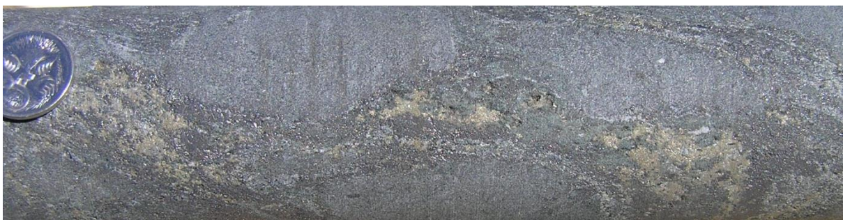
Figure 38: Breccia with dacite clasts and matrix of magnetite, pyrite and clinopyroxene at 199.7 m in drill hole MN12D29
