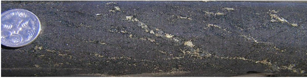
Figure 35: Pyrite and chlorite veinlets in fine-grained dacite at 165.9 m in drill hole MN12D29
