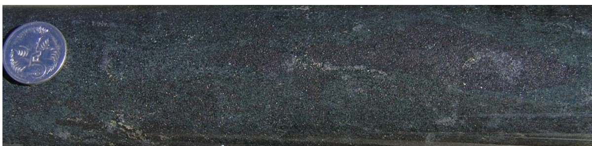
Figure 40: Magnetite clasts within clinopyroxene matrix at 288.5 m in drill hole MN12D29
