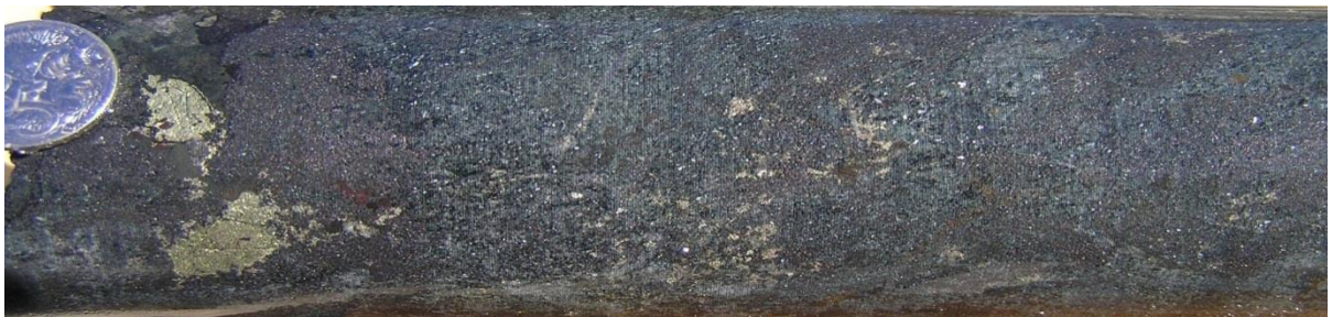
Figure 36: Magnetite +clinopyroxene +chalcopyrite alteration at 166.9 m in drill hole MN12D29
