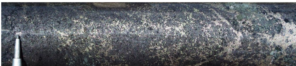
Figure 28: MN13D30 at 373.00m. Magnetite alteration zone also containing amphibole, pyrrhotite and trace chalcopyrite
