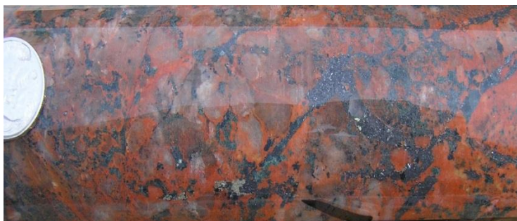
Figure 13: Coarse-grained granite with red-rock alteration at 83.9 m in drill hole MN11D24
