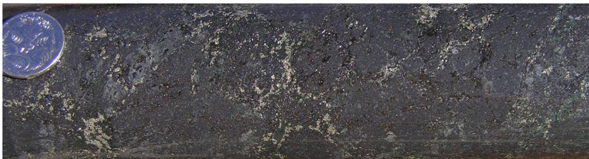
Figure 39: Porphyritic dacite with irregular sulphide veinlets at 273.5 m in drillhole MN12D29
