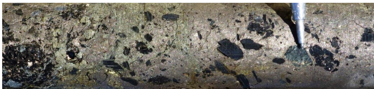
Figure 21: MN13D30 at 109.35m. Massive pyrrhotite breccia containing lesser chalcopyrite and pyroxene
