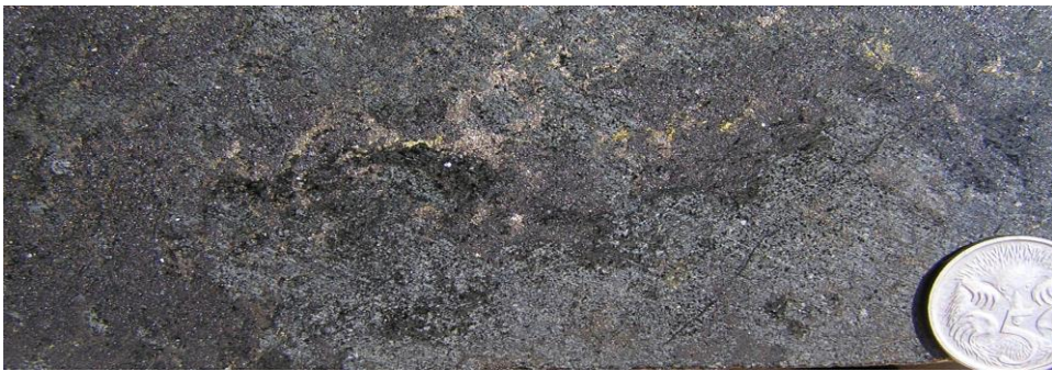
Figure 16: Magnetite- and amphibole-bearing alteration zone at 107.1 m in drill hole MN11D20
