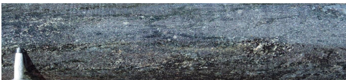
Figure 45: MN13D31 at 197.00m. Strong foliation (parallel to core axis) within magnetite-rich brecciated dacite
