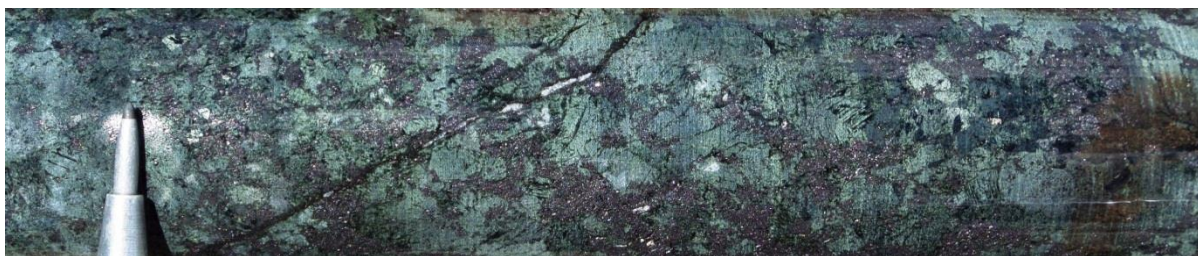
Figure 29: MN13D30 at 385.00m. Coarse-grained magnetite and pyroxene alteration zone
