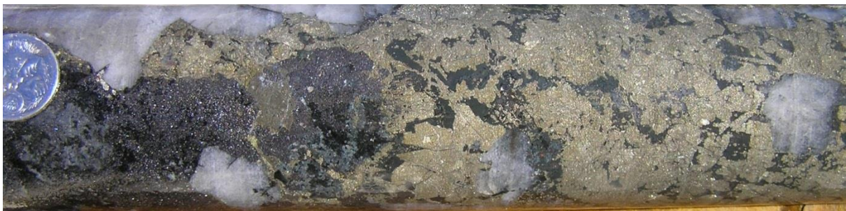
Figure 37: Coarse nickeliferous pyrite, quartz, magnetite alteration zone at 173.6 m in drill hole MN12D29
