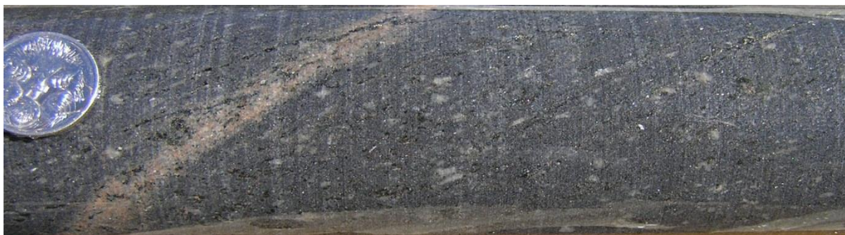
Figure 32: Light-grey, fine-grained weakly-foliated porphyritic dacite at 131.6 m in drill hole MN12D28
