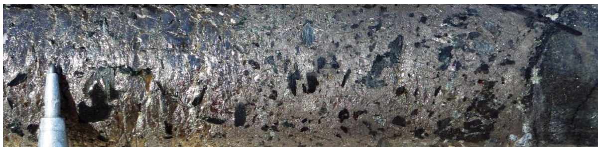
Figure 25: MN13D30 at 238.60m. Pyrrhotite-rich breccia containing amphibole/pyroxene crystals
