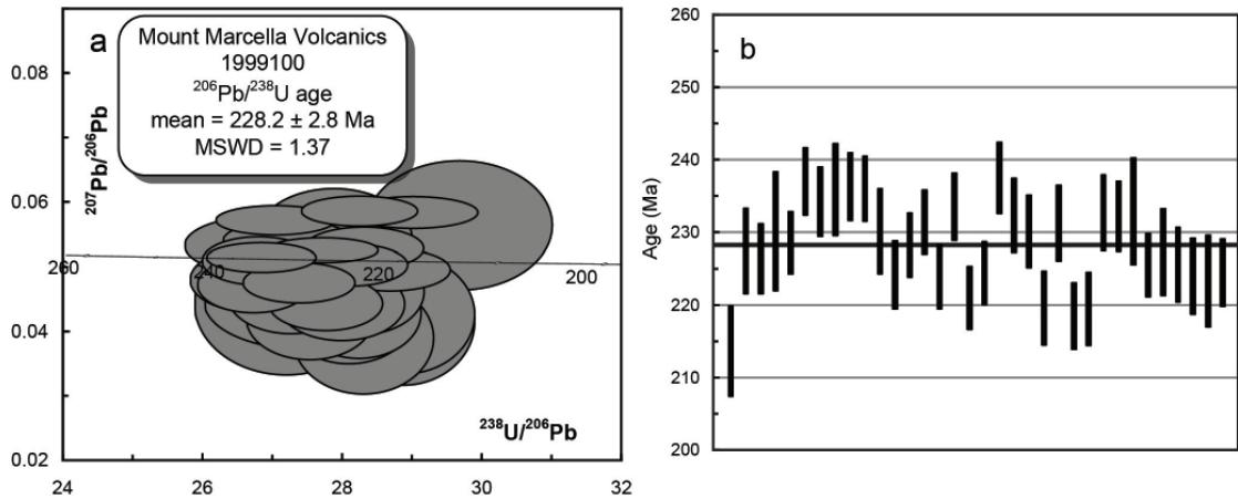
Figure 14. (a) Tera-Wasserburg concordia plot and (b) temporal trend of the  $^{206}\text{Pb}/^{238}\text{U}$  ages from the Mount Marcella Volcanics (1999100)
