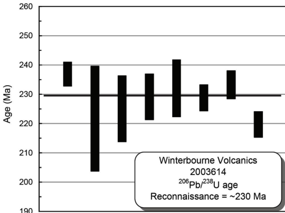
Figure 24. Temporal trend of the  $^{206}\text{Pb}/^{238}\text{U}$  ages for the Winterbourne Volcanics (2003614). This result is interpreted as reconnaissance in nature as the few zircons that were analysed have very high  $^{206}\text{Pb}_c$  proportions.
