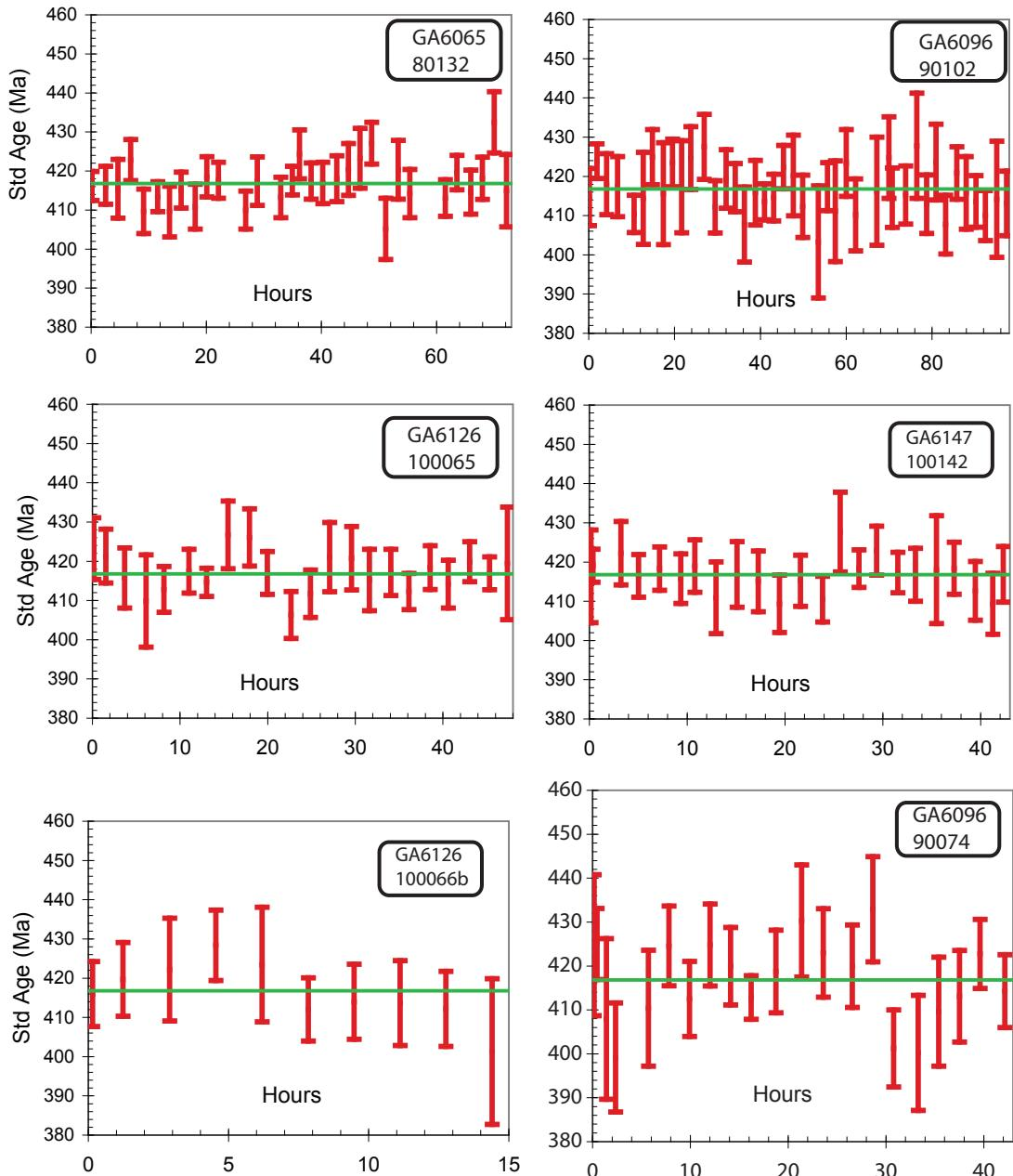
Figure 2. Temporal trend of the  $^{206}\text{Pb}/^{238}\text{U}$  ages for the TEMORA 2 zircon standard for the analytical sessions used in this study (error bars are  $2\sigma$ ). See Table 2 and Appendix 1 for further session details.
