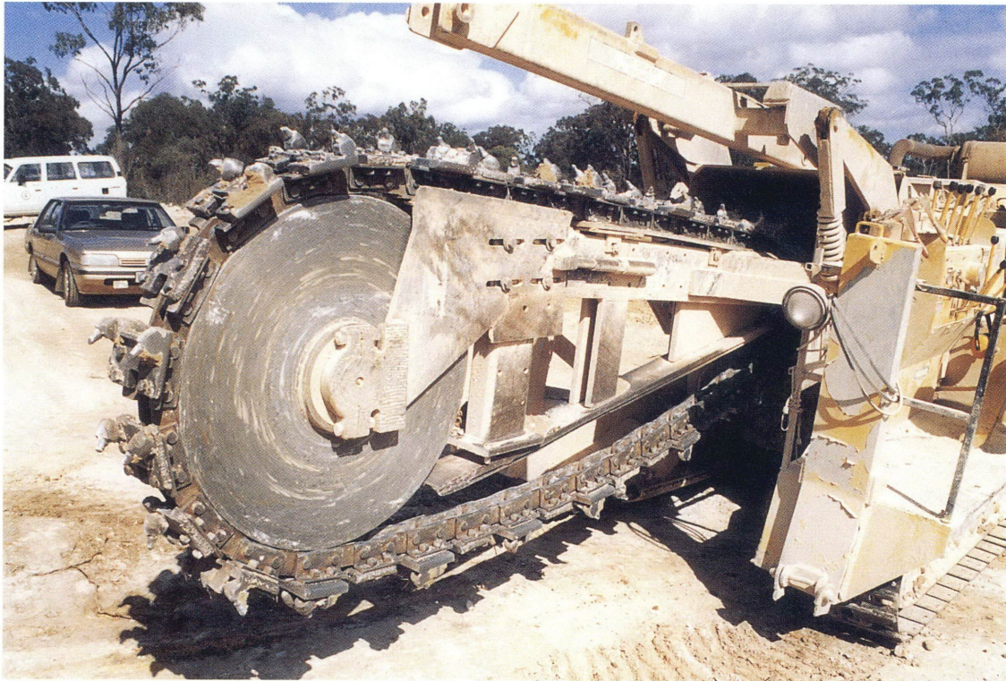
Figure 22: Trenching machine, Helidon Sandstone quarry; J.H.Wagner and Sons Pty Ltd
