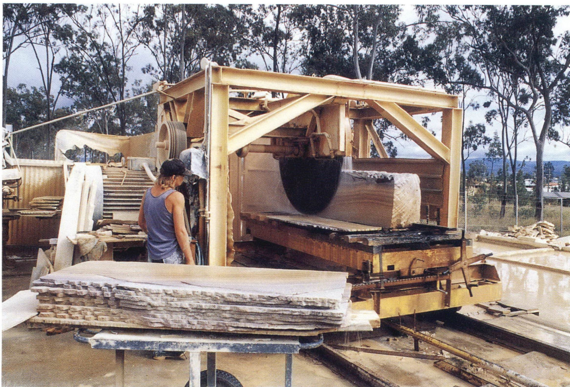
Figure 23: Diamond-bladed block saw, Helidon Sandstone; Lockyer Sandstone Company
