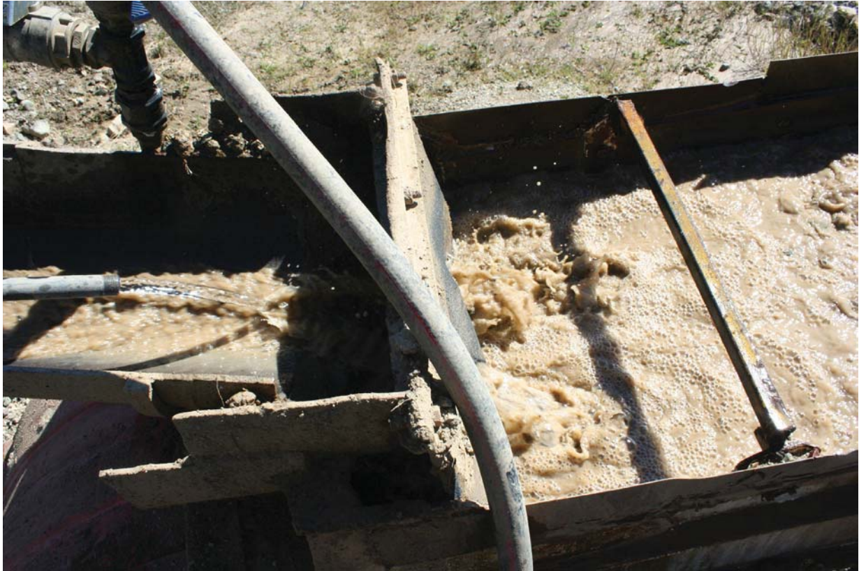
Photograph 135: Sluice box with carbon matt for collecting fine alluvial gold from gravel at the Prophet Gold Mine, Kilkivan.
