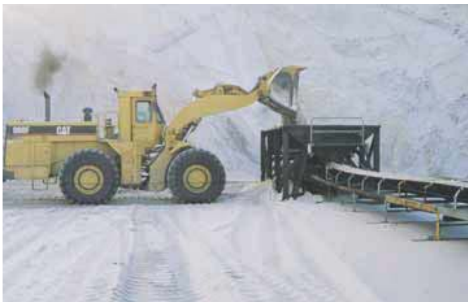
Photograph 216: Bulk loading of silica sand in conveyor belt to the wharf at Cape Flattery (image courtesy DNRM, Queensland Mineral and Petroleum Review, 2002).
