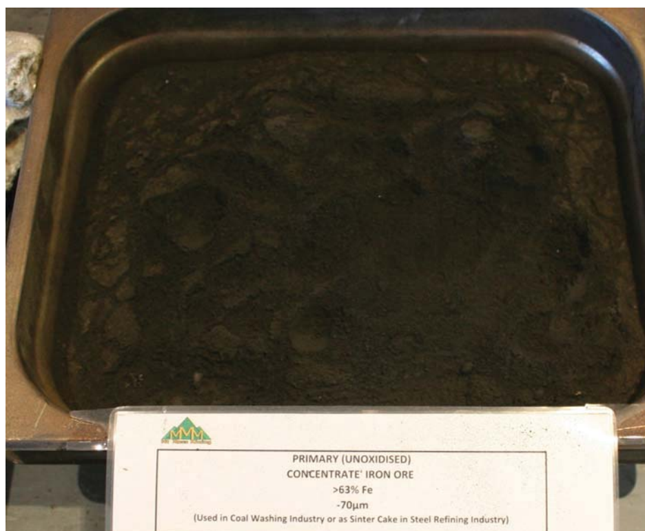
Photograph 136: Primary (unoxidised) iron ore concentrate at -70µm (>63% Fe) produced at Mount Moss, (this product is used in the coal washing industry or as sinter cake in the steel refining industry).
