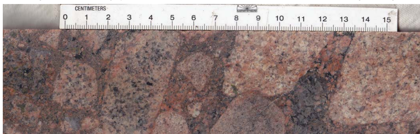
Photograph 64: Milled breccia with polymictic clasts of granite and granodiorite in fine molybdenum-rich matrix Wingfield Granodiorite of the Rawbelle Batholith, Whitewash South prospect.
