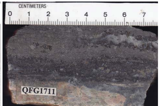
Photograph 116: (left) Gold and base metal (mostly lead and zinc) in a silicified porphyry breccia from Horn Island; (right) massive sphalerite, chalcopyrite and galena bands as vein-infill from Horn Island.
