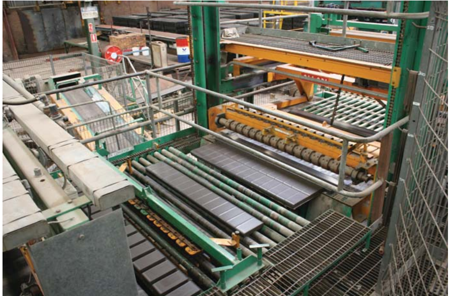
Photograph 219: Automated cutting of clay pavers prior to kiln firing at Claypave's Dinmore plant
