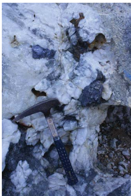
Photograph 156: Wolframite and molybdenite mineralisation in Wolfram Camp open cut.
