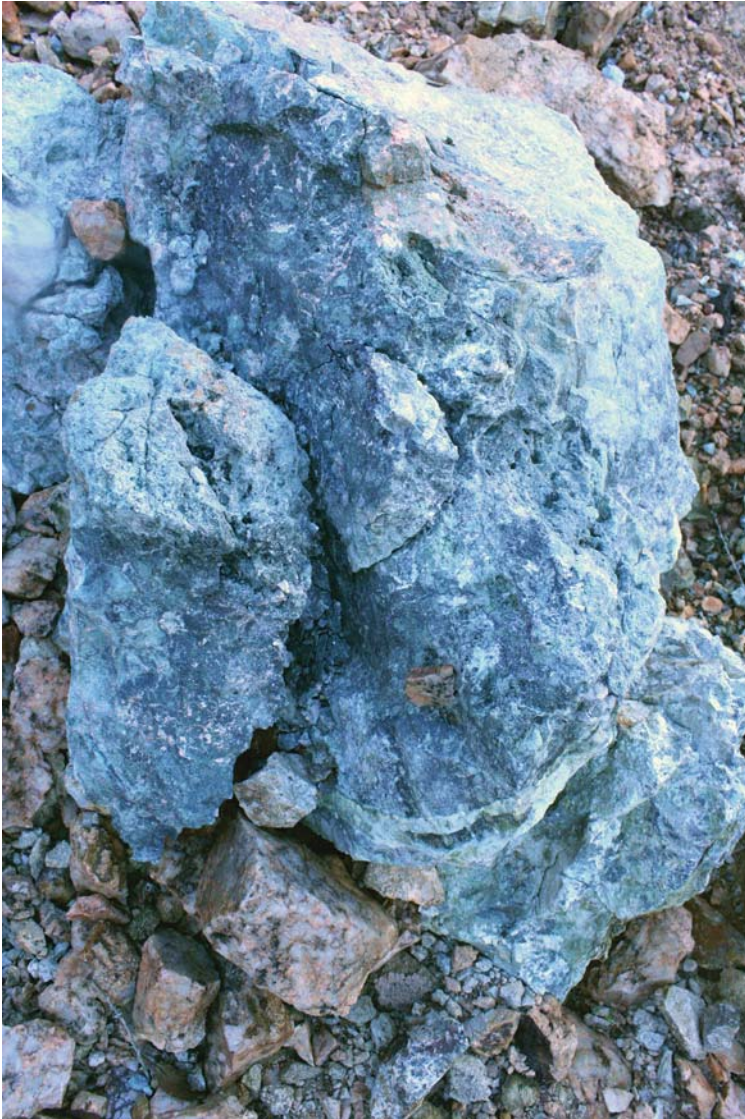
Photograph 131: Sulphide mineralisation (arsenopyrite with gold) from an ore lens in the Lorena Gold mine open cut.
