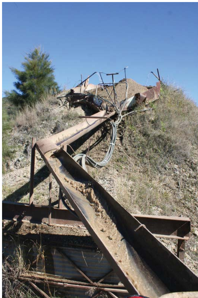
Photograph 134: Processing of alluvial gravel at the Prophet Gold Mine, Kilkivan.
