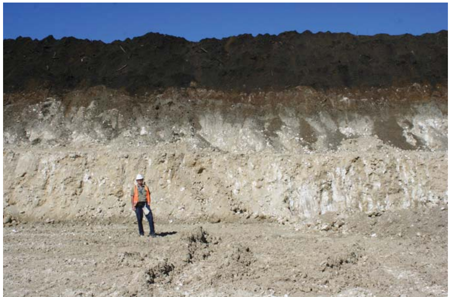
Photograph 203: Light-coloured magnesite nodular horizon under black clay-soil overburden at Pit 23, Kunwarara Magnesite mine.
