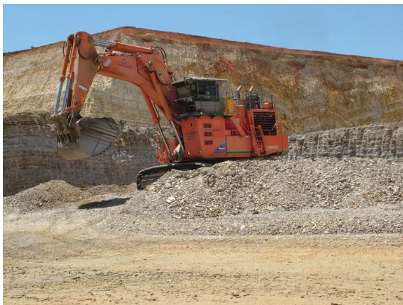
Photograph 212: Mining phosphate rock from flat-lying phosphatic siltstone within the Beetle Creek Formation at Phosphate Hill (image courtesy David Carmichael, 2007, DNRM).
