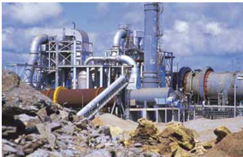
Photograph 232: Stage one Stuart Oil Shale plant; rotary dryer and processor (image courtesy QER Pty Ltd, Queensland Mineral and Petroleum Review, 2002)
