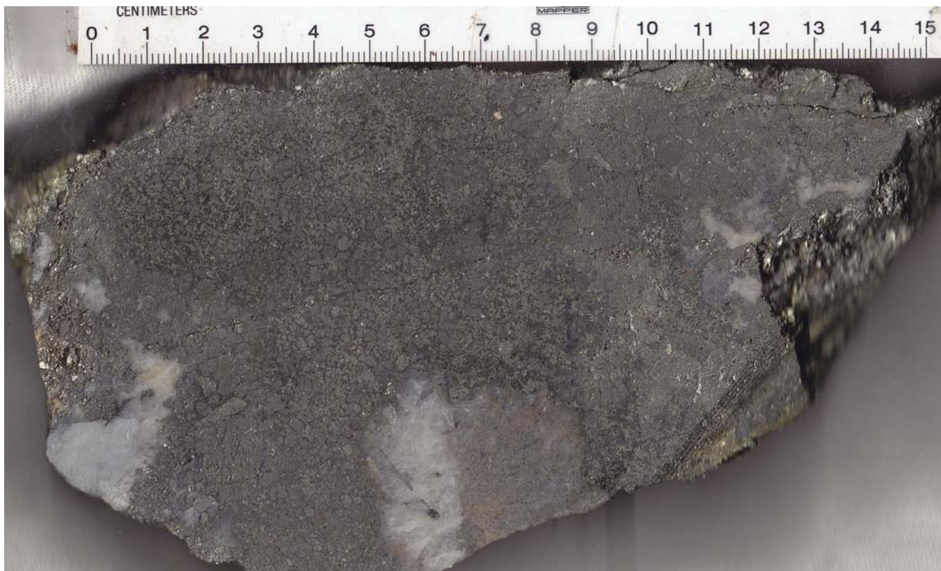
Photograph 52: Sulphide (chalcopyrite) mineralisation from Great Australia mine.
