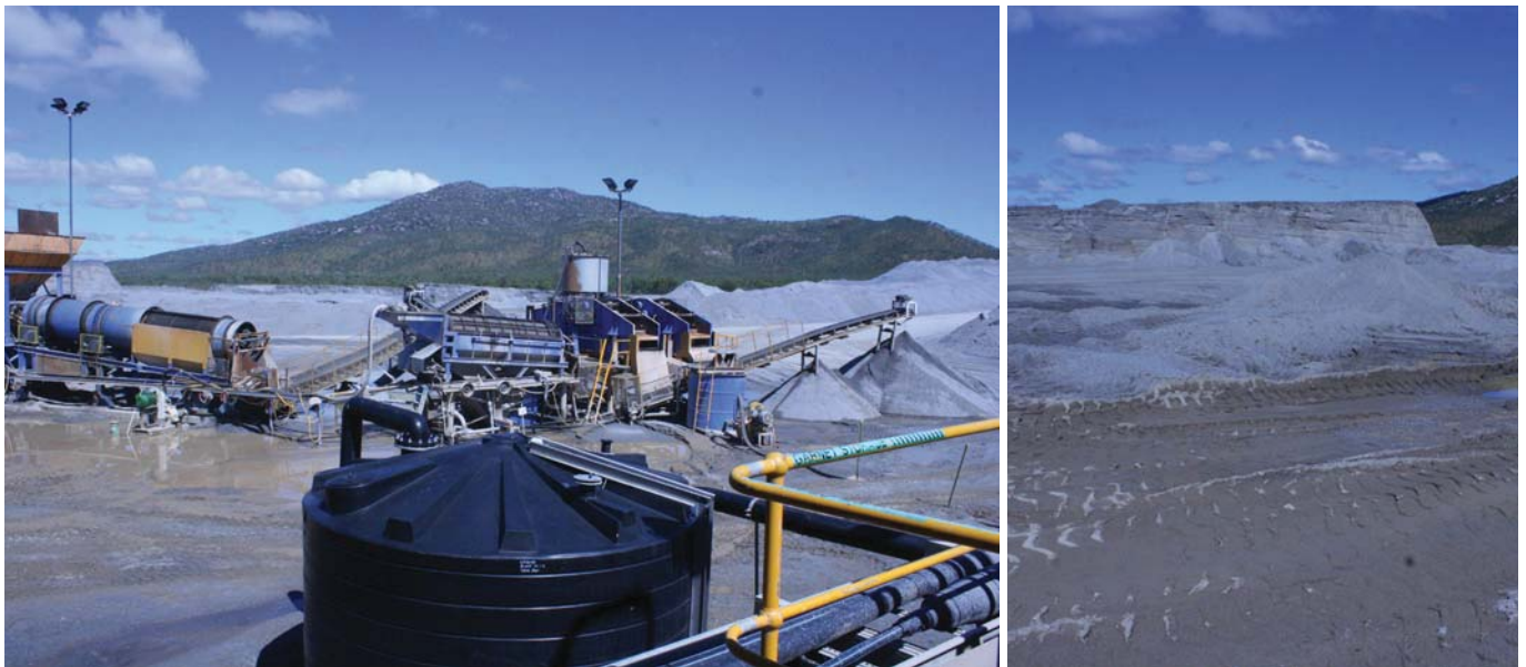
Photograph 162: (left) Mount Carbine tailings retreatment plant; (right) Mount Carbine tailings dam currently being re-worked. Note the fine layering in the material in the background.
