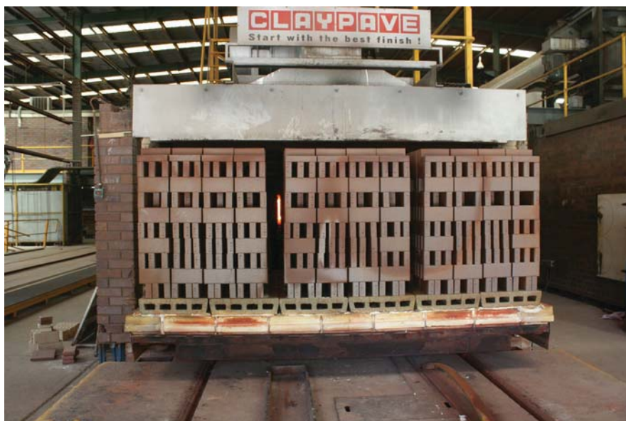
Photograph 221: Clay pavers stacked loosely for firing in Kiln train at Claypave's Dinmore plant
