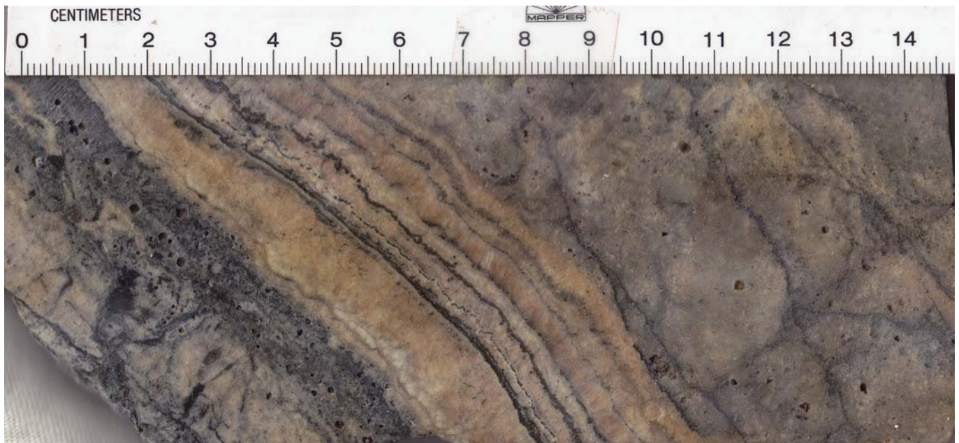
Photograph 96: Banded open space fill alunite-sphalerite-pyrite-engargite veins from V2, within the Mount Carlton Project.
