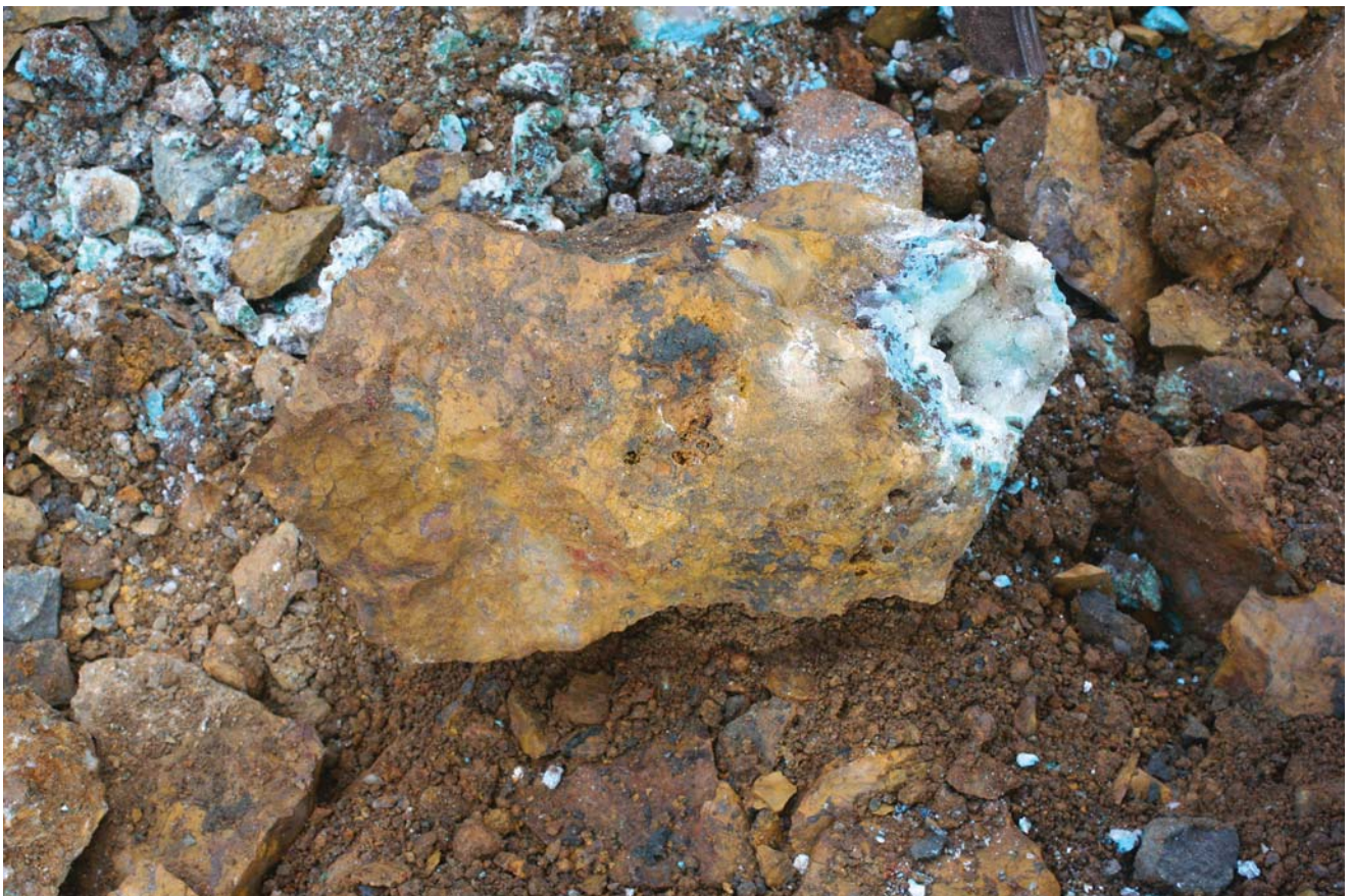
Photograph 51: Chrysocolla, cuprite and quartz mineralisation from the oxidised zone at Great Australia mine.
