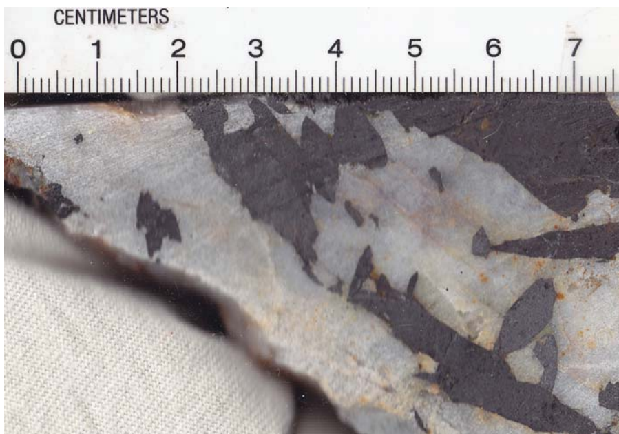
Photograph 155: Tungsten quartz vein mineralisation from Mount Carbine wolfram mine.
