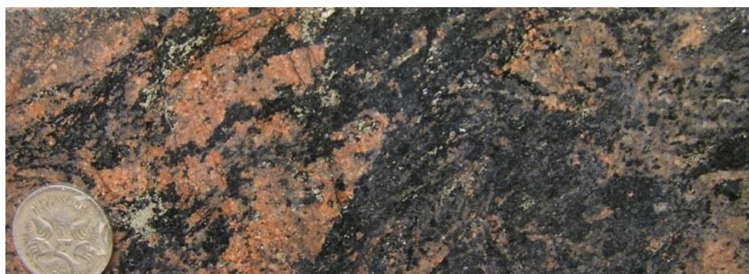
Figure 19: MN14D34 at 64.1m. Magnetite +amphibole +pyrite-rich zone within felsic gneiss
