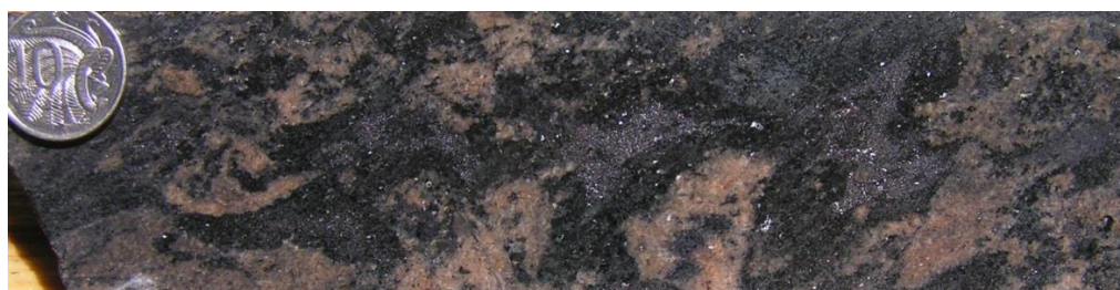
Figure 21: Folded, early-generation magnetite +amphibole band interlayered with felsic gneiss
