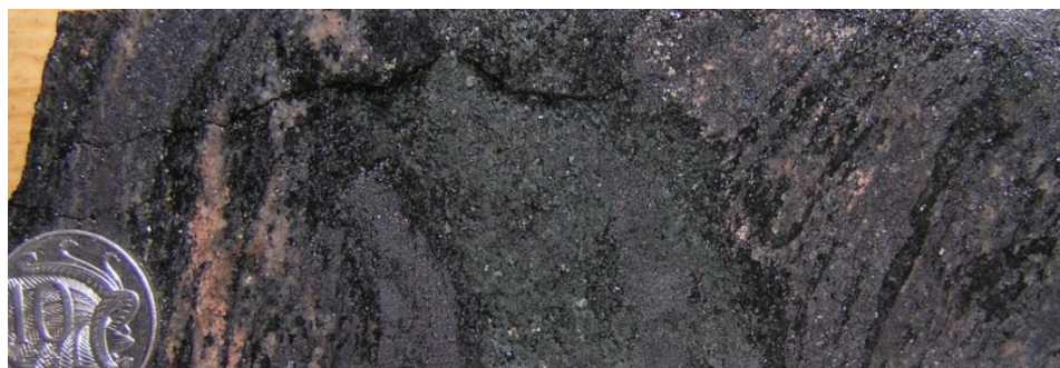
Figure 22: MN14D34 at 101.5m. Magnetite +amphibole vein discordant to foliation within grey felsic gneiss
