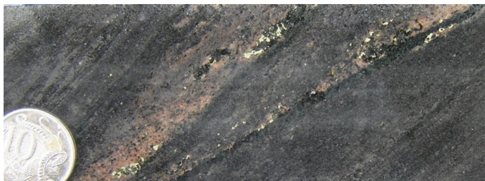
Figure 24: MN14D34 at 176.7m. Thin, late-stage amphibole +chalcopyrite veins within grey quartz +feldspar +biotite gneiss
