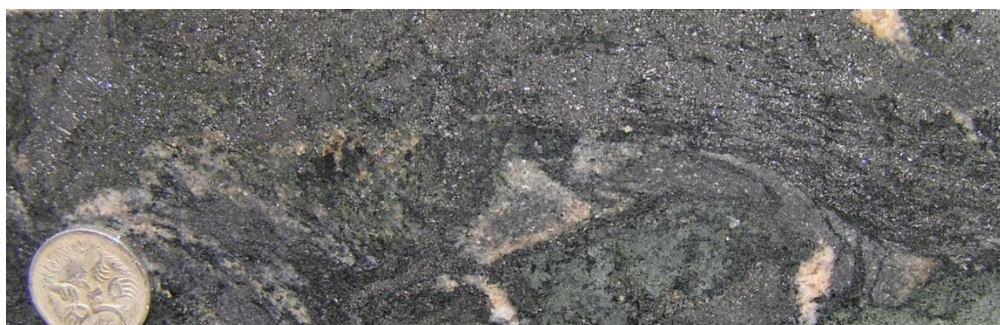
Figure 25: MN14D34 at 223.5m. Magnetite +amphibole-rich alteration zone
