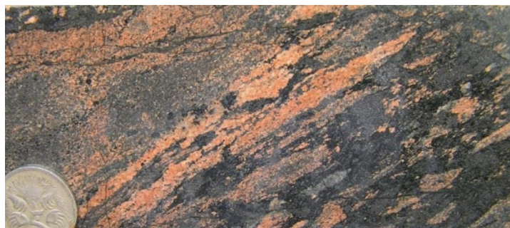
Figure 20: MN14D34 at 69.8m. Magnetite +amphibole +pyrite alteration zone within brecciated felsic gneiss
