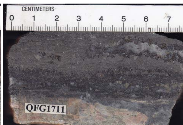
Photograph 129: (left) Gold and base metal (mostly lead and zinc) in a silicified porphyry breccia from Horn Island; (right) massive sphalerite, chalcopyrite and galena bands as vein-infill from Horn Island.
