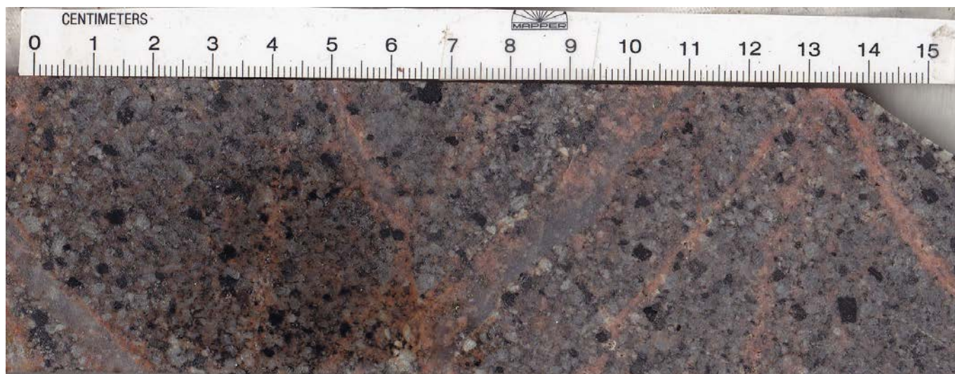
Photograph 67: Biotite porphyry with disseminated copper and molybdenum and fine quartz veinlets in Wingfield Granodiorite of the Rawbelle Batholith, John Hill prospect.
