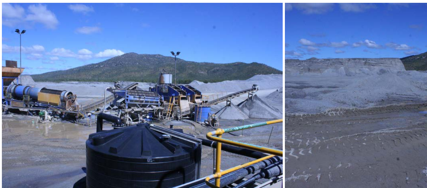
Photograph 184: (left) Mount Carbine tailings retreatment plant; (right) Mount Carbine tailings dam currently being re-worked. Note the fine layering in the material in the background.
