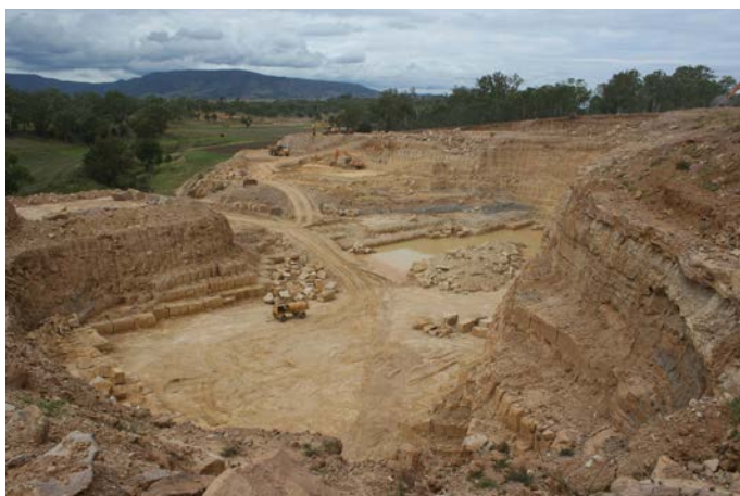
Photograph 215: (a, left) Main working face of the Yangan deposit (Malcolm Guy mine) with at least 8 benches of good quality sandstone blocks cut (b, right) Raw cut sandstone block of typical medium grained pale brown banded sandstone ready for processing.
