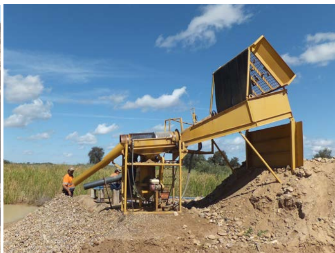
Photograph 205: (left) One of several deep open cuts down to the 'wash' levels of the alluvium at the Australia Mine; (right) mobile alluvial screening plant at Australia Mine.
