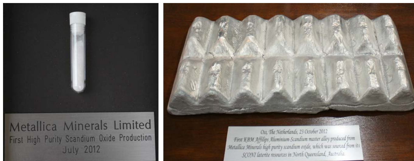
Photograph 170: (Left) First refined high purity scandium oxide production from SCONI project, July 2012, Metallica Minerals Limited. (Right) Aluminium-scandium master alloy, Metallica Minerals Limited 2012.
