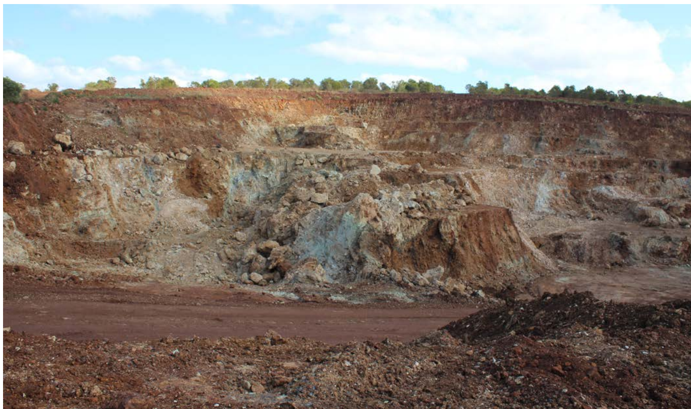
Photograph 164: Profile of Nontronite ore on saprolite and weathered serpentinite basement in pit 2 at the Brolga nickel mine.
