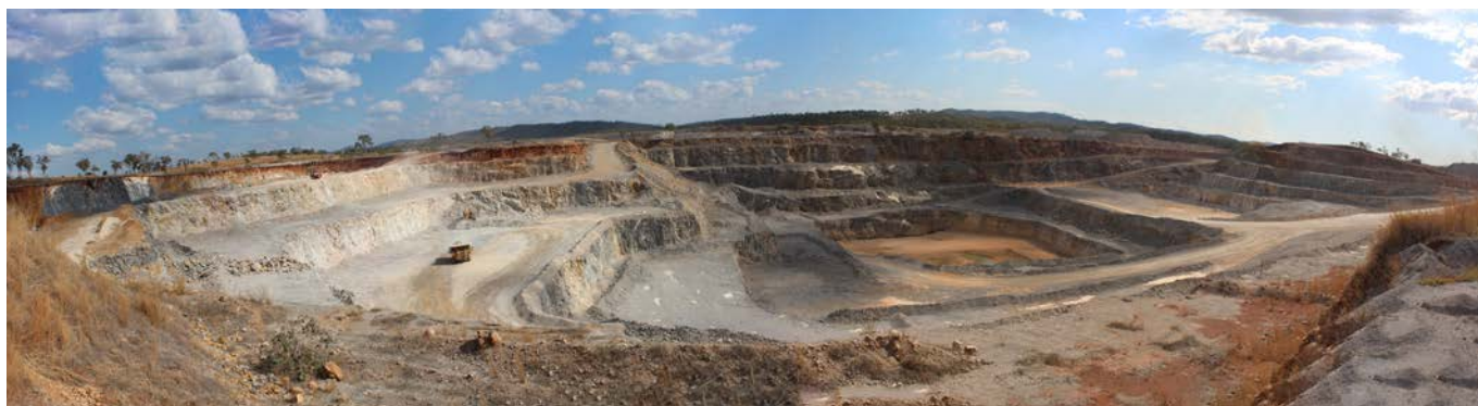
Photograph 260: Taragoolla open cut within highly fractured grey limestone.
