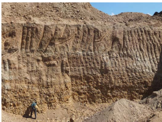
Photograph 205: (left) One of several deep open cuts down to the 'wash' levels of the alluvium at the Australia Mine; (right) mobile alluvial screening plant at Australia Mine.
