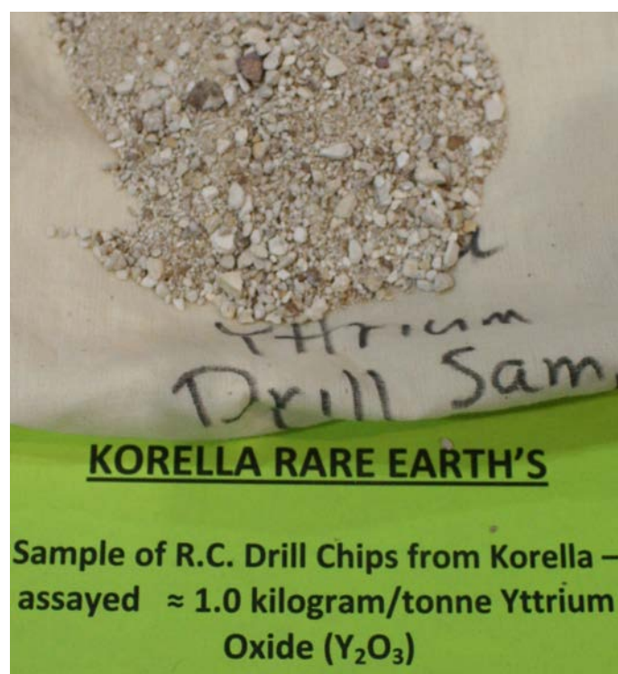
Photograph 195: R.C. drill chips of yttrium mineralisation contained in the mineral xenotime from the Korella Rare Earths prospect.
