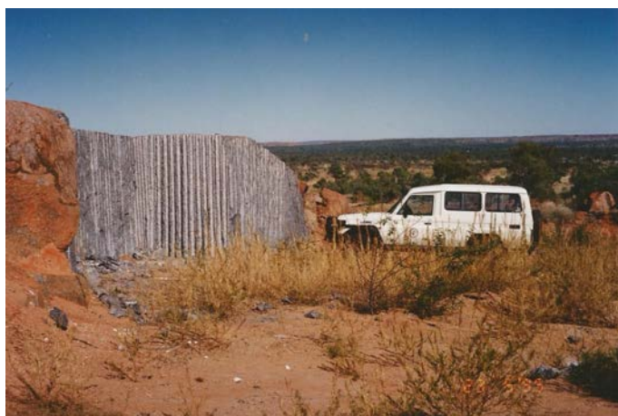
Photograph 235: (left) Freshly drilled rock face at Mount Guide Holding Sybella granite quarry in 1995; (right) Close-up of drilling rock block of Sybella granite (images courtesy David Trezise).
