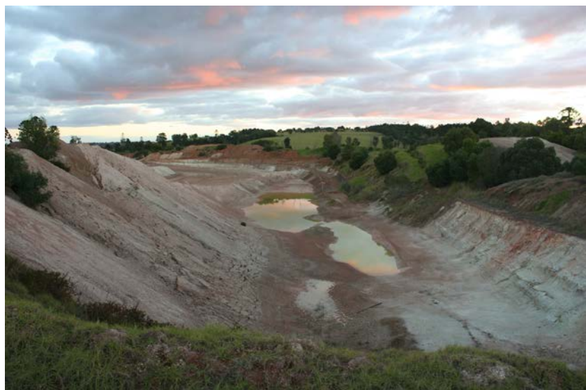
Photograph 243: Cedars mine open cut, source of sodium bentonite from flat-lying altered volcanic sediments formed in a lacustrine environment.
