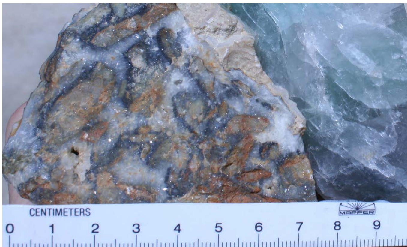
Photograph 130: Welcome Siliceous Breccia with tin-quartz-fluorite mineralisation from Horn Island.
