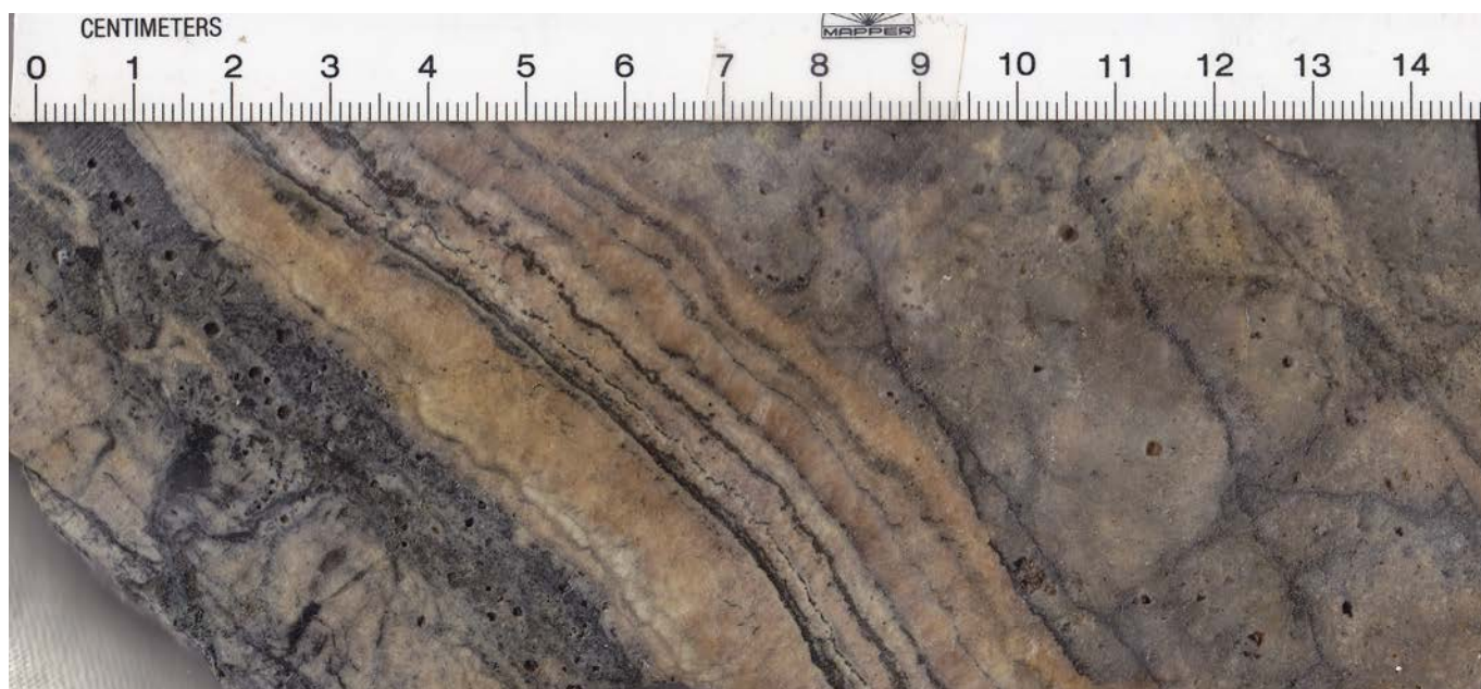
Photograph 97: Banded open space fill alunite-sphalerite-pyrite-enargite veins from V2, within the Mount Carlton Project.
