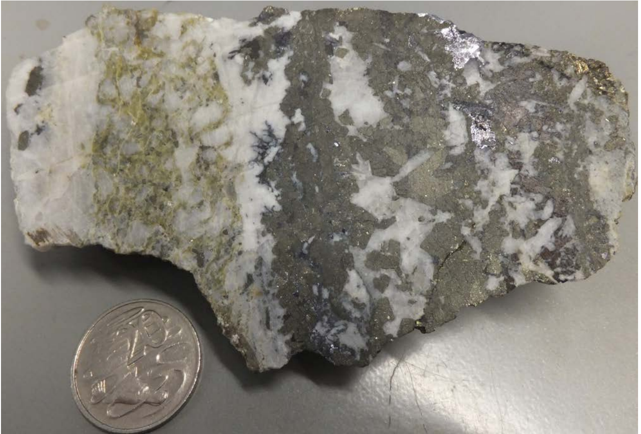
Photograph 108: Intrusive auriferous chalcopyrite-pyrite quartz vein mineralisation from Charters Towers (sample from GSQ's historical collection, image courtesy Paul Blake, GSQ).
