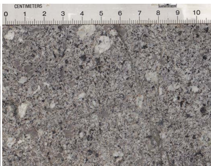
Photograph 237: (a) Medium-grained equigranular pink biotite granite associated with the main body of the Stanthorpe Granite batholith; (b) Fine-grained porphyritic biotite granite with large euhedral feldspar and quartz phenocrysts, highly silicified, also associated with the Stanthorpe Granite.
