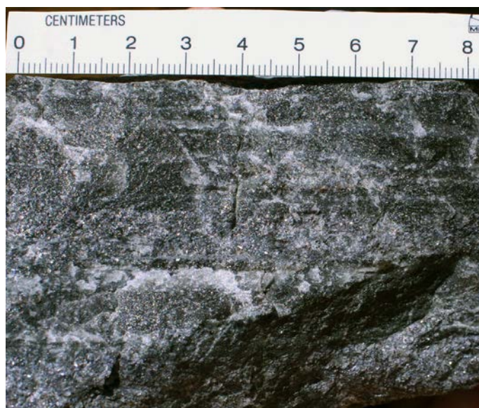
Photograph 83: Stratiform lead and zinc mineralisation from Cannington underground mine.
