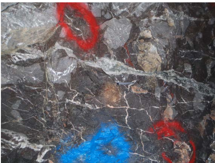
Photograph 136: Mineralised vein breccia and silicified volcanic rock at Roses Pride underground mine, Cracow.
