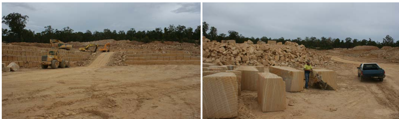
Photograph 217: (a) Main open cut within the Tanamerah sandstone deposit in 2014. (b) Banded pale brown sandstone blocks ready for processing at the Tanamerah deposit.
