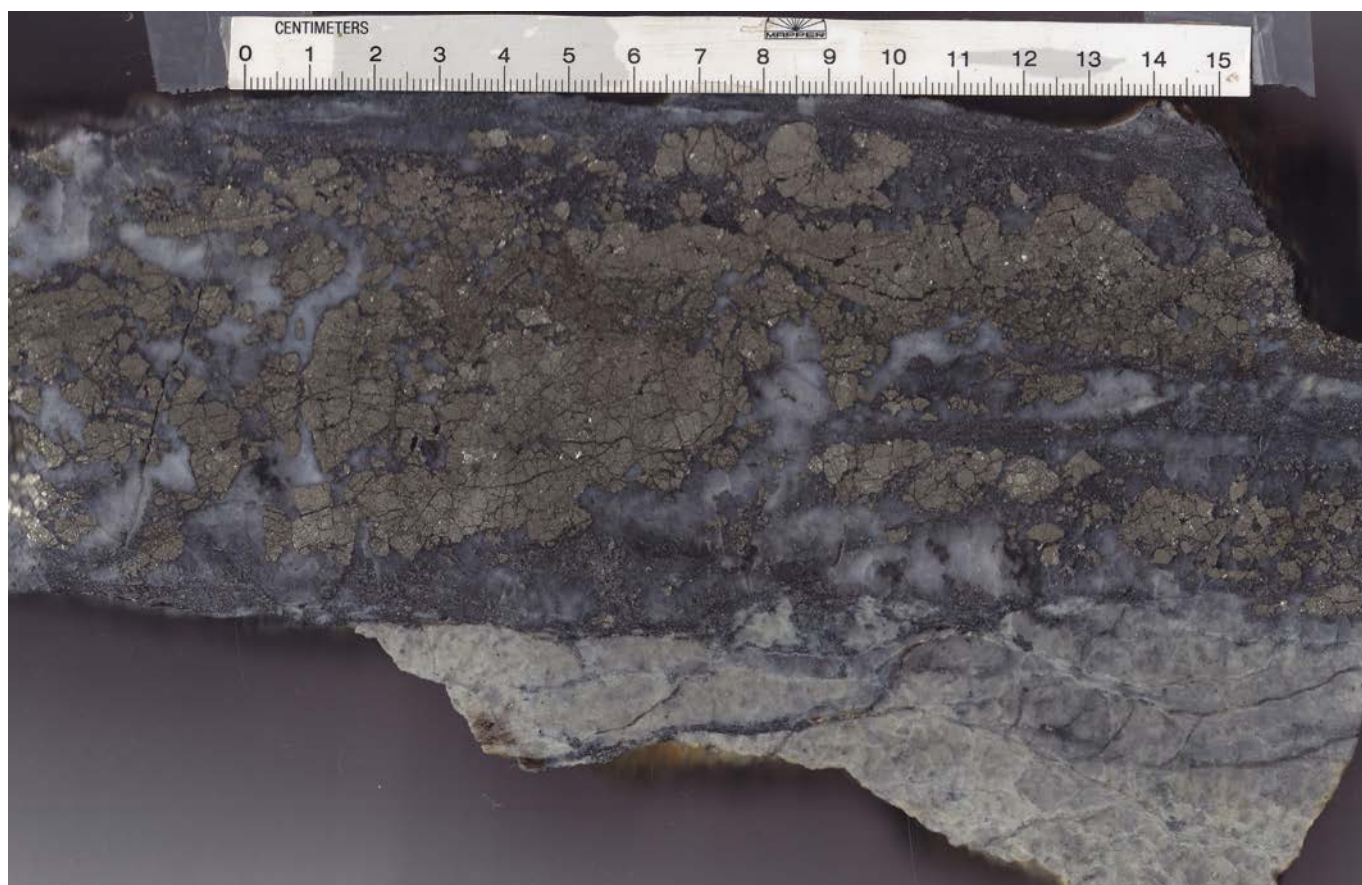
Photograph 122: Sulphide mineralisation (arsenopyrite–chalcopyrite with gold) within shear zone at the Frampton deposit, Norton Goldfield.
