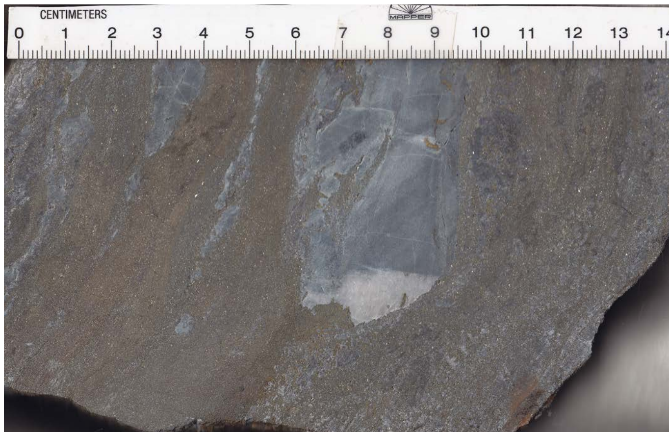
Photograph 56: Massive sulphide (pyrite, chalcopyrite) mineralisation from Highway-Reward mine.
