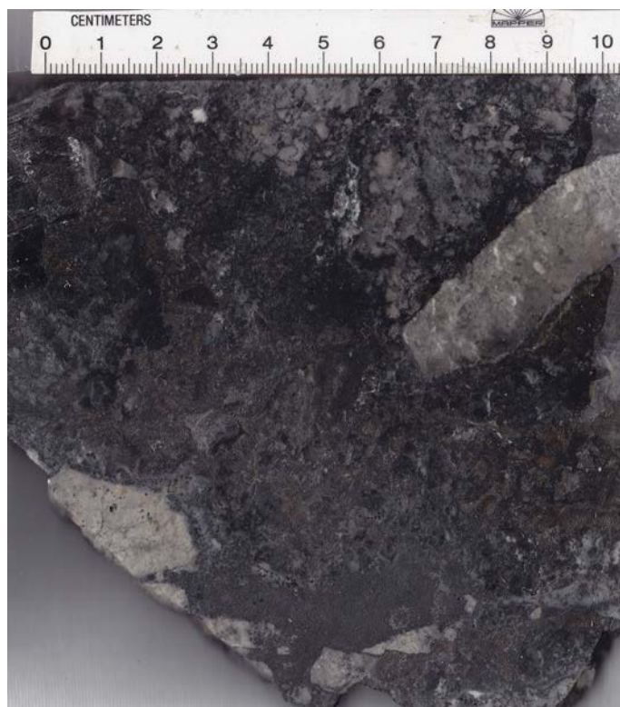
Photograph 241: Light grey barite in breccia from within the high-grade silver resource from the bottom of the A39 open cut at Mount Carlton silver–gold mine.
