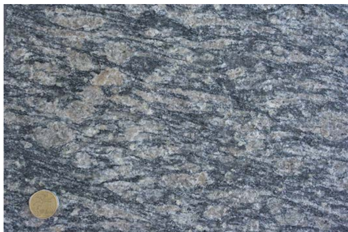
Photograph 236: (a) Coarse-grained, porphyritic or porphyroblastic augen gneiss ('granite'), set in a strongly foliated biotite rich groundmass; (b) Sybella granite pavers placed in the Queen Street Mall in Brisbane in 2000 by J.H. Wagner and Sons Pty Limited (Photo taken in 2015).
