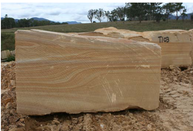
Photograph 215: (a, left) Main working face of the Yangan deposit (Malcolm Guy mine) with at least 8 benches of good quality sandstone blocks cut (b, right) Raw cut sandstone block of typical medium grained pale brown banded sandstone ready for processing.
