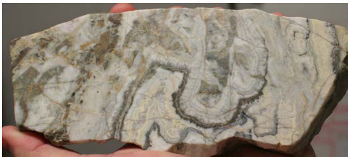
Photograph 135: (above) Auriferous colliform quartz veining and brecciation, Cracow Gold mine; (right) auriferous quartz veining with adularia alteration, GoldenPlateau open cut, Cracow Gold mine.
