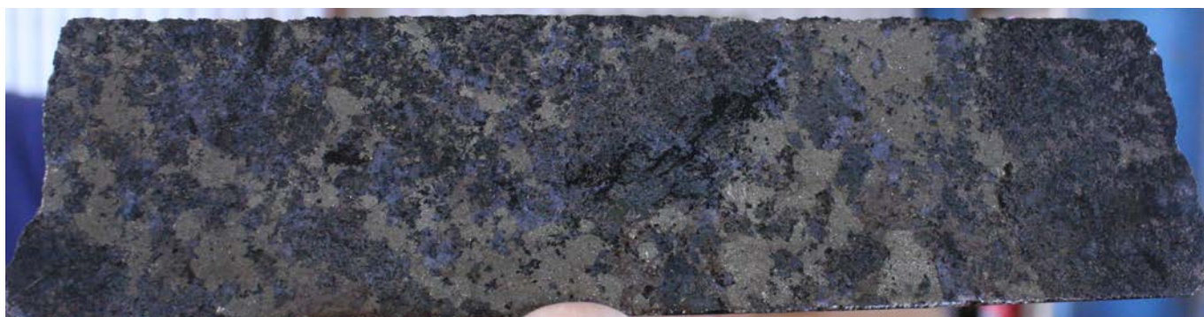
Photograph 193: Drill core from Elaine Dorothy in coarse-grained massive sulphides in pyroxenite with an extremely high radioactive response (uranium mineralisation present).
