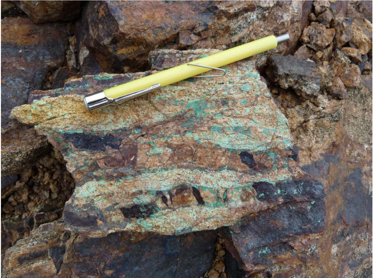
Photograph 62: Copper mineralised vein system from the Kiwi Prospect at Boobyjan (image courtesy Doug Young, ActivEx).
