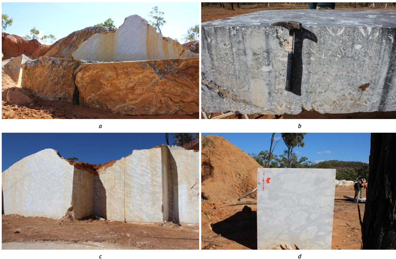
Photograph 224: (a) The black fossiliferous limestone quarry (Federation Stone quarry) at Chinaman Creek, south of Greenvale; (b) The limestone contains abundant white fossil bivalves, corals, sponges and brachiopods, including shells of giant megalodont clams; (c) White marble breccia with a distinct orientation of breccia clasts is produced from the 'White quarry' at Chinaman Creek by NQ Marble; (d) One block of white marble breccia from the 'White quarry', stamped by NQ Marble, ready for export.
