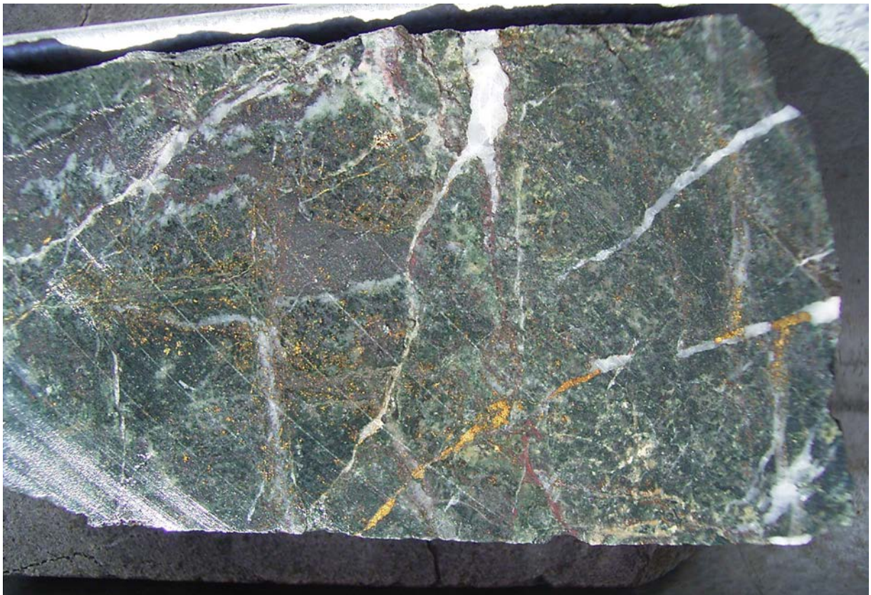
Photograph 63: Copper mineralisation in drill core (KAKD1, 98m) from the Kiwi Prospect, Boobyjan (image courtesy Doug Young, ActivEx).
