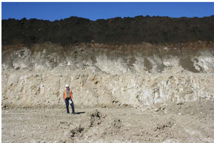
Photograph 267: Light-coloured magnesite nodular horizon under black clay-soil overburden at Pit 23, Kunwarara Magnesite mine.
