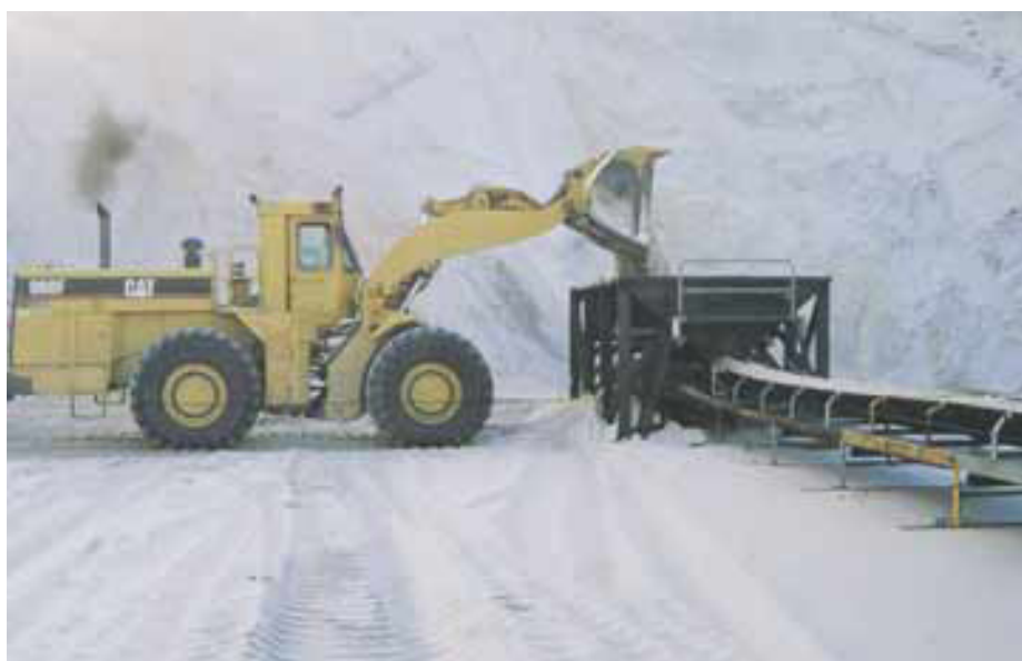
Photograph 280: Bulk loading of silica sand in conveyor belt to the wharf at Cape Flattery (image courtesy DNR, Queensland Mineral and Petroleum Review, 2002).
