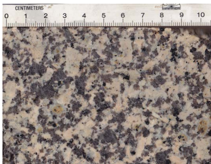
Photograph 237: (a) Medium-grained equigranular pink biotite granite associated with the main body of the Stanthorpe Granite batholith; (b) Fine-grained porphyritic biotite granite with large euhedral feldspar and quartz phenocrysts, highly silicified, also associated with the Stanthorpe Granite.
