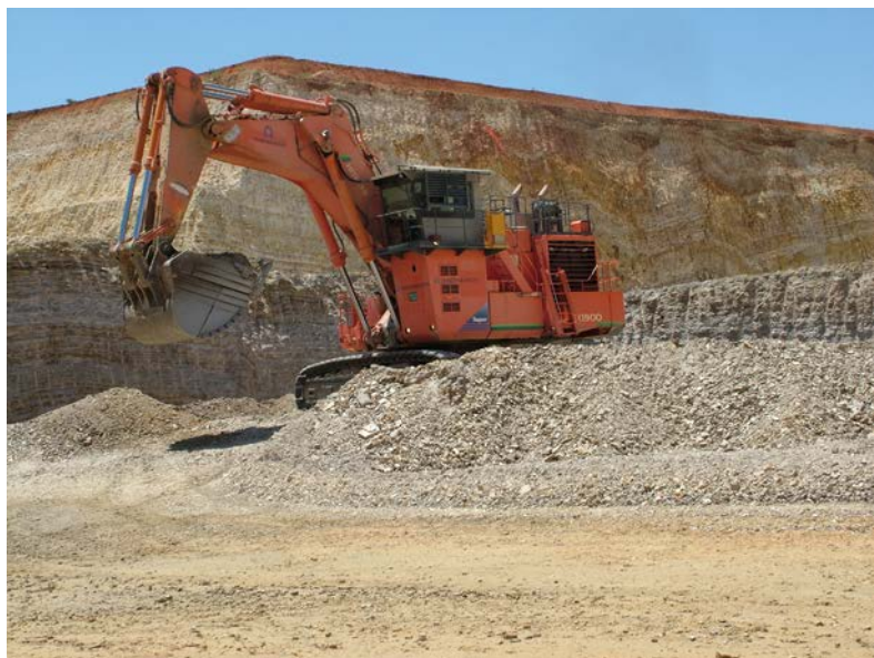
Photograph 276: Mining phosphate rock from flat-lying phosphatic siltstone within the Beetle Creek Formation at Phosphate Hill (image courtesy David Carmichael, 2007, DNRM).
