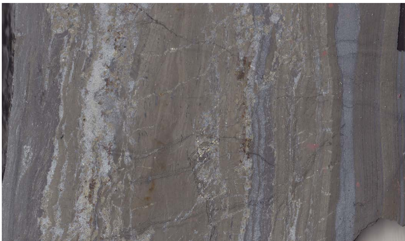
Photograph 77: Banded sphalerite and galena mineralisation in metasediments from George Fischer mine.
