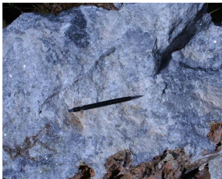
Photograph 291: The pen marks area in photograph showing wollastonite mineralisation in Chillagoe marble from the Wollastonite pit, owned by Chillagoe Marble Australia Pty Limited.
