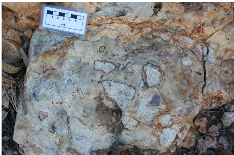
Photograph 138: Siliceous epithermal breccia in Robin Hood Granodiorite near Sherwood, Agate Creek Project.
