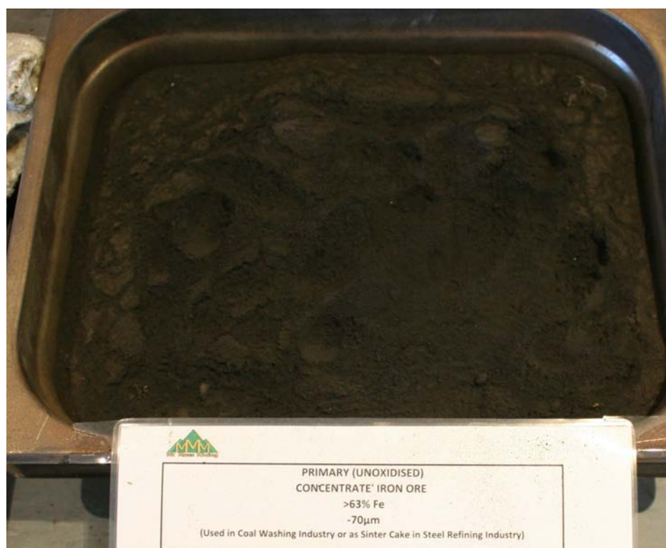
Photograph 150: Primary (unoxidised) iron ore concentrate at -70µm (>63% Fe) produced at Mount Moss, (this product is used in the coal washing industry or as sinter cake in the steel refining industry).
