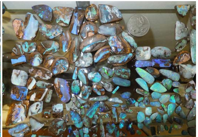
Photograph 202: Numerous examples of polished boulder opal displaying some ironstone rock along margins (samples from GSQ's historical collection, image courtesy Paul Blake, GSQ).
