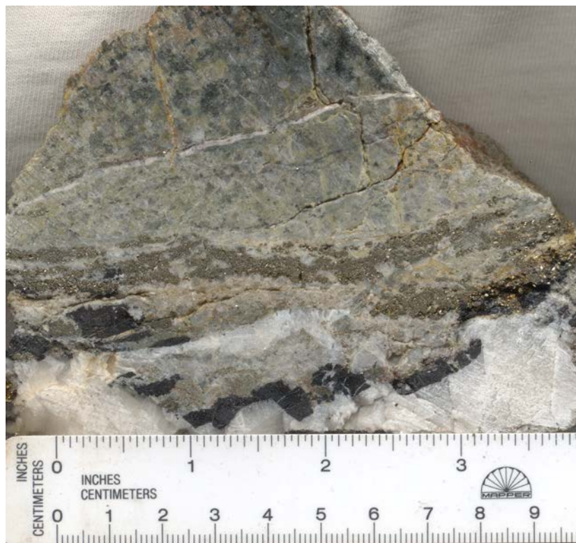
Photograph 115: Intrusion-related breccia, with infilled sulphides into granite, from Mount Leyshon.
