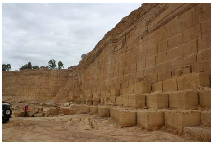
Photograph 215: (a, left) Main working face of the Yangan deposit (Malcolm Guy mine) with at least 8 benches of good quality sandstone blocks cut (b, right) Raw cut sandstone block of typical medium grained pale brown banded sandstone ready for processing.
