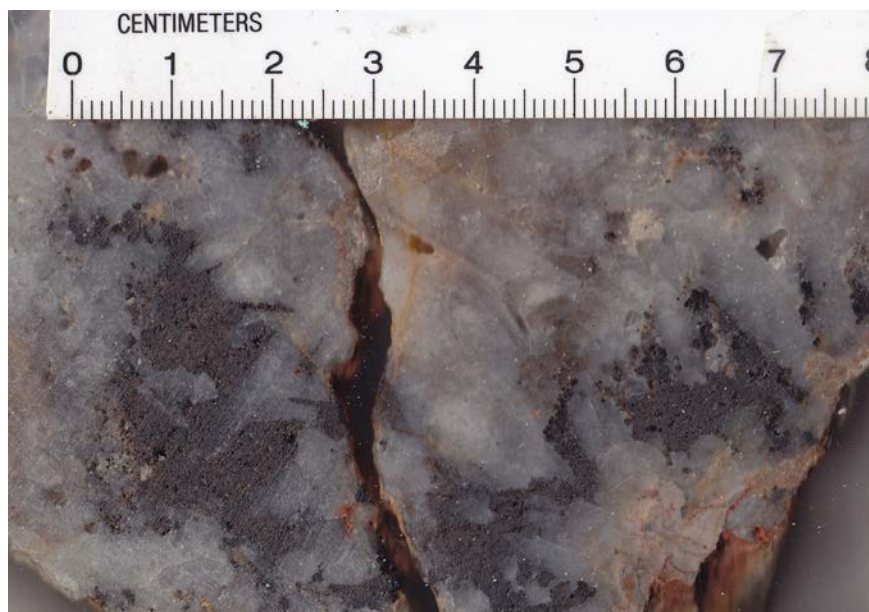
Photograph 175: Cassiterite quartz vein mineralisation at Dalcouth prospect.
