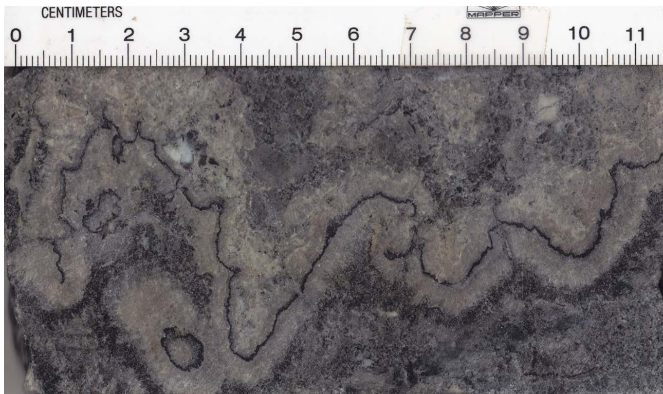
Photograph 98: Banded to colliform acanthite (silver sulphide) and stromeyerite (silver copper sulphide) in quartz-kaolin-dickite altered epiclastic to volcanoclastic sediments from A39, within the Mount Carlton Project
