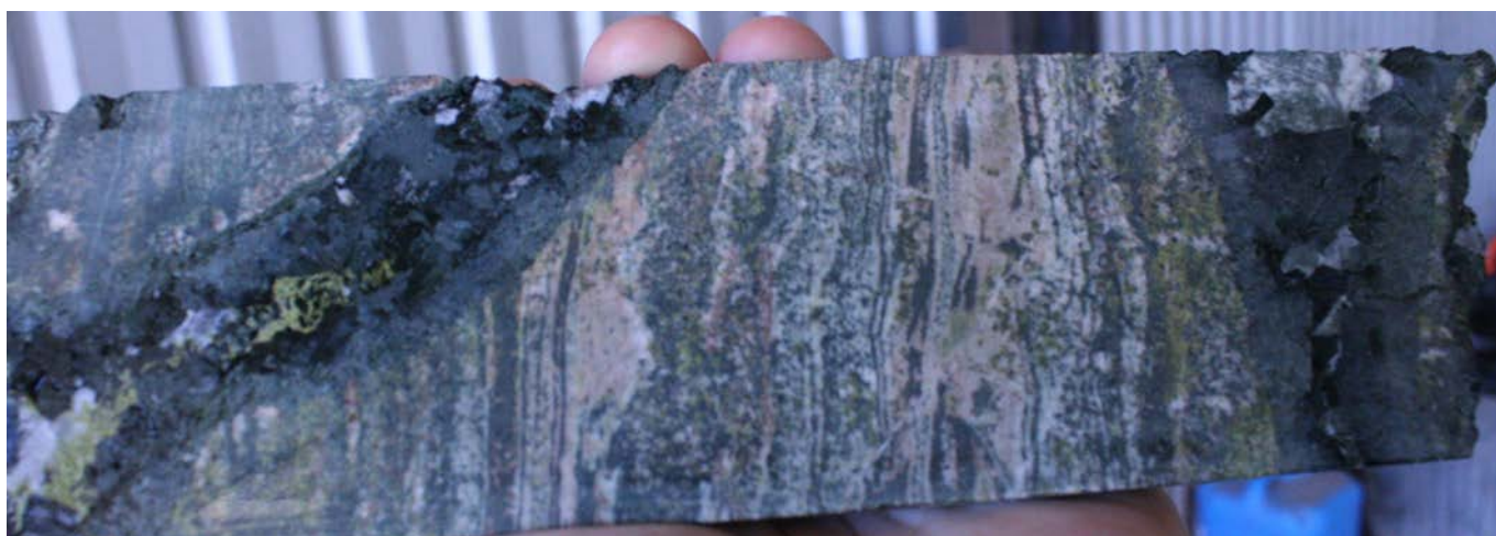
Photograph 55: Drill core from Elaine Dorothy; Well-banded calc-silicate with chalcopyrite vein mineralisation.
