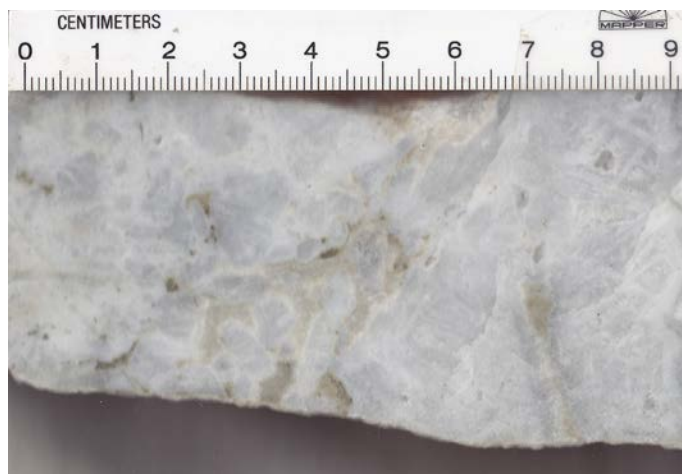
Photograph 132: (left) Epithermal quartz veins from Pajingo; (right) mineralised sheared fault in Vera Nancy (Pajingo) open cut (image courtesy Vladimir Lisitsin, GSQ).
