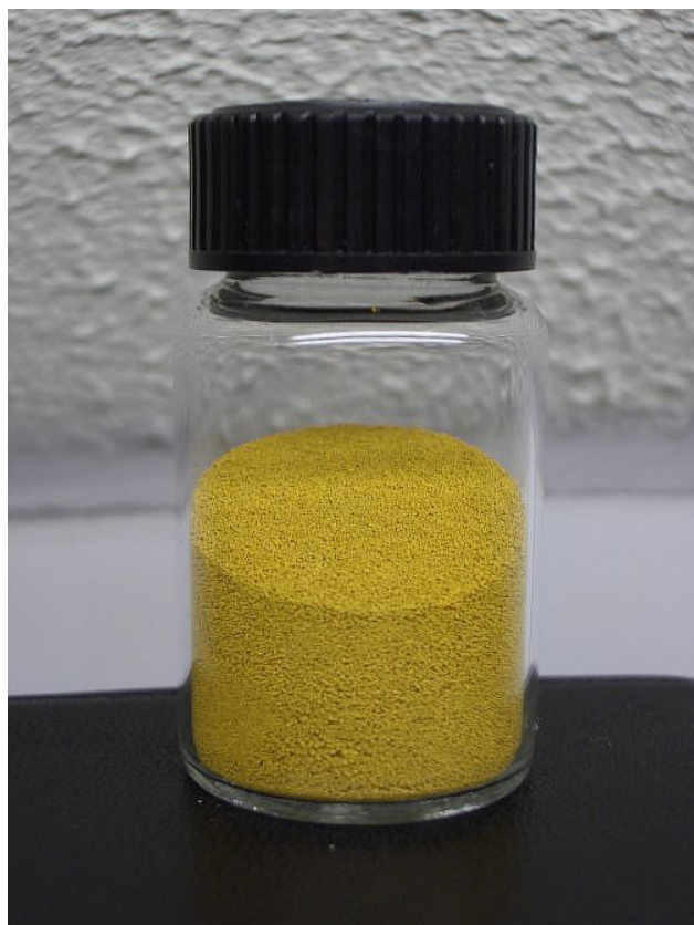
Photograph 194: Divanadium pentoxide ( V_2O_5 ) is an inorganic compound precipitated from aqueous solution. This compound of vanadium is the principal precursor to alloys of vanadium and is a widely used industrial catalyst (image courtesy of W. Oelen, Wiki Commons).
