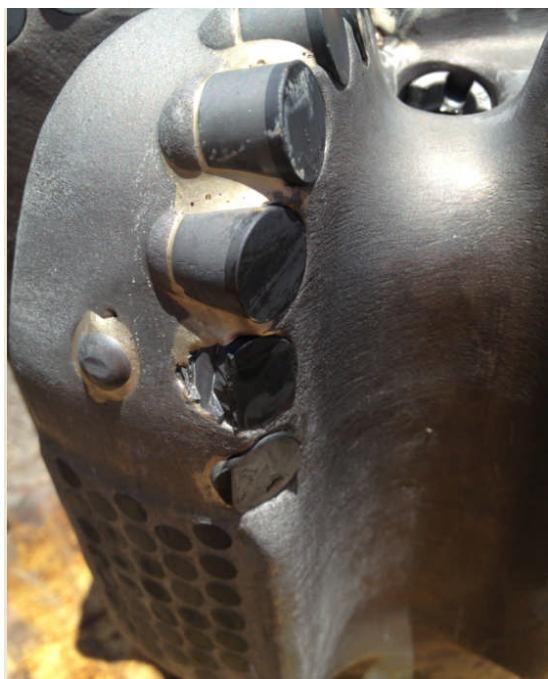
Blade-1: broken Teeth in shoulder, minor ovoid wear.
