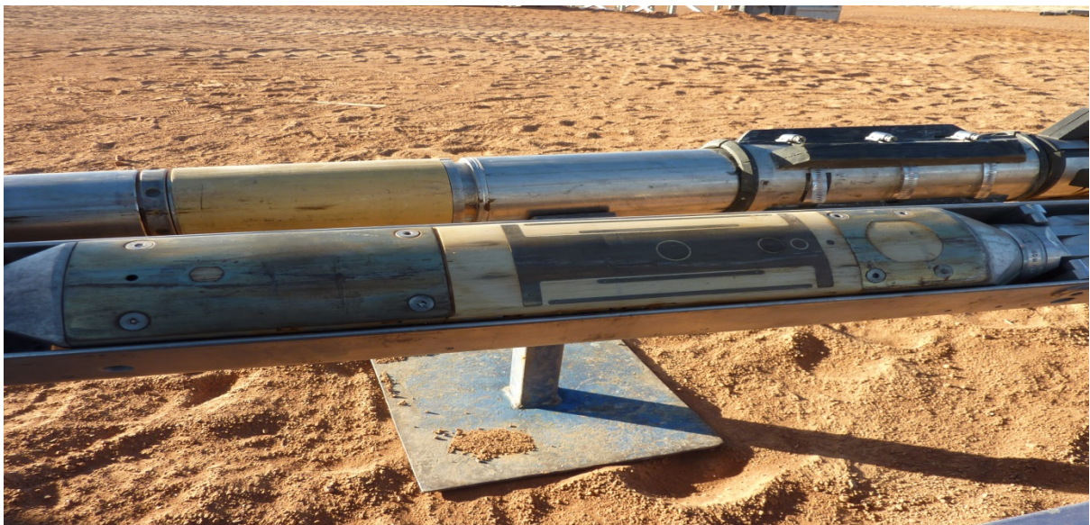
Figure-2 Showing MCFL buttons situated in between the TLD detectors.
