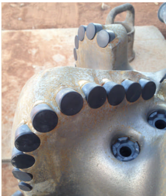
Green cutters and evidence of minor tiger stripe/matrix erosion.
