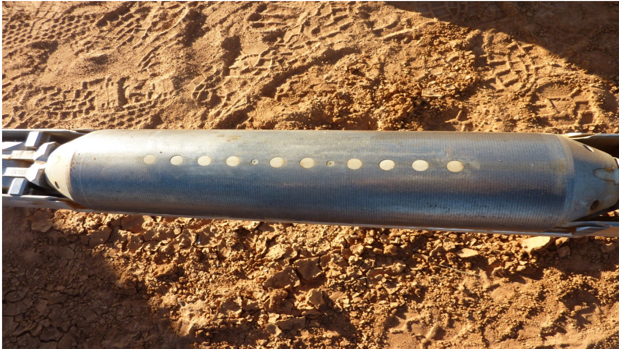
Figure 4- ADT top and lower Transmitters (in the middle) and 4 set-Top and Bottom receivers
