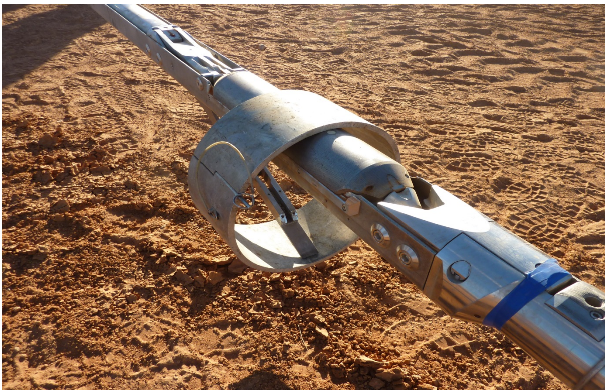
Figure 4- ADT caliper and large caliper ring used to calibrate the caliper section.
