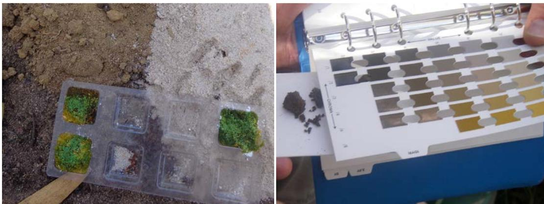
Figure 6: Field pH testing and soil colour recording. Left: Field pH test using the CSIRO Inuculo™ pH testing kit to establish soil acidity. Right: Recording the wet and dry soil colour using the Munsell soil-colour charts.
