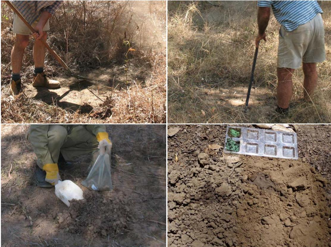
Figure 4: Sampling TOS. (From top left): A. Clearing surface organic matter and vegetation using a shovel, B. Loosening and homogenising soil to 10 cm depth with a steel crowbar, C. Thoroughly compositing soil and transferring TOS sediments with a clean white plastic scoop into pre-labelled polythene bag, D. Field tests including pH test, acid test, recording wet and dry soil colour and lithologic logging.
