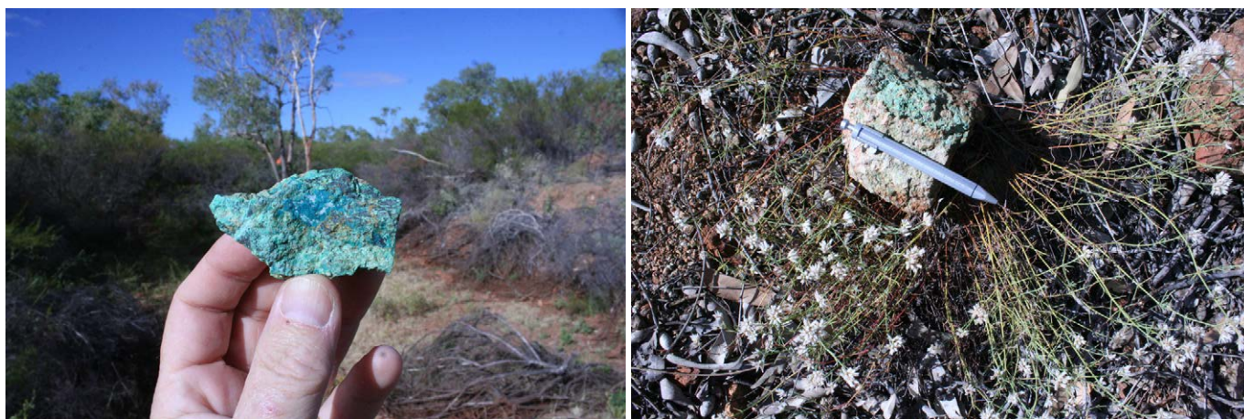
Photograph 49: Copper mineralisation at the Little Eva prospect. (Note sample in right hand photograph, placed on outcrop expression identified by presence of Copper Bush plant).
