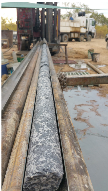
Photograph 251: Recovery of Metallica drill core (WD002) from the Esmeralda Graphite Project at drill site. Darker enclaves within the Esmeralda Granite contain graphite (image courtesy Metallica Minerals Limited).
