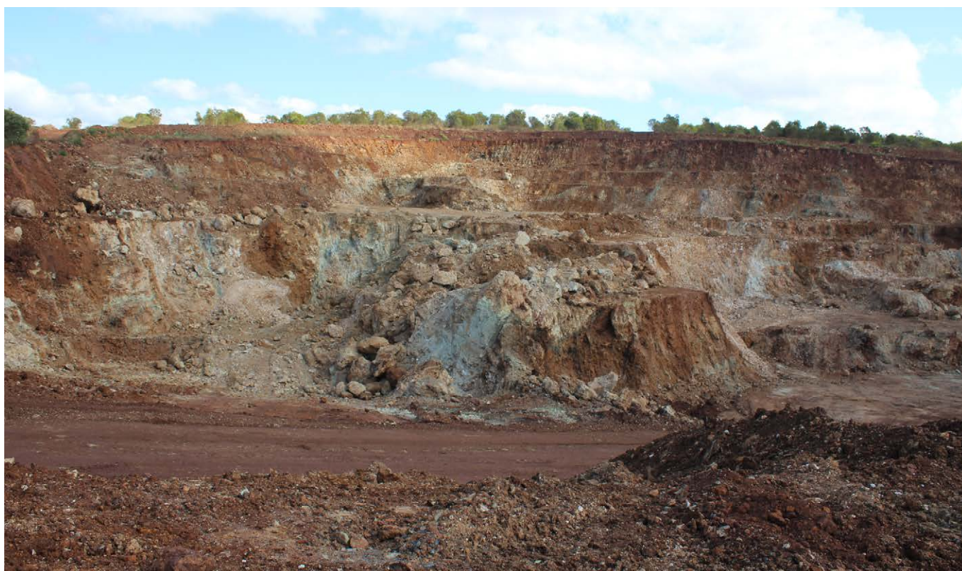
Photograph 164: Profile of Nontronite ore on sapprolite and weathered serpentinite basement in pit 2 at the Brolga nickel mine.
