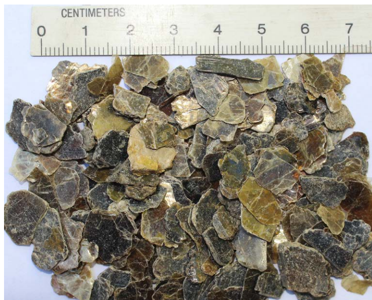
Photograph 290: Olive-brown vermiculite flakes (imported from the Phalaborwa deposit in South Africa).
