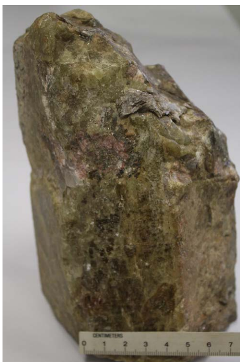
Photograph 207: Crystalline beryl with impurities from pegmatite within the Mica Creek deposits (assumed to come from Big Beryl deposit). Historical specimen in the GSQ Collection.
