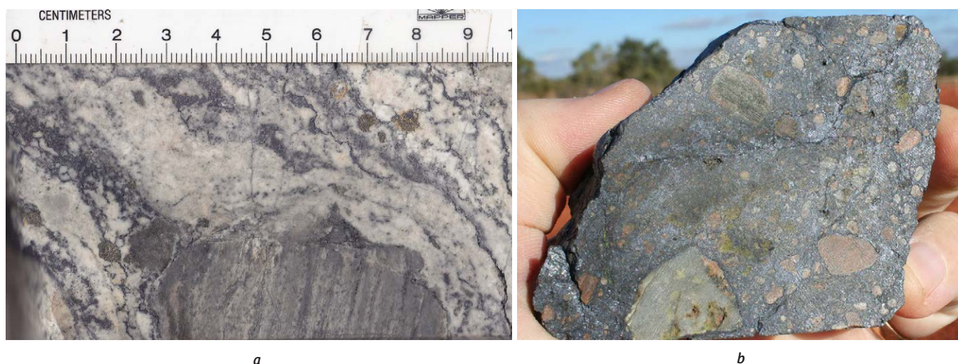
Photograph 159: (Left, a) Fault breccia infill in highly altered metasediments with molybdenite and rhenium mineralisation from the Merlin deposit. (Right, b) Matrix-supported ore breccia with molybdenite and rhenium mineralisation as matrix infill and silicified sub-rounded metasediment clasts (between 0.2 and 1.5 cm) from drill hole MDQ0404 at 410 m depth within the Merlin deposit.
