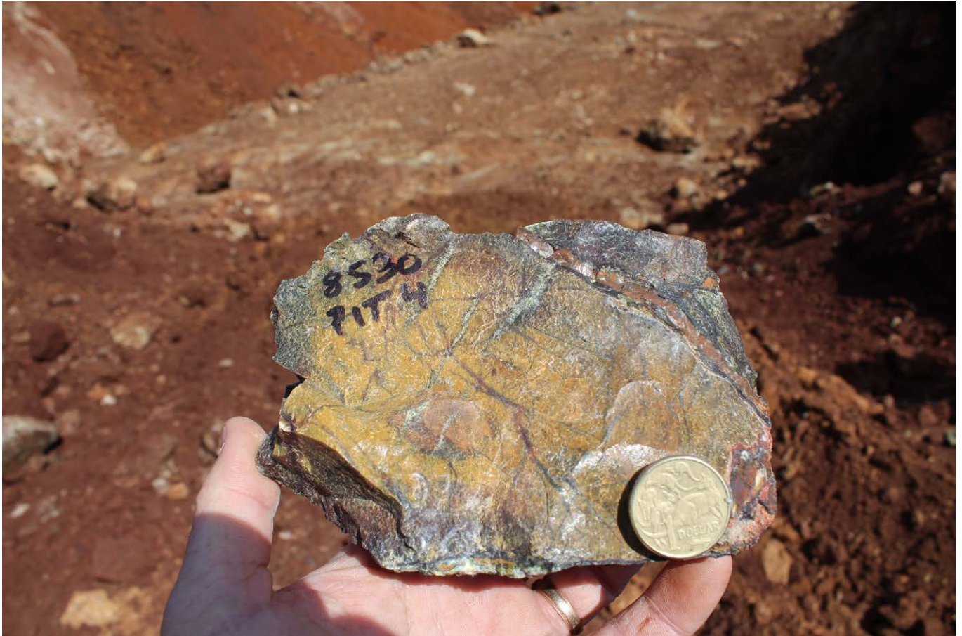
Photograph 165: Enriched weathered serpentinite with approximately 1.6–1.8% Ni (hand-held XRF readings) from pit 4 at the Brolga nickel mine.
