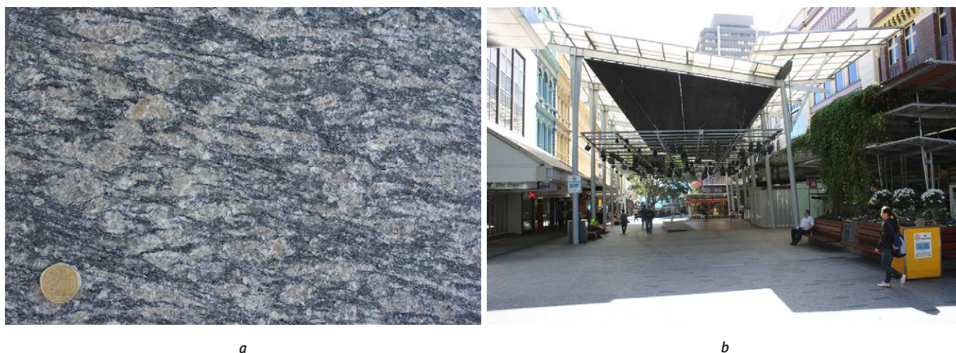
Photograph 236: (a) Coarse-grained, porphyritic or porphyroblastic augen gneiss ('granite'), set in a strongly foliated biotite rich groundmass; (b) Sybella granite pavers placed in the Queen Street Mall in Brisbane in 2000 by J.H. Wagner and Sons Pty Limited (Photo taken in 2015).
