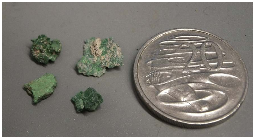
Photograph 191: Secondary torbernite crystals from the Milo project.
