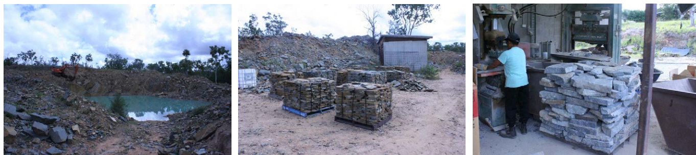
Photograph 227: (a) Australian Porphyry's Rogina deposit featuring the brown and greenish-grey rhyolite porphyry with its favourable slaty break, facilitating a pre-sorting of saleable stone at the deposit; (b) Pre-packed porphyry stone slabs ready for shipment from the quarry; (c) Optional pressure cutting of porphyry slabs to blocks, pavers and cobbles on a mechanical guillotine is done at Australian Porphyry's Herberton factory.
