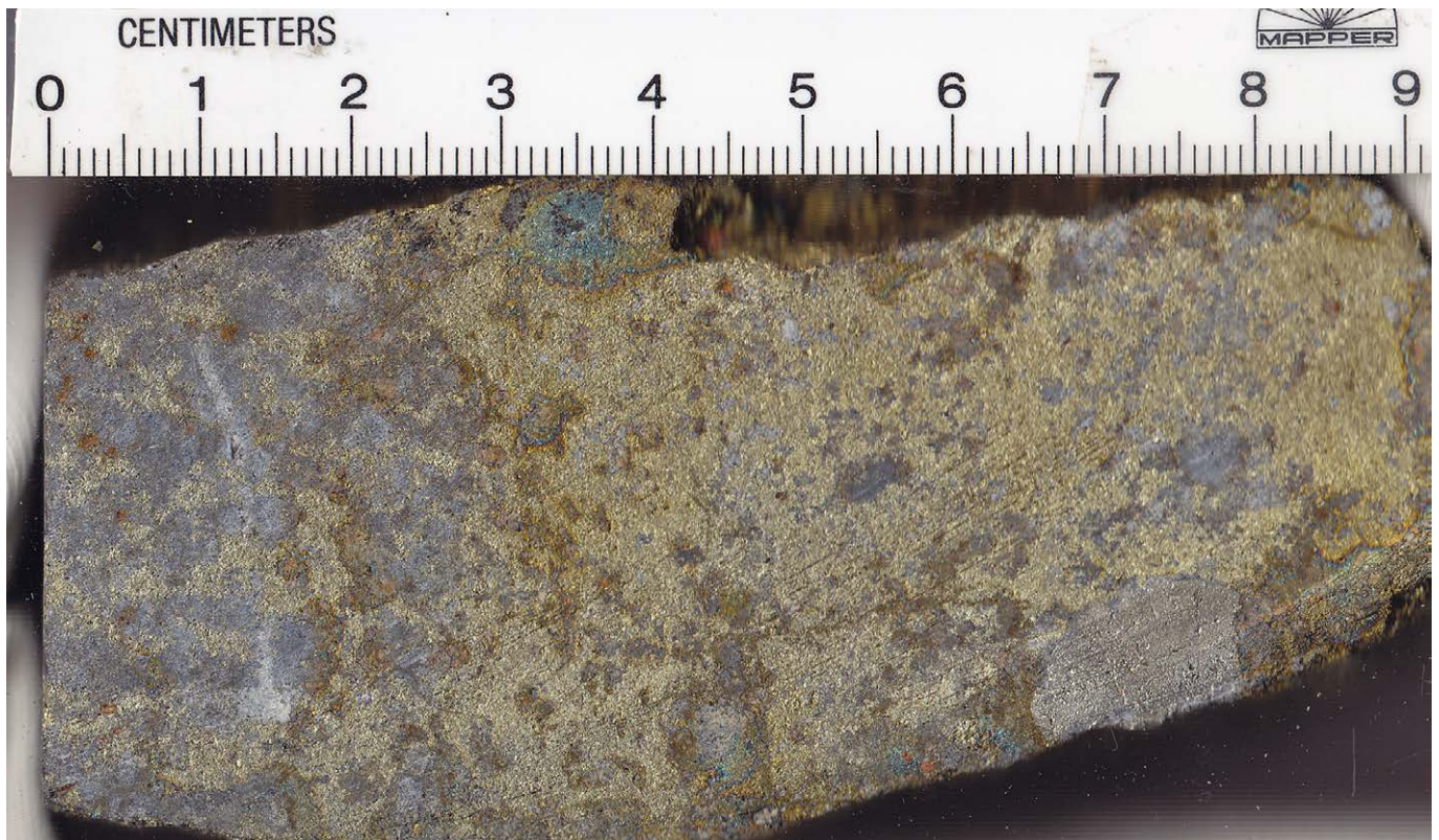
Photograph 22: Massive copper mineralisation (mostly chalcopyrite) from the 3000 ore body at Mount Isa Copper Mine.
