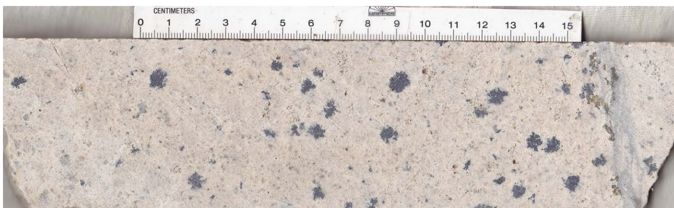
Photograph 66: Porphyry with molybdenum rosettes and some chalcopyrite within the Wingfield Granodiorite of the Rawbelle Batholith, Gordons prospect, Whitewash Project.
