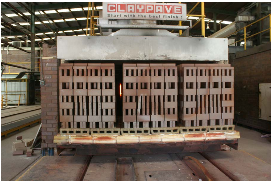
Photograph 285: Clay pavers stacked loosely for firing in Kiln train at Claypave's Dinmore plant
