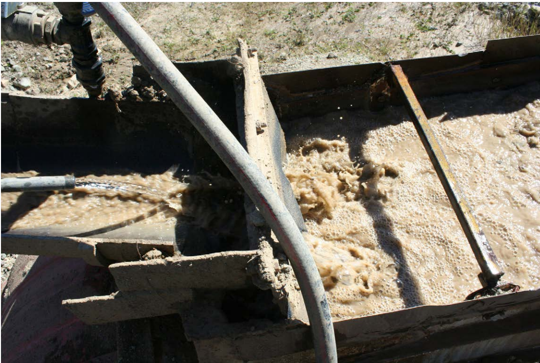
Photograph 148: Sluice box with carbon matt for collecting fine alluvial gold from gravel at the Prophet Gold Mine, Kilkivan.
