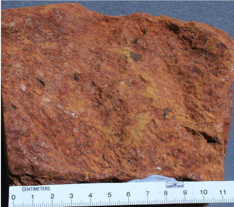
Photograph 166: Lateritic nickel ore from the Greenvale Nickel mine open cut.
