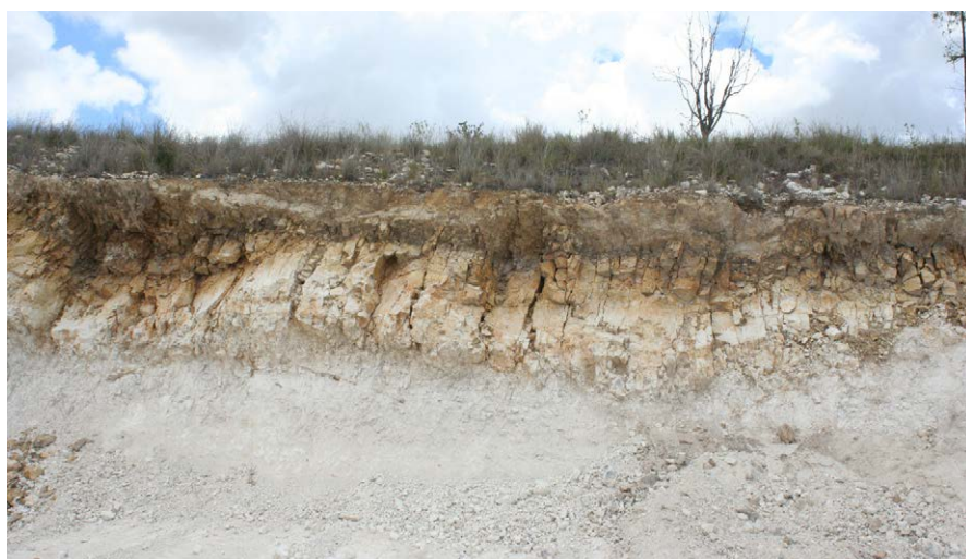
Photograph 269: A white palygorskite clay is overlain by dolomite in the open cut on the Wadley Lease on the Flinders Dolomite Ridge.
