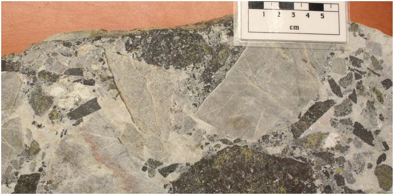
Photograph 91: Skarn breccia with zinc-rich polymetallic mineralisation from Mungana mine.
