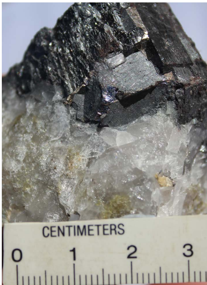
Photograph 101: Wolframite and bismuth, together with minor chalcopyrite and molybdenite, are intergrown within a pipe quartz, collected from the base of the Wolfram Camp mine open cut in 2015.
