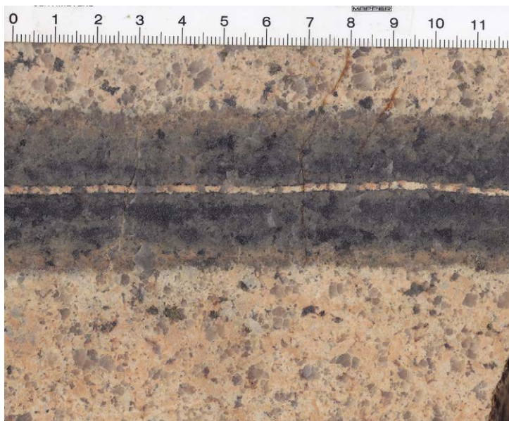
Photograph 171: Tin vein (Cornish style) mineralisation in granite from New St Patrick mine, near Herberton.
