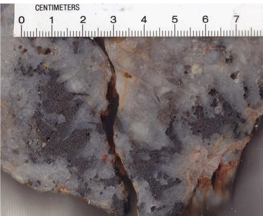
Photograph 175: Cassiterite quartz vein mineralisation at Dalcouth prospect.
