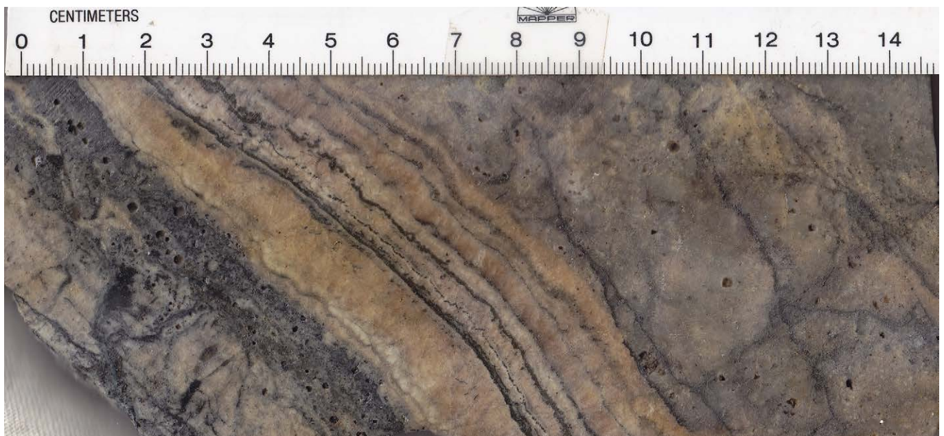
Photograph 97: Banded open space fill alunite-sphalerite-pyrite-engargite veins from V2, within the Mount Carlton Project.
