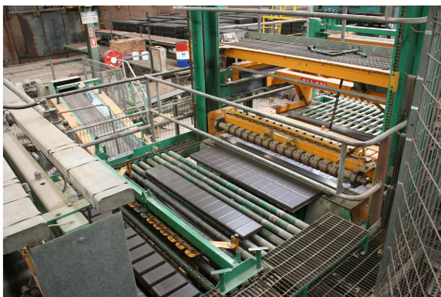
Photograph 283: Automated cutting of clay pavers prior to kiln firing at Claypave's Dinmore plant
