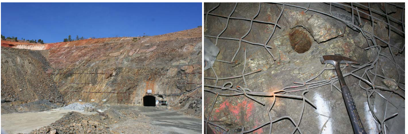
Photograph 60: (left) Balcooma copper underground portal; (right) Balcooma underground massive copper mineralisation (mostly chalcopyrite).
