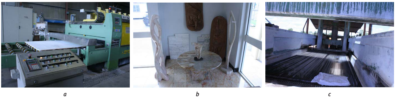
Photograph 219: (a) Automated slab polisher at Cairns Marble & Granite's workshop (=trade name for Cairns Marble Australia Pty Limited); (b) showroom at Cairns Marble & Granite displaying tiles, furniture and sculptures made of Chillagoe marble; (c) slab cutting box at Cairns Marble Australia Pty Limited's Chillagoe processing facility.
