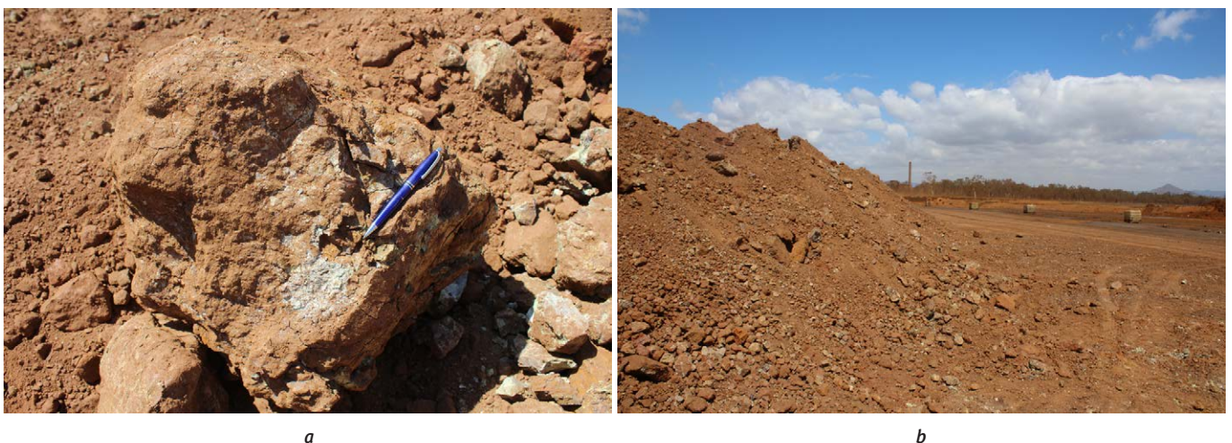
Photograph 167: (left) Lateritic nickel ore from Dingo Dam; (right) Nickel ore stockpile from Dingo Dam awaiting processing at the Palmer Nickel and Cobalt refinery in August 2015.
