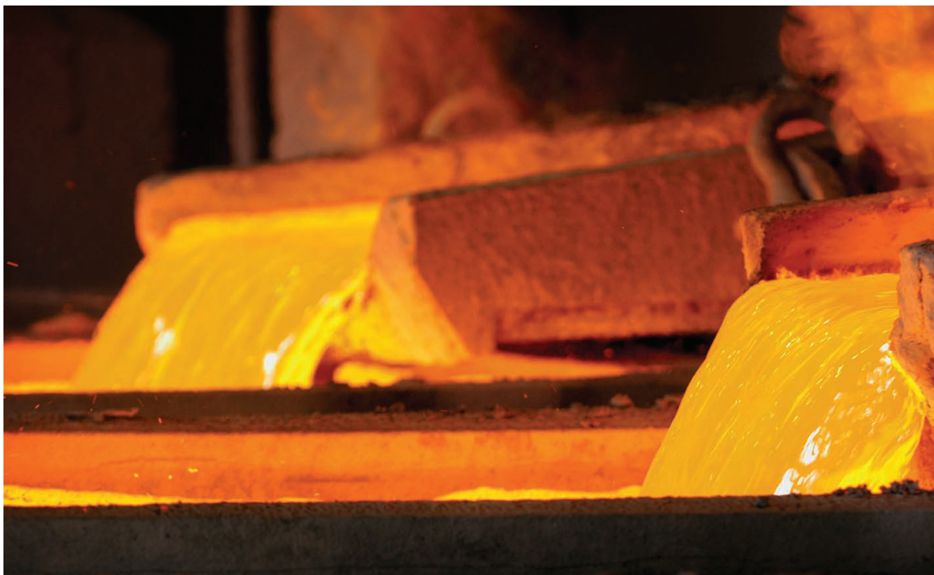
Photograph 12: Mount Isa copper anode wheel at the copper smelter (image courtesy Xstrata Copper; Queensland mining and petroleum 2005).
