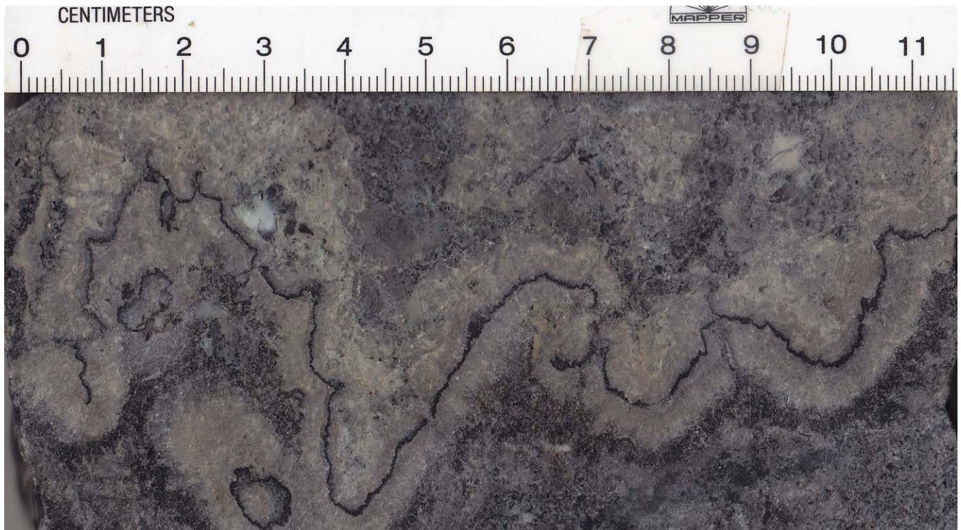
Photograph 98: Banded to colliform acanthite (silver sulphide) and stromeyerite (silver copper sulphide) in quartz-kaolin-dickite altered epiclastic to volcanoclastic sediments from A39, within the Mount Carlton Project
