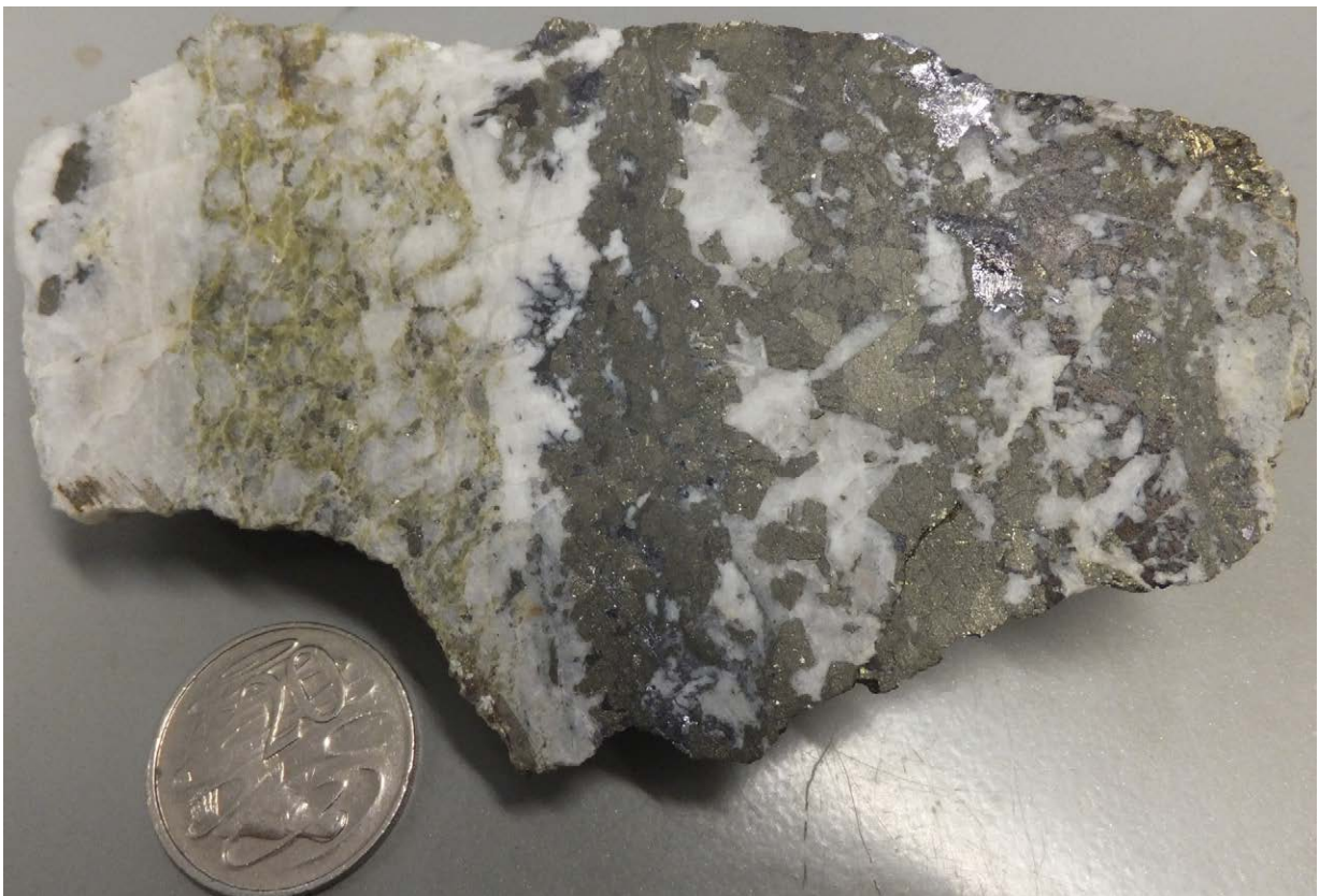
Photograph 108: Auriferous pyrite-chalcopyrite-galena-sphalerite quartz vein mineralisation from Charters Towers (sample from GSQ's historical collection, image courtesy Paul Blake, GSQ).
