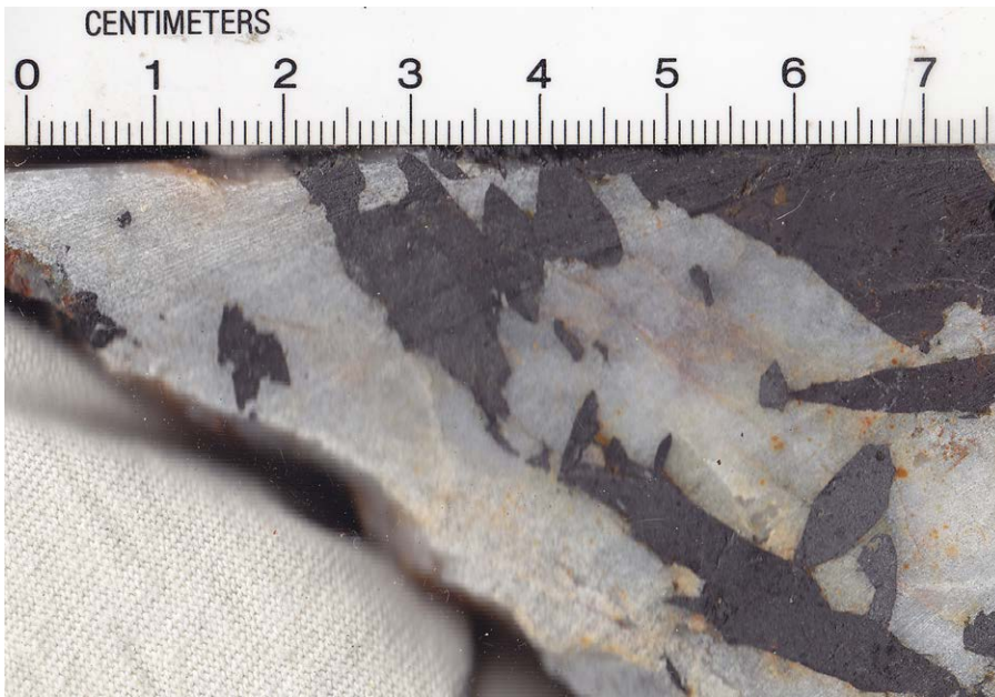
Photograph 177: Tungsten quartz vein mineralisation from Mount Carbine wolfram mine.
