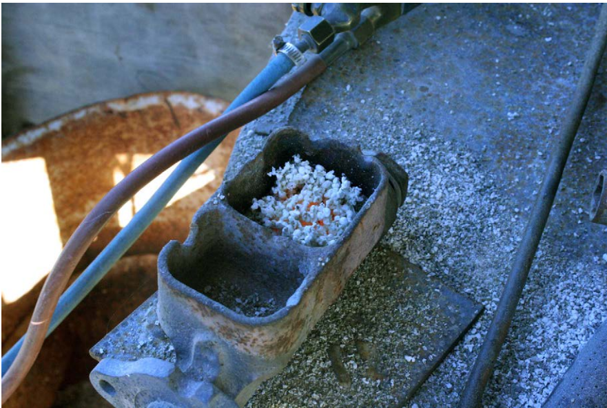
Photograph 271: Making crushed perlite expand under red heat (demonstration only).
