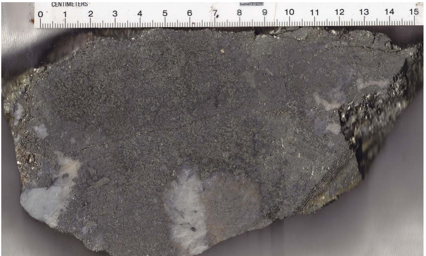
Photograph 52: Sulphide (chalcopyrite) mineralisation from Great Australia mine.
