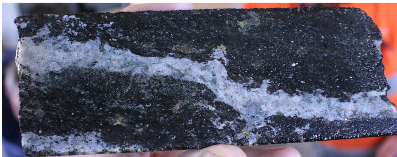
Photograph 192: Drill core from Elaine Dorothy in quartz veined and foliated pyroxenite with an extremely high radioactive response (uranium mineralisation present).
