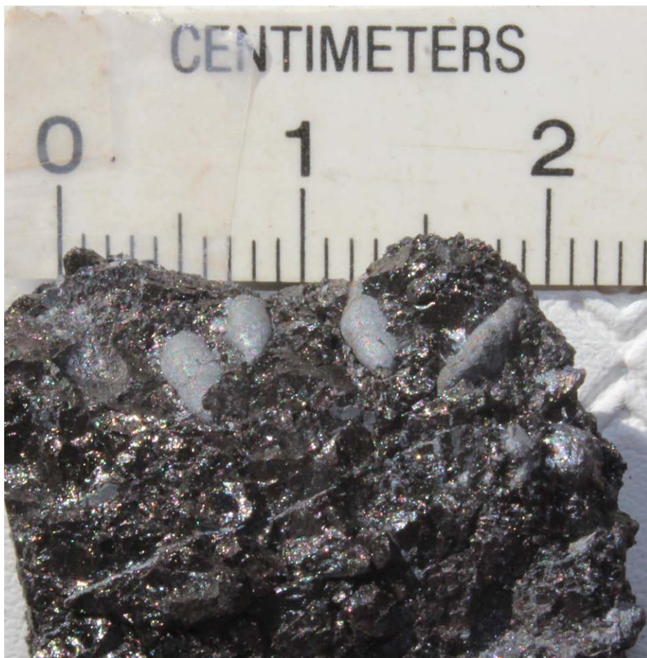
Photograph 102: Wolframite with blebs (teardrop-shaped) native bismuth from Wolfram Camp mine open cut.
