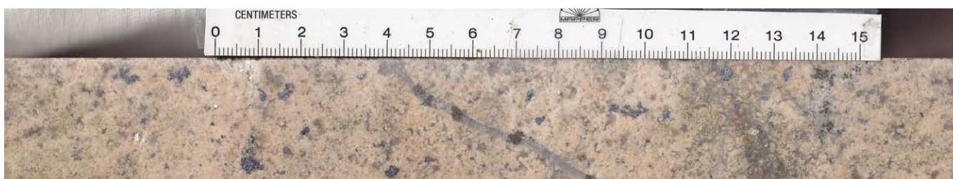
Photograph 65: “Miesels” porphyry with molybdenum rosettes and chalcopyrite veinlets within the Wingfield Granodiorite of the Rawbelle Batholith, Gordons prospect, Whitewash Project.
