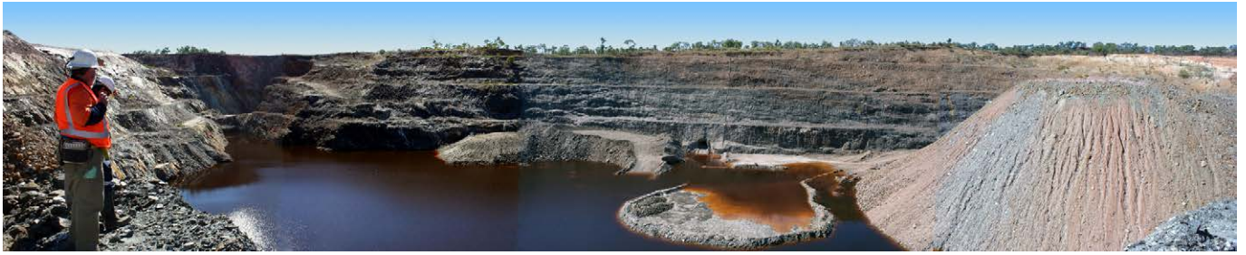
Photograph 58: Panorama view of the Surveyor open cut with underground portal and waste dump refill on right of view.
