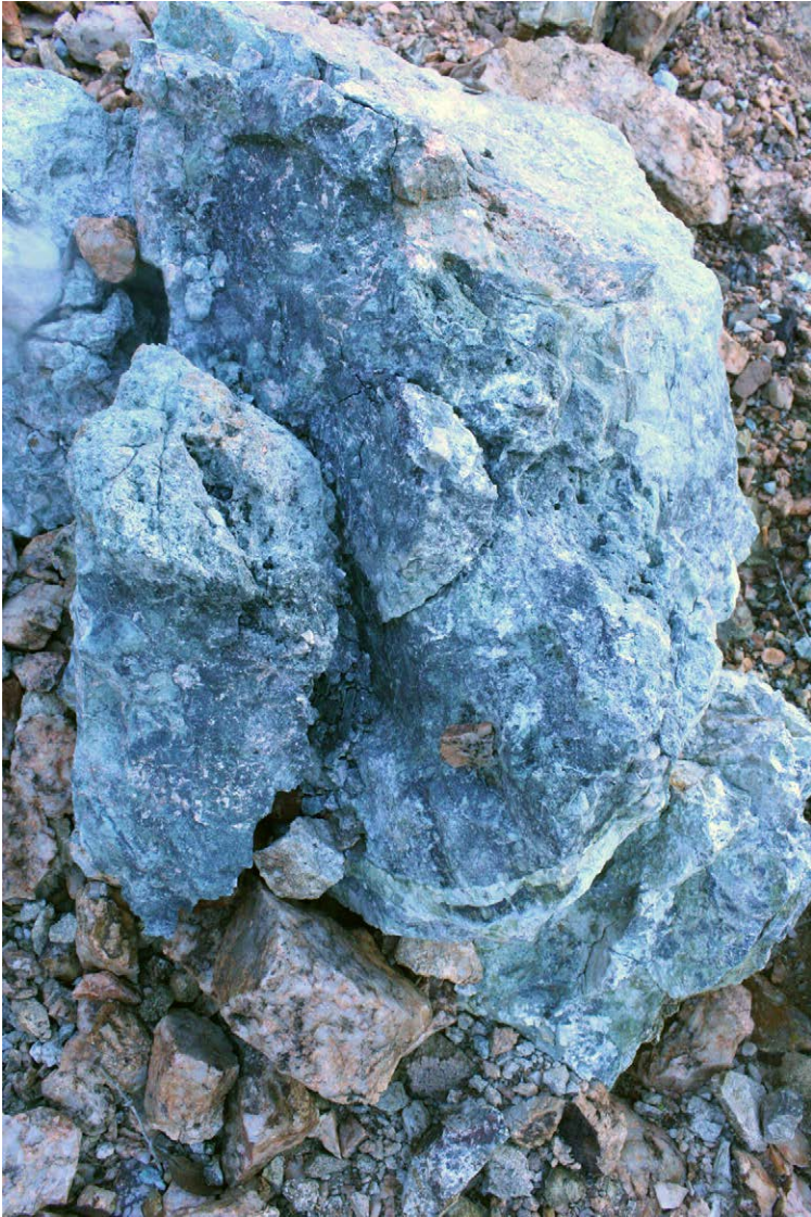
Photograph 144: Oxidised sulphide mineralisation (arsenopyrite with gold) from an ore lens in the Lorena Gold mine open cut.
