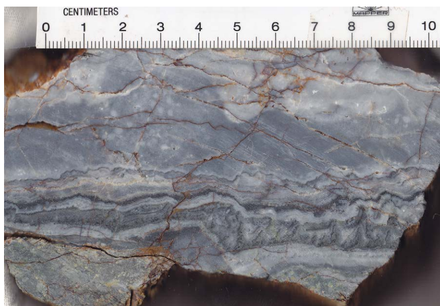
Photograph 141: Mineralised quartz veins from Glen Eva.
