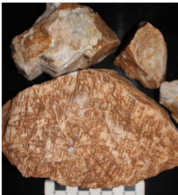
Photograph 155: (Left) Medium gained pink lepidolite from Pegmatite 1 at Buchanan's Creek. (Right) Quartz feldspar lepidolite pegmatite from Pegmatite 3 at Buchanan's Creek.
