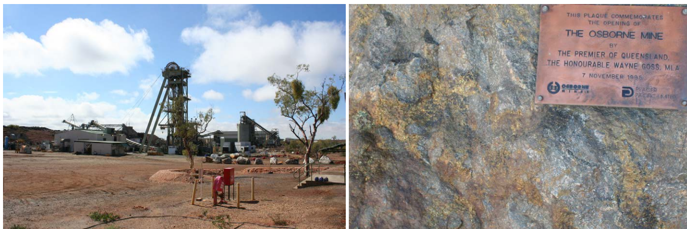
Photograph 36: (left) Osborne plant with headframe and conveyor belts; (right) Osborne copper mineralisation.
