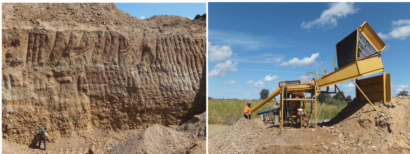
Photograph 205: (left) One of several deep open cuts down to the 'wash' levels of the alluvium at the Australia Mine; (right) mobile alluvial screening plant at Australia Mine.
