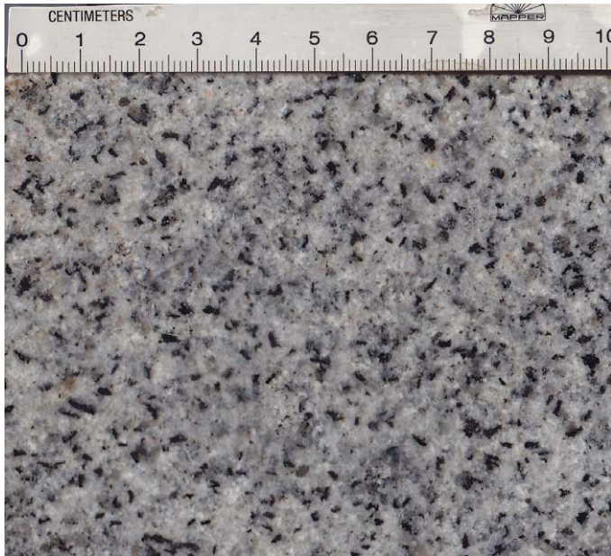
Photograph 238: Fine to medium-grained biotite granite from Greymare quarry near Warwick.
