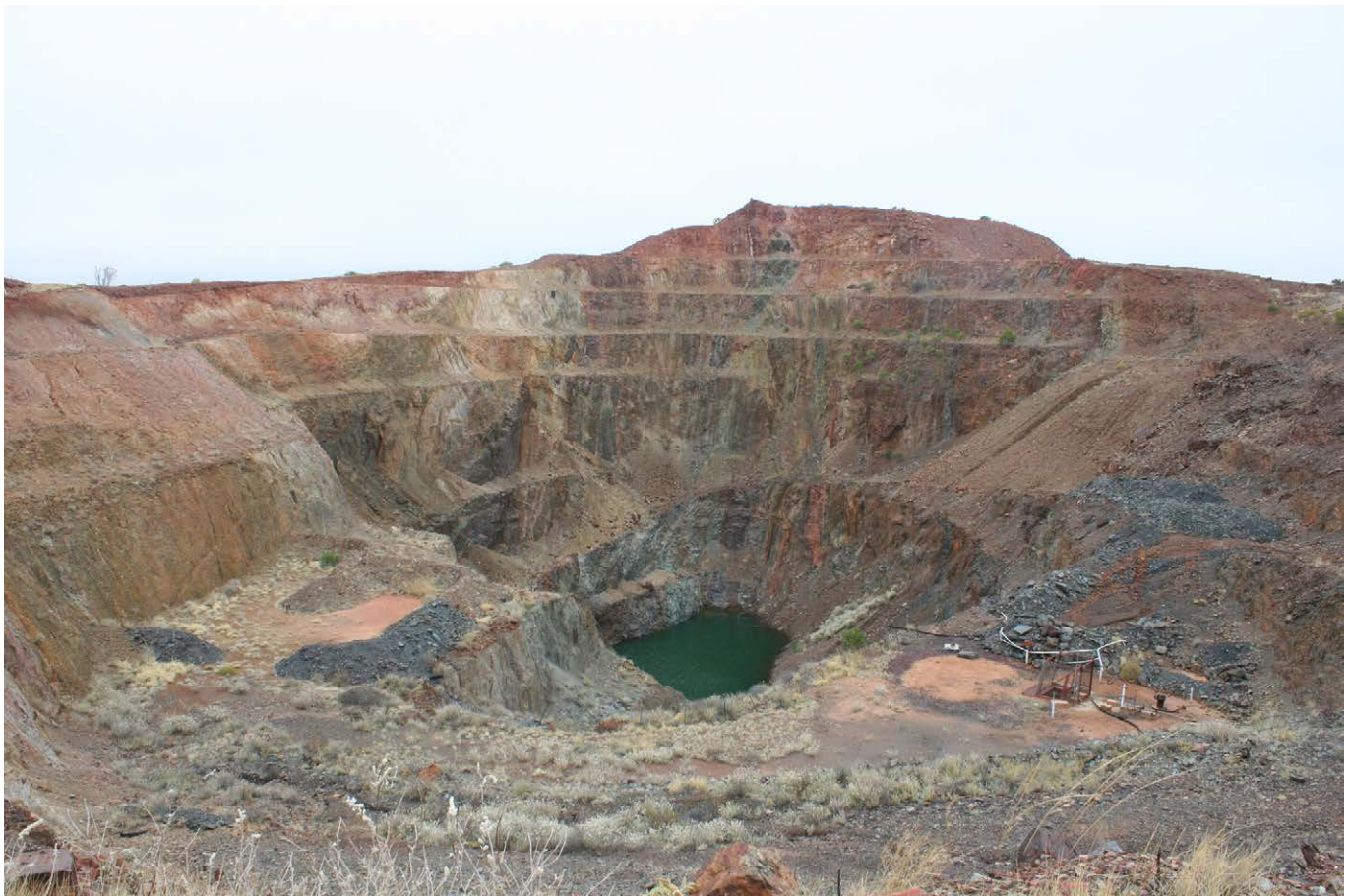
Photograph 38: Starra 257 open cut showing steeply dipping massive hematite bands within the Starra Line stratigraphy. Laminated hematite quartz ironstone and fine hematite mica schist are the main rock types.
